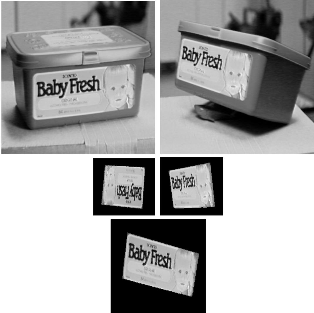
Figure 3: Results by affine invariant method on the Baby-Wipe pictures.
