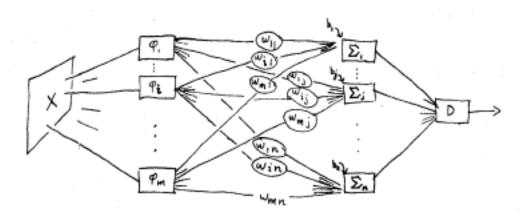
where D is a device that simpl**g** decides which of its inputs is the largest. Each  $\phi$ -device emits a standard-sized pulse (if  $\phi(X) = 1$ ) when X is presented. The pulses are multiplied by the w<sub>ij</sub> quantities as indicated, and summed at the  $\Sigma$ -boxes.
