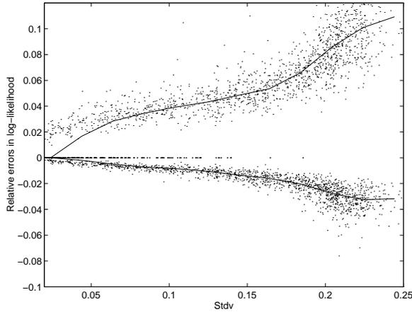
Figure 2: Accuracy of the bounds for noisy-OR networks. The solid lines are the median relative errors in log-likelihood as a function of  $\sigma_{std}$ . The upper and lower curves correspond to the upper and lower bounds respectively.
