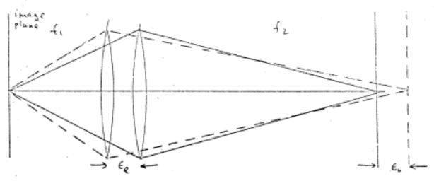
$$d = f_1 + f_2 = \frac{f_1^2}{f_1 - f} \; ; \; : \; f_1 = \frac{d - \int d^2 t df}{2} = f \left[ \left( \frac{d - 2f}{2f} \right)^2 + 1 - \left[ \left( \frac{d - 2f}{2f} \right)^2 - 1 \right] \right]$$
