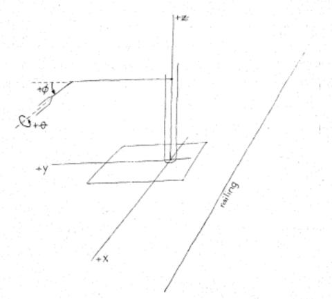
It should be pointed out that because of the geometry of the arm, a change in X,Y will cause a change of \$\phi\$ since an attempt is made to keep the proper orientation of the hand. If a user specifies a position outside the limit specified for the axis, the position will peg at the relevant limit. In addition, a null motion is represented by a word of all ones where the new position value is normally found. The current routine has two additional features:
