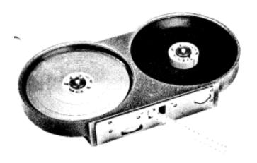
Put the roll of film on the spindle, using the core adapters if necessary. Be sure to draw the end of film downward to prevent slack from being caught under the roll.
