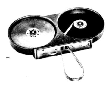
7. Push inward on the take-up light lock lever and insert the end of the film into the slot in the take-up side of the chamber until the end of the film can be put in the slot in the plastic core. Put about 2 loops of film on the core. Replace the take-up compartment cover. Draw out about a 1 1/2-foot loop of film from the supply reel.
