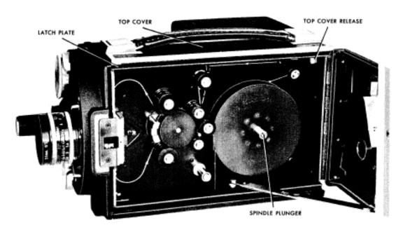
Take the film loop that extends from the bottom of the film chamber and put it through the rectangular opening in the top of the camera. Slide the front edge of the chamber under the cover retaining latch plate. Latch the top cover release to secure the chamber on the camera top.
