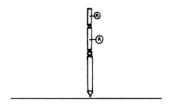
Project: Design a program to balance this device. The letter A marks two places at which accelerometers are attached.
