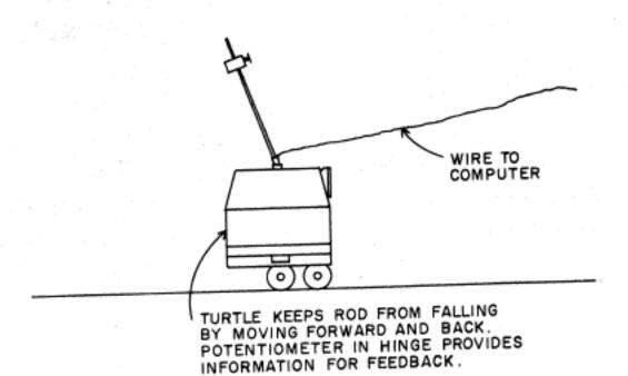
What kind of program can make the turtle balance the rod? It is remarkable (but very typical of this kind of work) that an incredibly simply procedure will work under restricted but realistic conditions. This procedure (believe it or not!) is simply:
