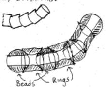
Also, one can make the friction very low, to get an extremely compliant wrist, by relaxing the tendons that act counter to the desired direction of motion. This principle is used in several commercial holding and positioning devices.
