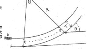
If the rod has thickness T and length L, and one side is D shorter than the other, the rod will bend in a curve for which
