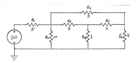
At first glance, this is a 3 node equation network with no possible series-parallel reductions. We want to generalize Guillemin's trick to solve this network (with fewer than 3 equations).
