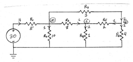
We have solved the network with only two unknowns. As we approach a full graph network, this method degrades smoothly to be the node method, but usually it uses far fewer unknowns.
