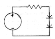
In this circuit, the only physically consistent states for the diodes to be in is both conducting. If, however, we assume both are cutoff, EL will not discover the contradiction because that would entail the propagation of inequalities. De Kleer <de Kleer 1976> solves this problem by propagating ranges, but he cannot handle symbolic expressions at all. We are looking for a way of handling inequality constraints in a more declarative manner than by monitor demons.
