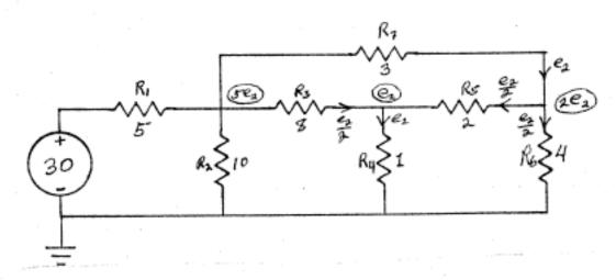
Continuing, we deduce that the current through  $R_2$  must be  $5e_2/10=e_2/2$ . By KCL, the current through  $R_1$  must be  $2e_2$ . Ohm's law now gives as the voltage at the left of  $R_1$  as  $15e_2$ . But this voltage is set by the voltage source, so  $15e_2=30$ . We conclude that  $e_2=2$ :
