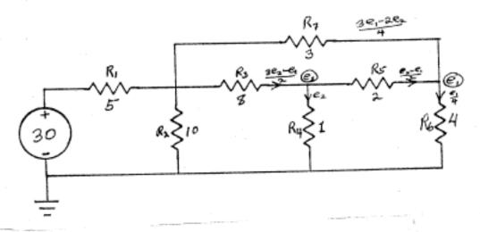
At this point we can deduce that the voltage on the leftmost terminal of  $R_7$  is  $e_1 \cdot (3/4)(3e_1 - 2e_2)$  or  $(13e_1 - 6e_2)/4$ . We can also deduce that the voltage on the leftmost terminal of  $R_3$  is  $e_2 \cdot 8((3e_2 - e_1)/2) = 13e_2 \cdot 4e_1$ . Since these terminals are connected together we have two expressions for the same node voltage. Setting them equal and simplifying, we get  $e_1 \cdot 2e_2$ . The result of this simplification is:
