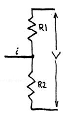
Supposing V and i are known, the current through R1 (and hence through R2) can be propagated by simultaneously assuming the correctness of both R1 and R2.
