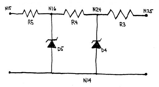
Assume that the fault in this circuit is that D4 has a breakdown voltage too low. This causes the voltage across D5 to be less than its breakdown. Assume the following measurements are made:
