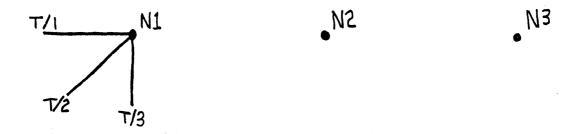
The circuit consists of components such as resistors and capacitors etc., terminals of these components are connected to nodes at which two or more terminals are joined. In the above diagram T/1, T/2 and T/3 are terminals and NI, N2 and N3 are nodes. Currents are normally associated with terminals, and voltages with nodes.
