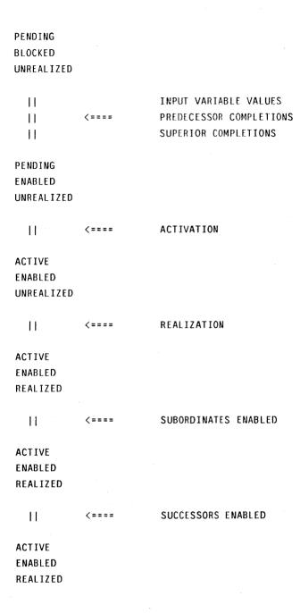
Figure 2: Intention progress state transitions. A pending intention is blocked until it has input variables, and its predecessors and superiors are complete. The intention then becomes ACTIVE, and when realized by a plan, is followed by its subordinates and successors.
