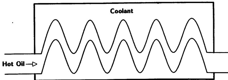
Figure 4: Hot Oil Flows Through Heat Exchanger
