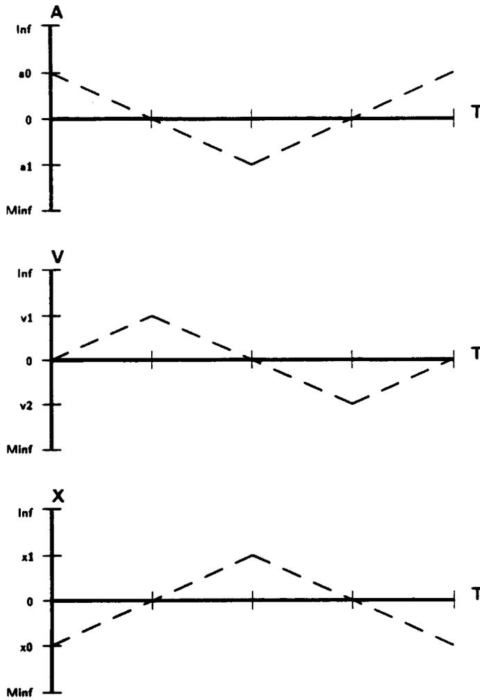
Figure 2: QSIM Behavior for Stable Spring Oscillation
