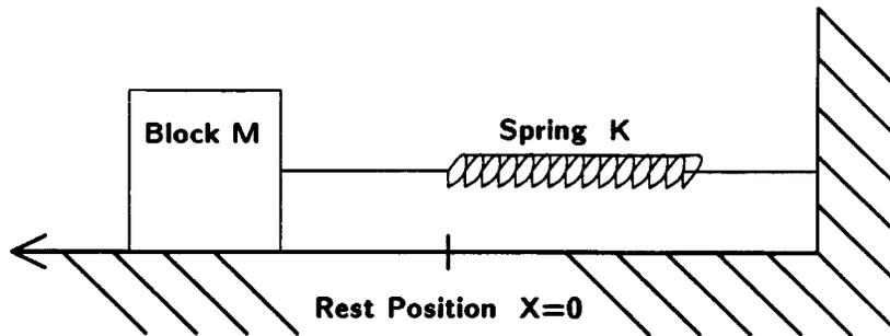
Figure 1: Ideal Spring Attached to Block on Frictionless Table
