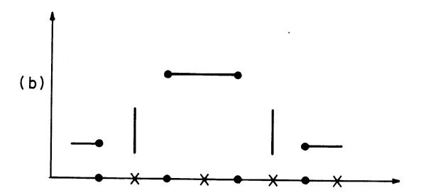
Figure 1 The line processors. In (a) there are no line processes and the interpolation process assumes that the points lie on a single surface. In (b) the line processes switch on and break the surface where the gradient is large.
