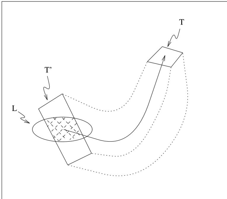
Figure 5.17: Computing whether a single-segment path meets a tolerance. The solid arrow is the path segment  $\vec{S}$ ;  $T$  is the tolerance region at its endpoint.  $T'$  is the same region, integrated backwards to the starting point  $\vec{S}_{init}$ .  $L$  is the domain of the junction controller at  $\vec{S}_{init}$ . If  $\vec{S}_{final}$  lies in  $T$  and  $\vec{S}_{init}$  lies in the intersection of  $T'$  and  $L$ , the segment passes the check.
