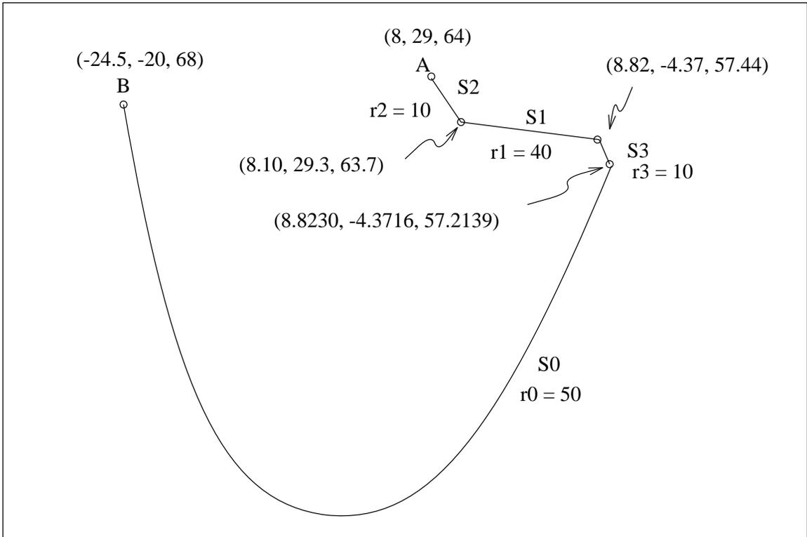
Figure 7.13: Schematized segmented path between **A** and **B**
