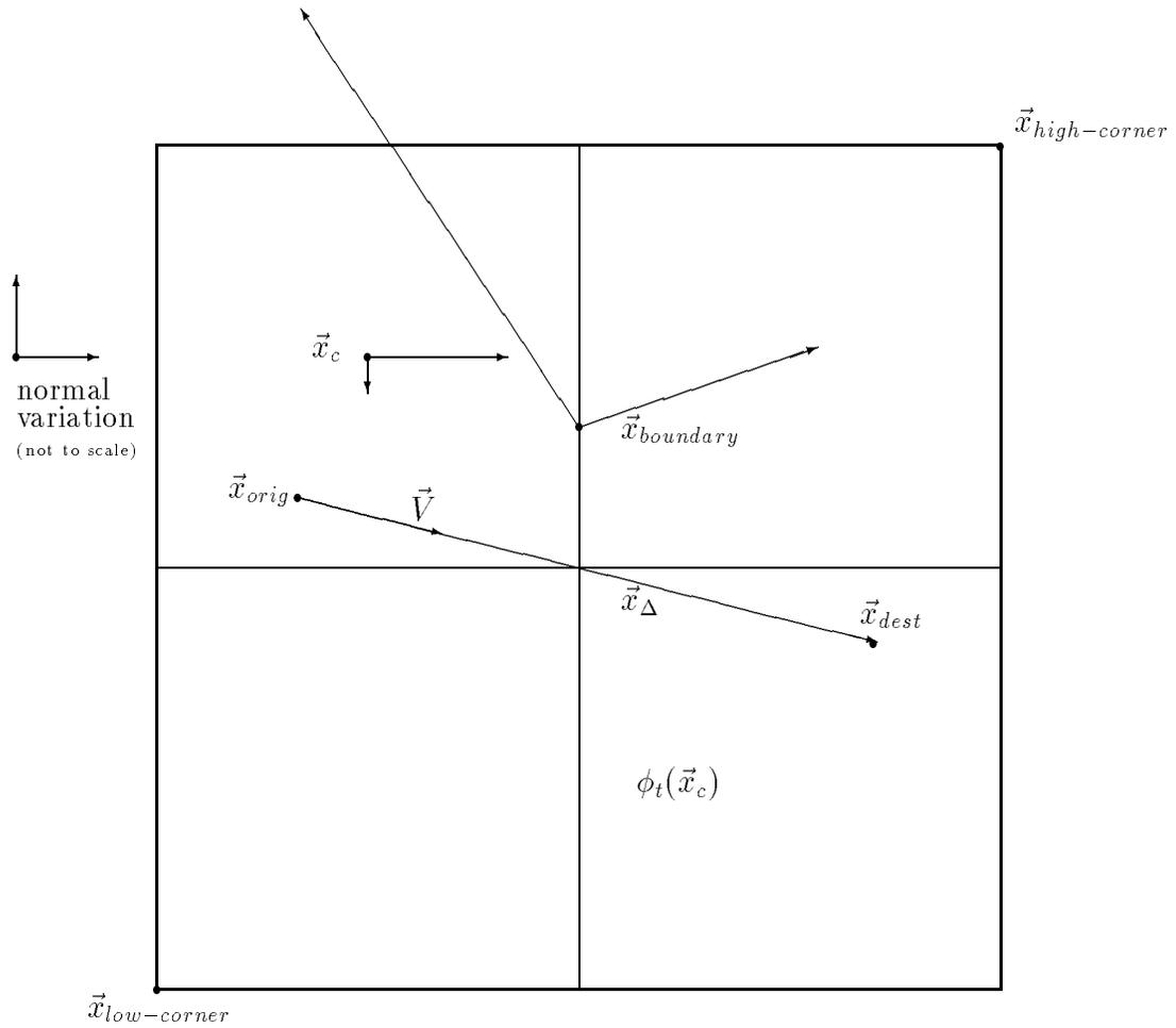
Figure 5.15: Refining the grid: if the variation  $\vec{V}$ , integrated forwards from the centerpoint  $\vec{x}_c$  of the origin cell to its boundary, grows to be larger than the cell itself, the cell size is reduced. The initial variation is a scaled version of the difference vector  $\vec{x}_\Delta$  between the origin and the destination
