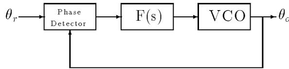
Figure 7.29: Phase-locked loop block diagram
