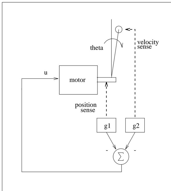
Figure 3.2: Linear feedback control of an inverted pendulum: A traditional linear controller stabilizes a system by wrapping it in a feedback loop and finding values for the feedback gains  $g_1$  and  $g_2$  that place the poles of the closed-loop system in the left-half plane.
