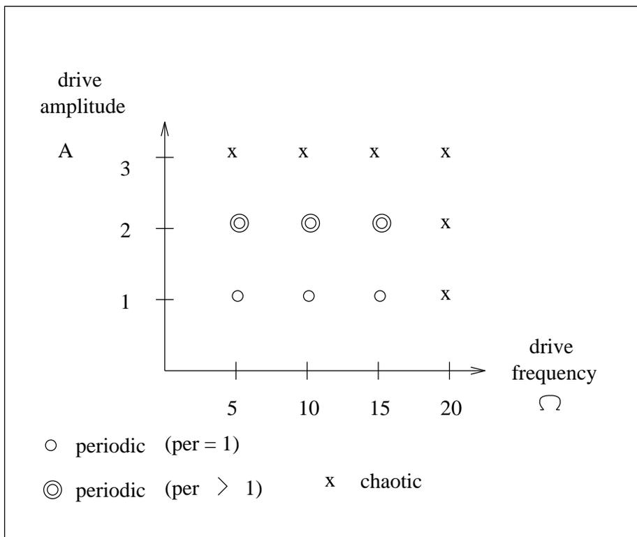
Figure 7.21: Parameter-space plot for the driven-vertex pendulum
