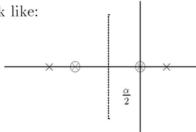
The  $\otimes$  points are  $\Omega = 0$  poles and the  $\times$  poles reflect some nonzero natural frequency. The latter — the true physical situation — is clearly unstable. The  $\alpha < 0$  plot is the mirror image of this one about the y-axis.
