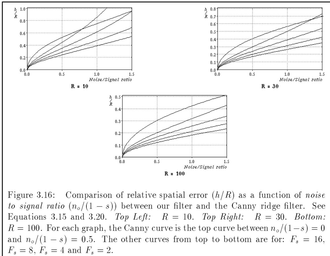
Figure 3.16: Comparison of relative spatial error ( $h/R$ ) as a function of *noise to signal ratio* ( $n_o/(1-s)$ ) between our filter and the Canny ridge filter. See Equations 3.15 and 3.20. *Top Left:*  $R = 10$ . *Top Right:*  $R = 30$ . *Bottom:*  $R = 100$ . For each graph, the Canny curve is the top curve between  $n_o/(1-s) = 0$  and  $n_o/(1-s) = 0.5$ . The other curves from top to bottom are for:  $F_s = 16$ ,  $F_s = 8$ ,  $F_s = 4$  and  $F_s = 2$ .
