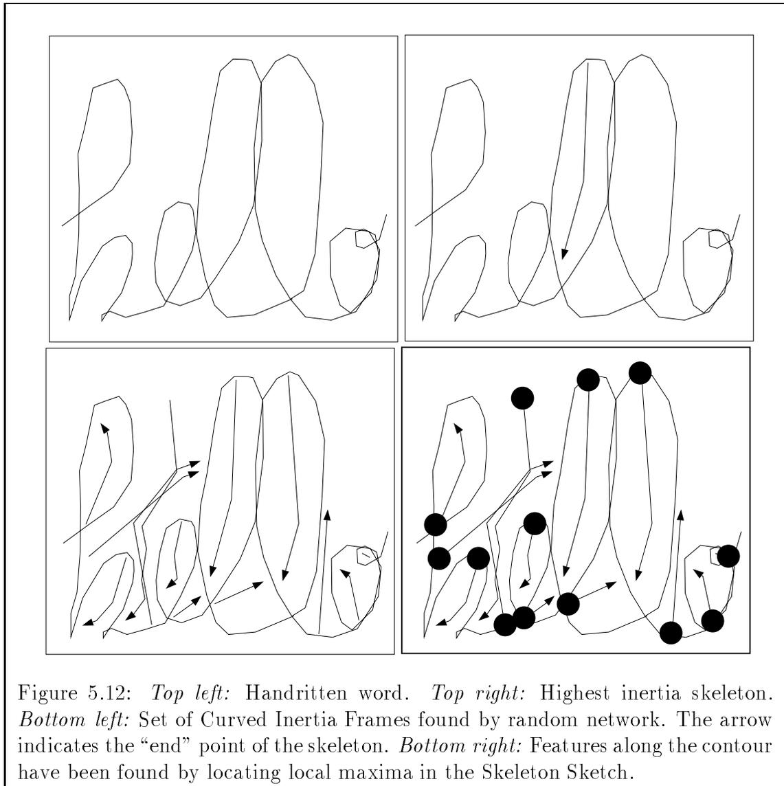
Figure 5.12: *Top left:* Handwritten word. *Top right:* Highest inertia skeleton. *Bottom left:* Set of Curved Inertia Frames found by random network. The arrow indicates the "end" point of the skeleton. *Bottom right:* Features along the contour have been found by locating local maxima in the Skeleton Sketch.
