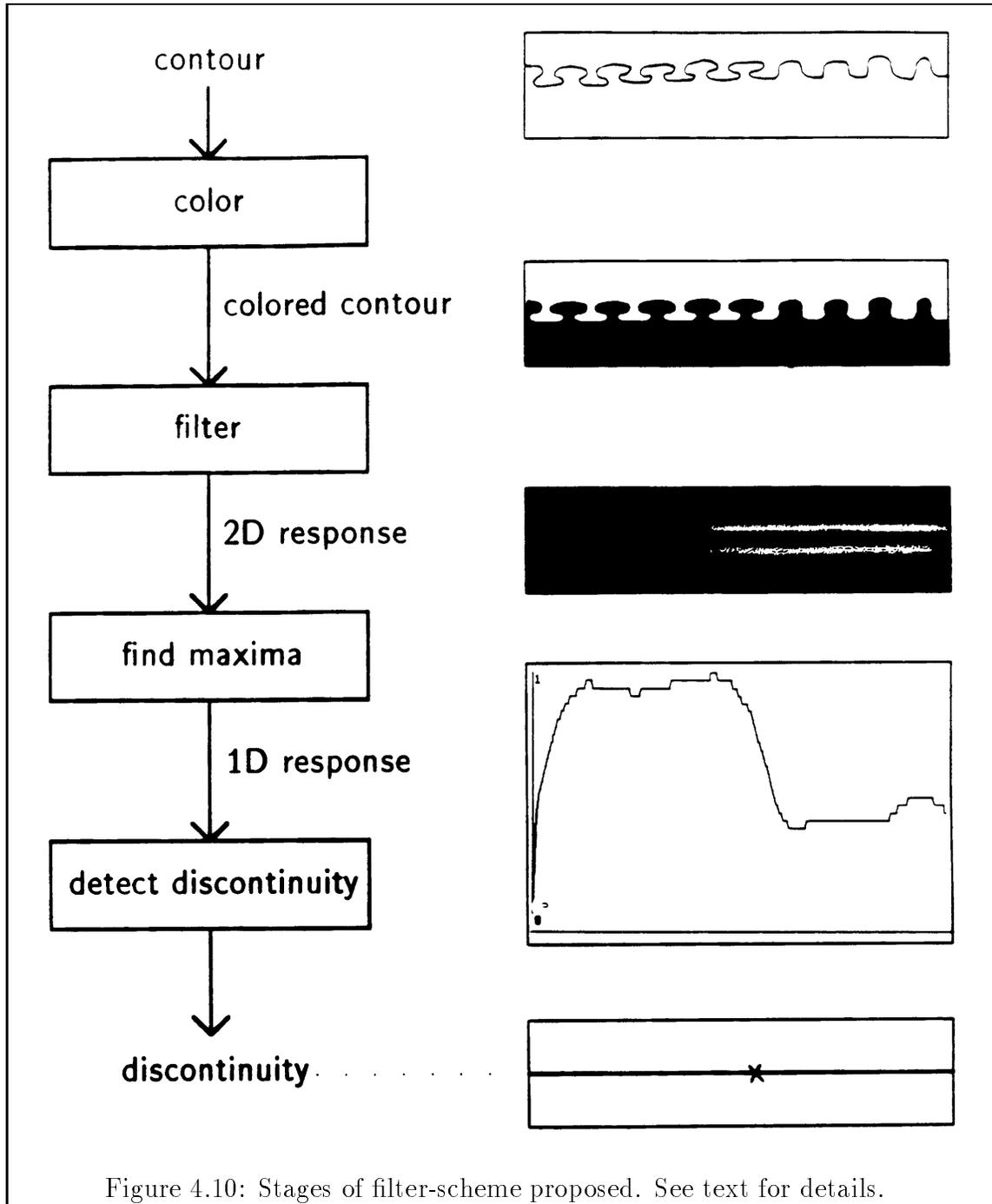
Figure 4.10: Stages of filter-scheme proposed. See text for details.
