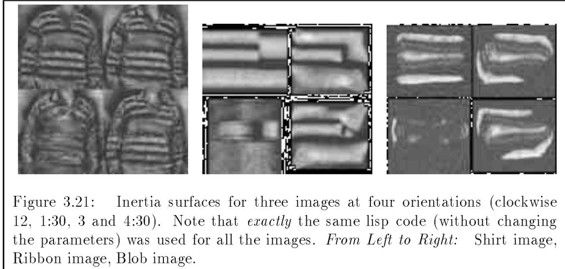
Figure 3.21: Inertia surfaces for three images at four orientations (clockwise 12, 1:30, 3 and 4:30). Note that *exactly* the same lisp code (without changing the parameters) was used for all the images. *From Left to Right:* Shirt image, Ribbon image, Blob image.
