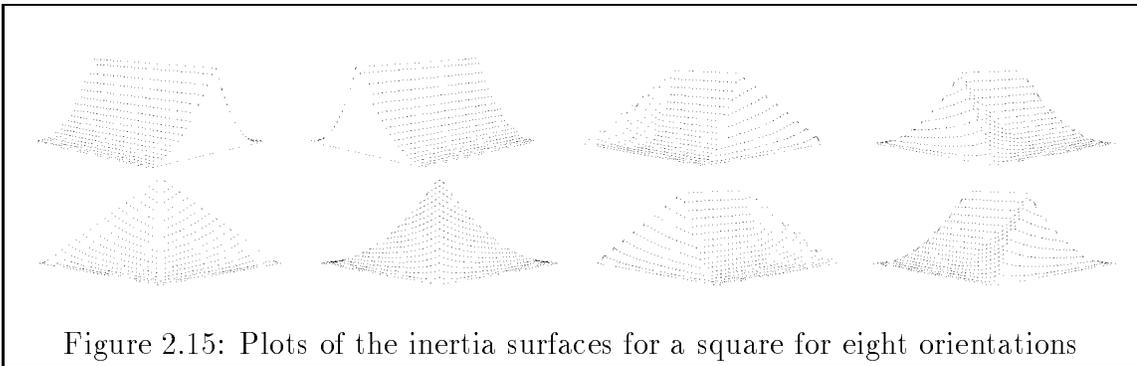
Figure 2.15: Plots of the inertia surfaces for a square for eight orientations
