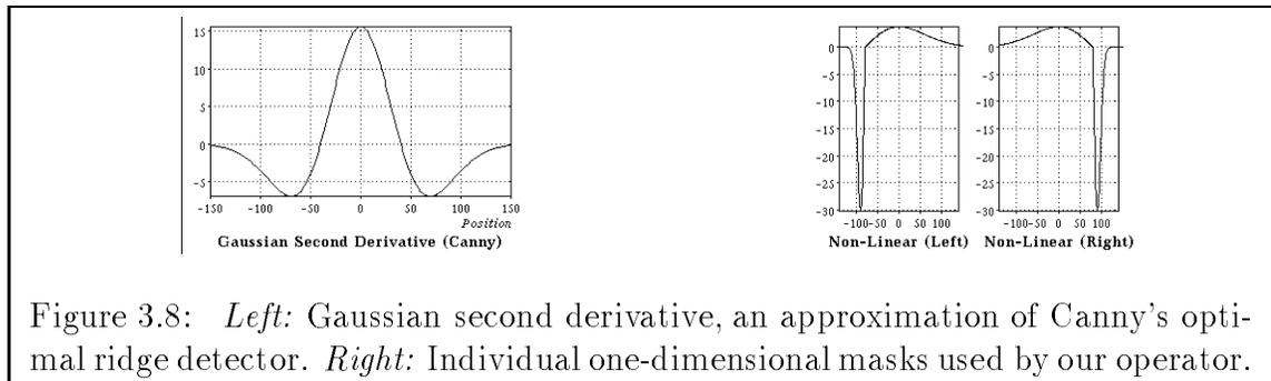
Figure 3.8: *Left*: Gaussian second derivative, an approximation of Canny's optimal ridge detector. *Right*: Individual one-dimensional masks used by our operator.
