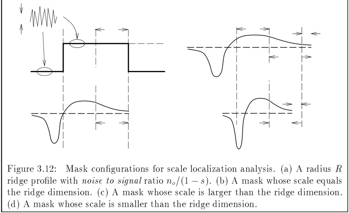
Figure 3.12: Mask configurations for scale localization analysis. (a) A radius  $R$  ridge profile with *noise to signal* ratio  $n_o/(1-s)$ . (b) A mask whose scale equals the ridge dimension. (c) A mask whose scale is larger than the ridge dimension. (d) A mask whose scale is smaller than the ridge dimension.
