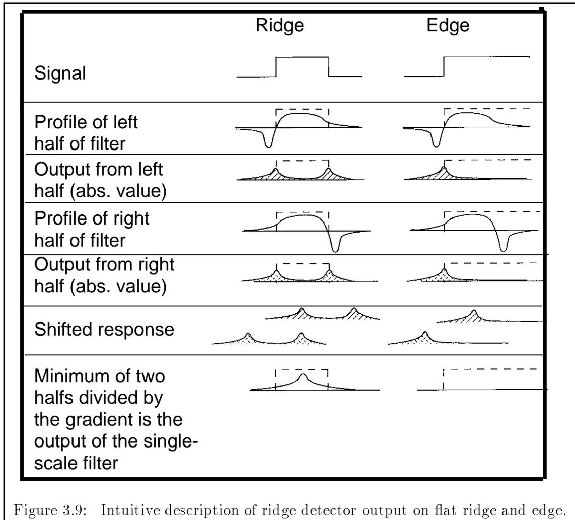
Figure 3.9: Intuitive description of ridge detector output on flat ridge and edge.
