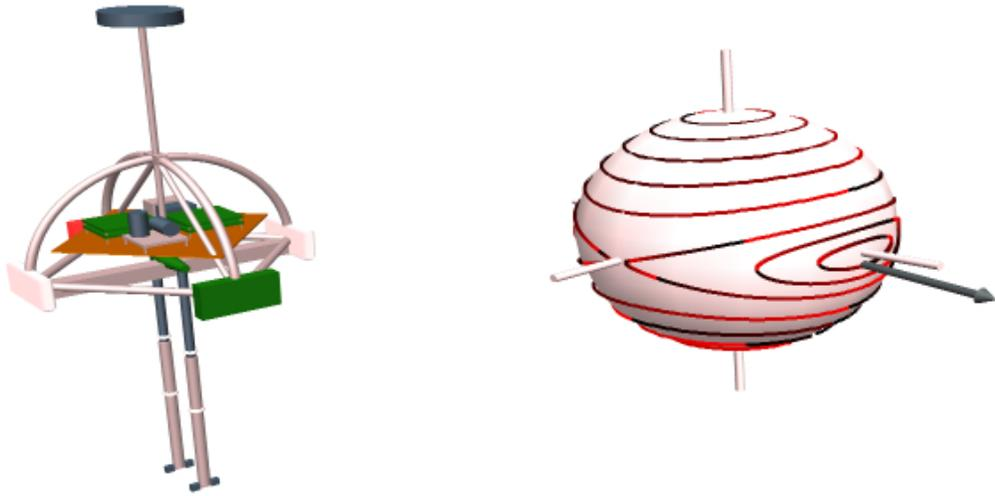
Figure 6-6: Spherical coordinate map of the tilt and twist Euler angle trajectories for the 3D Biped with  $4\text{ kg}$  of weight added at a distance of  $0.8\text{ m}$  above the hip.
