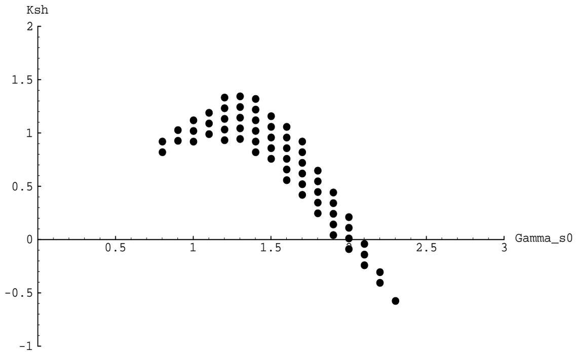
Figure 4-9: Each darkened point in this plot corresponds to a specific choice of  $K_{sh}$  and the nominal symmetric arm angle ( $\Gamma_{s0}$ ) that stabilize the full five d.o.f. linear system,  $b_{sh}/\dot{\Phi} = 0$ .
