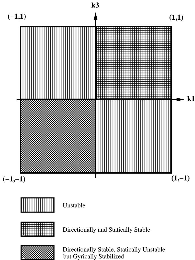
Figure 2-3: Stability diagram for the simple spin solutions of a rigid body. Rigid body rotational stability depends only upon the two non-dimensional inertia ratios  $k_1$  and  $k_3$ . We assume the body is rotating about the principal axis corresponding to  $I_2$  for this diagram.
