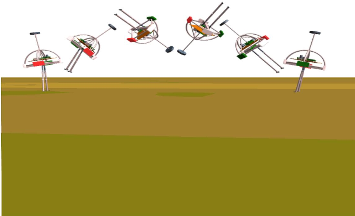
Figure 6-7: Sequence of images of the simulated 3D Biped somersault with twist.
