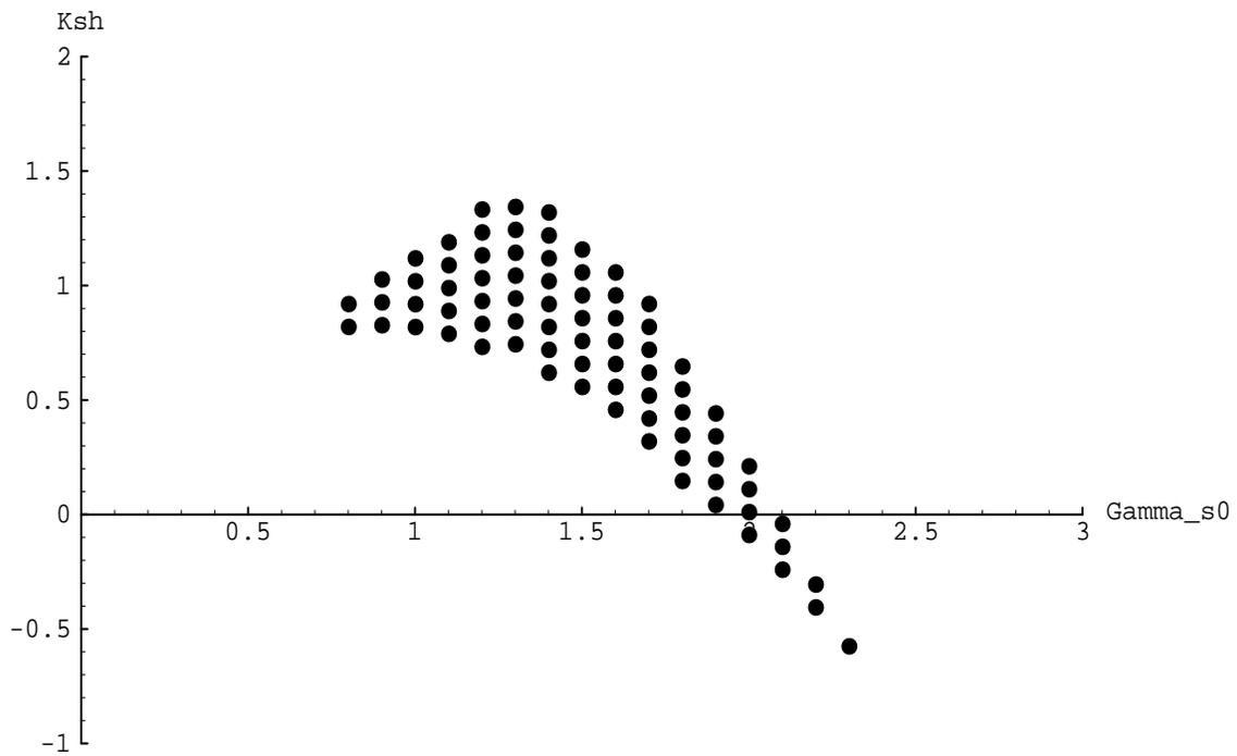
Figure 4-10: Each darkened point in this plot corresponds to a specific choice of  $K_{sh}$  and the nominal symmetric arm angle ( $\Gamma_{s0}$ ) that stabilize the three d.o.f. linear system of tilt, twist, and asymmetric arm movement,  $b_{sh}/\dot{\Phi} = 0$ .
