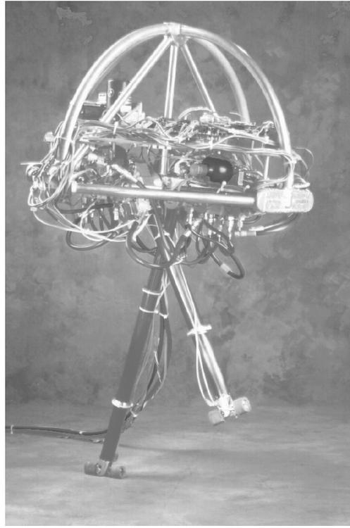
Figure 1-2: Photograph of the 3D Biped Robot.
