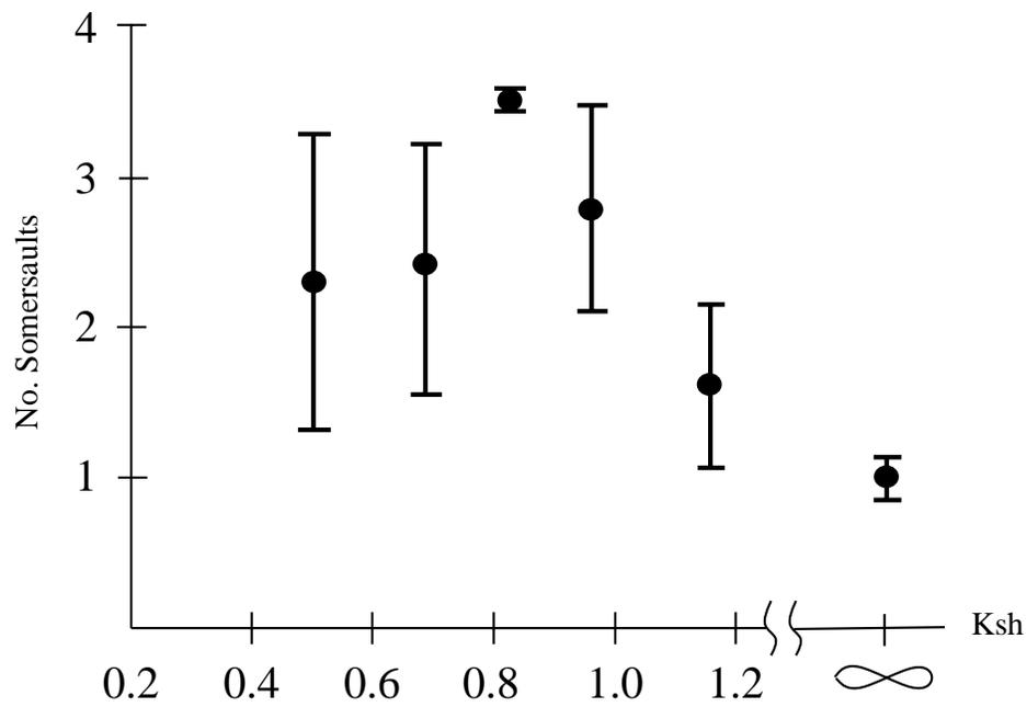
Figure 5-7: Plot of the average number of stable somersaults performed during twenty launches of the doll as a function of the shoulder spring constant,  $K_{sh}$ . The standard deviation is indicated by error bars. The data for the rigidly fixed arms is indicated by the infinite value of  $K_{sh}$ . The nominal arm angle was approximately 1.6 radians. The best value of  $K_{sh} = 0.82$  falls within the range of stability predicted by theory as indicated in Figure 5-5.
