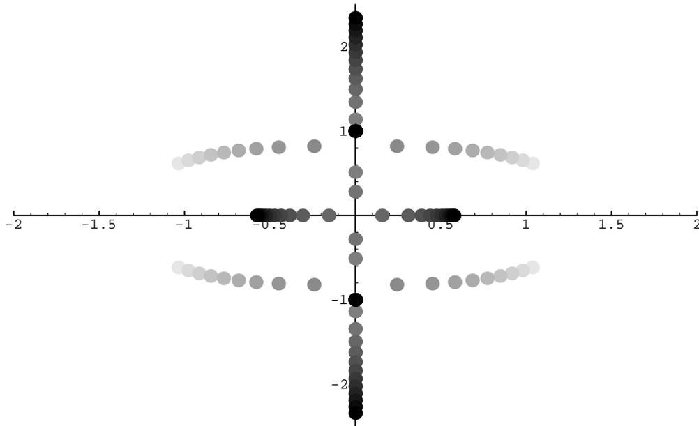
Figure 4-6: Root locus plot for the 3-by-3 subsystem of tilt, twist, and asymmetric arm movement.  $b_{sh}/\dot{\Phi} = 0.0$  and the nominal symmetric arm angle,  $\Gamma_{s0}$ , is 1.3 rad. Light dots indicate root locations for  $K_{sh} \approx -2.0$ . Dots get progressively darker as  $K_{sh}$  increases to 4.0.
