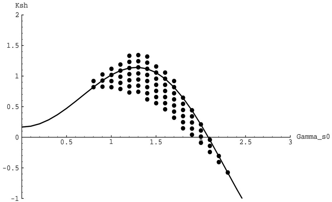
Figure 4-17: Plot of the stabilizing  $K_{sh}$  for a the 3-by-3 subsystem of the human model. The solid curve shows the value of  $K_{sh}$  that will exactly cancel the spring term due to centrifugal forces on the arm.
