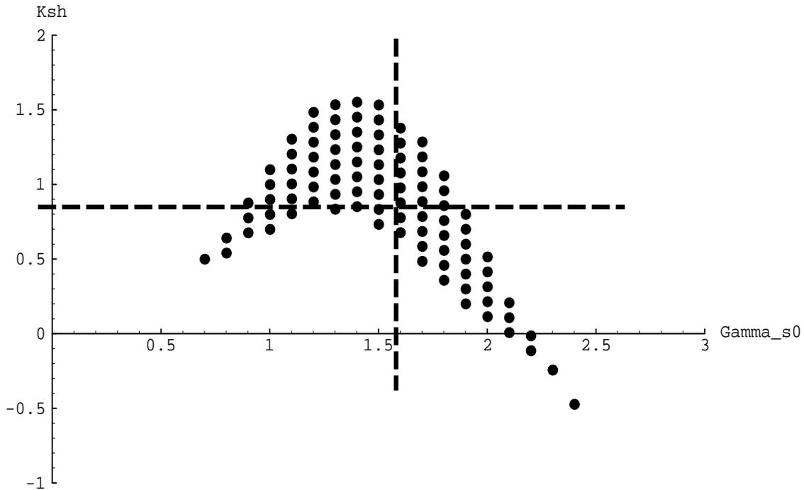
Figure 5-5: The points in this plot indicate the values of  $K_{sh}$  that theoretically will stabilize layout somersaults in the doll. The cross-hairs indicate the spring constant that best stabilized the doll during experiments.
