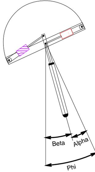
Figure 3-4: In order to maintain balance at landing the leg inclination angle,  $\beta$ , must be near the desired value.  $\beta$  is the angle the leg makes with the local vertical. It is a function of the the hip angle,  $\alpha$  and the body attitude,  $\Phi$ .
