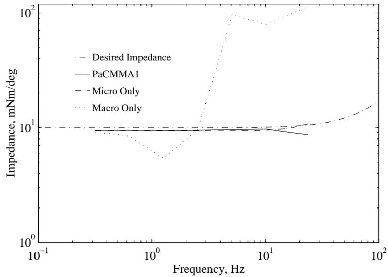
Figure 7-23: **Programmed Impedance.**  $Z(s) = 10 + 0.02s$  (Small Displacement)
