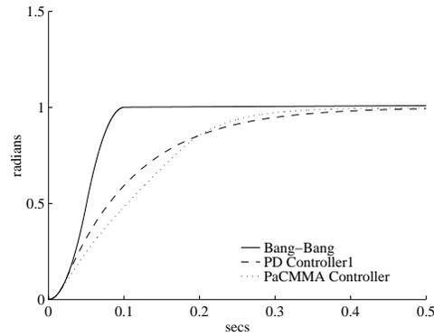
Figure 5-10: **Simulated Position Step Response.**  $x_{des} = 1.0\text{rad}$
