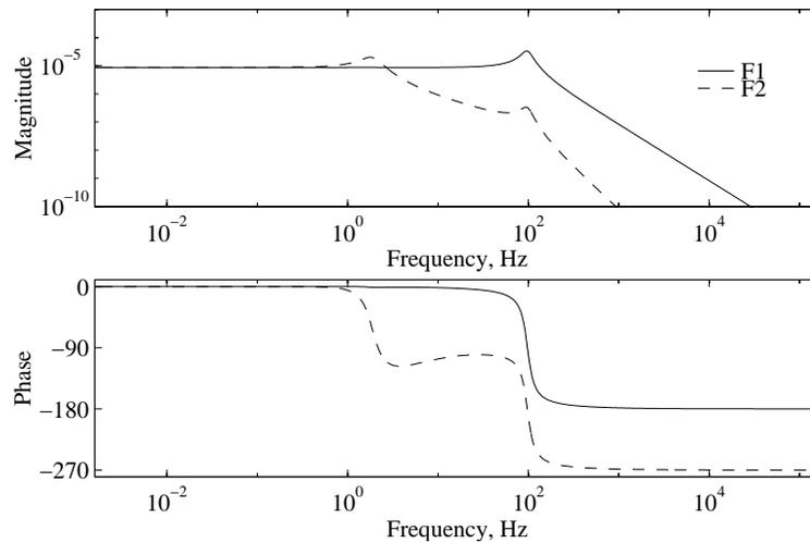
Figure 4-4: **Frequency Response with a stiff environment.**  $\frac{X_1(s)}{F_1(s)}, \frac{X_1(s)}{F_2(s)}$  where  $X_1$  is the displacement of the endpoint,  $F_1$  is the force command to the micro-actuator and  $F_2$  is the force command to the macro-actuator.
