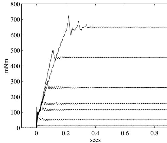
Figure 7-5: **Large Step Response for PaCMMMA1.** The small oscillations in the force which persist after reaching the desired force represent the unmodelled dynamics in the transmission. The steel extension springs are vibrating at 100 Hz due to the sudden change in force. Since this disturbance is greater than the micro-actuator bandwidth, they can not be suppressed.
