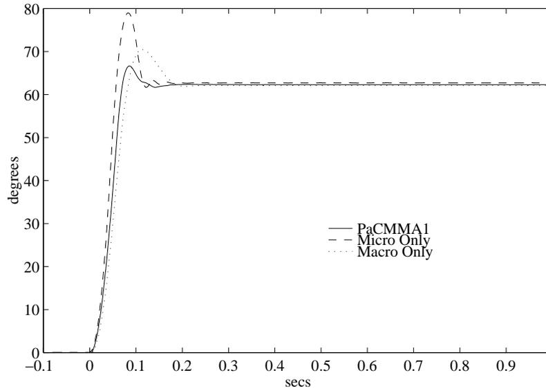
Figure 7-15: **Large Step Response.**  $F_{des} = 62.5$  degrees
