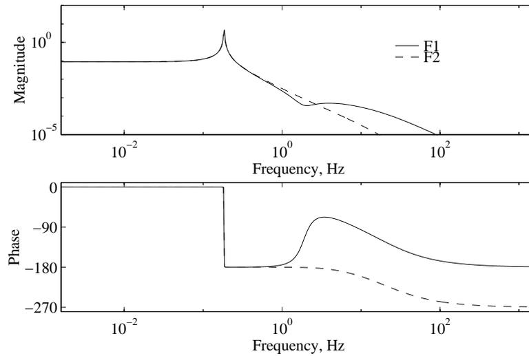
Figure 4-3: **Frequency Response with a soft environment.**  $\frac{X_1(s)}{F_1(s)}, \frac{X_1(s)}{F_2(s)}$  where  $X_1$  is the displacement of the endpoint,  $F_1$  is the force command to the micro-actuator and  $F_2$  is the force command to the macro-actuator.
