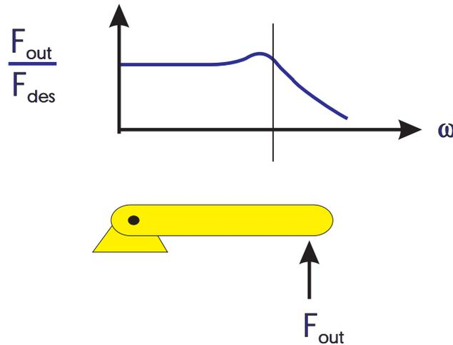
Figure 3-1: **Force Control Response.** Force control response is a frequency response measurement which is obtained with a fixed endpoint. The 3db point may be used to define force bandwidth.
