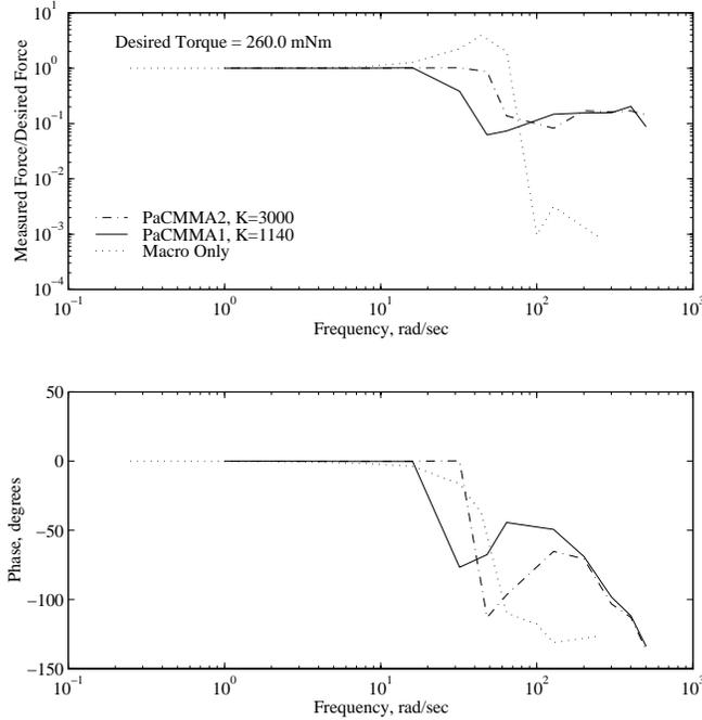
Figure 7-3: **Large Signal Force Control Bandwidth.**  $F_{des} = 0.32$ ,  $F_{2sat} = 2.3F_{1sat}$ . Performance was measured using explicit force control.
