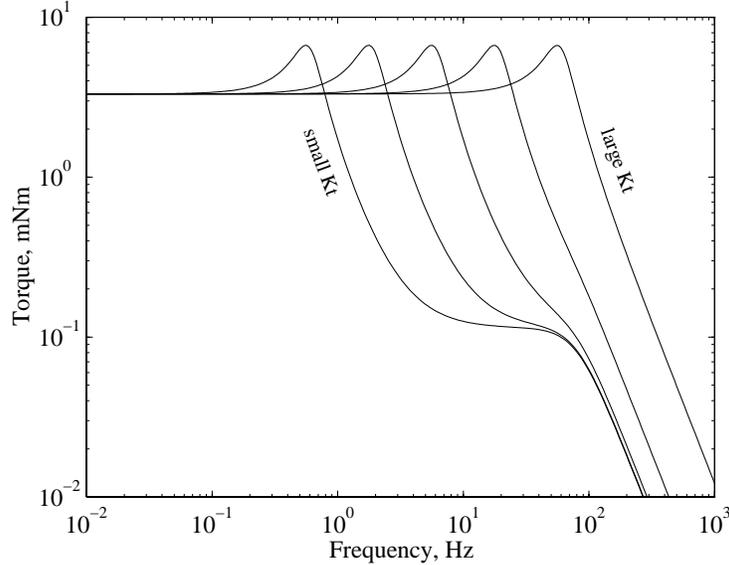
Figure 6-1: **Force Control Bandwidth for Varied Transmission Stiffness.** The force control bandwidth was calculated using equation 4.13 and the simulation parameters can be found in Appendix A. The transmission stiffness,  $K_t$ , was given the following values:  $114, 1.14 \times 10^3, 1.14 \times 10^4, 1.14 \times 10^5, 1.14 \times 10^6$  mNm/rad.
