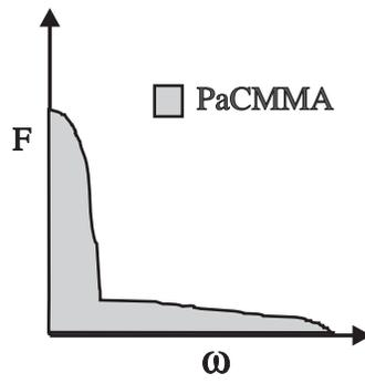
Figure 6-4: Force Control Performance Space for PaCMMA System
