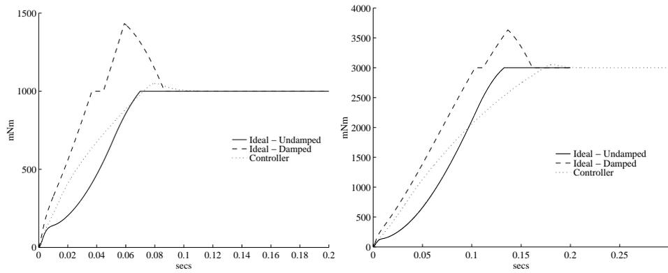
Figure 5-8: **Simulated Force Step Response.**  $F_{des} = 1000$  mNm and  $F_{des} = 3000$  mNm. This figure shows a comparison of three systems: Bang-bang control on an undamped transmission, bang-bang control on a damped system and the PaCMMA force controller. For damped case,  $\zeta = 0.25$
