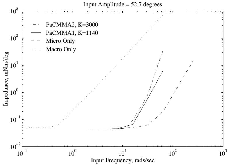
Figure 7-12: **Large Amplitude Impedance Response.** Impedance response data is shown for  $F_{des}^{\vec{r}}=0$ . All systems used explicit force control algorithms.
