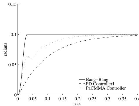
Figure 5-9: **Simulated Position Step Response.**  $x_{des} = 0.1\text{rad}$
