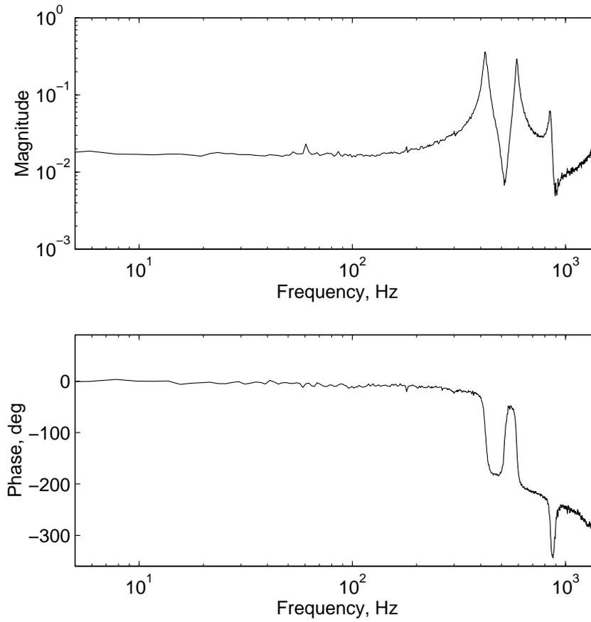
Figure A-1: **Micro Actuator Transfer Function.**  $\frac{F_c(s)}{F_1(s)}$  - Experimentally measured by clamping the output shaft and doing a frequency sweep,  $F_1 = A\sin(\omega t)$
