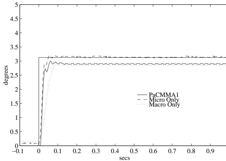
Figure 7-16: **Small Step Response.**  $F_{des} = 3.125$  degrees
