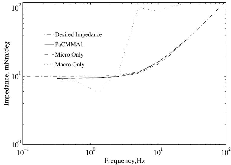
Figure 7-19: **Programmed Impedance.**  $Z(s) = 10 + 0.66s$  (Small Displacement). This shows that the micro-actuator and PaCMMMA can effectively produce the desired impedance. The macro-actuator can not emulate the impedance as accurately.
