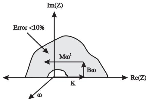
Figure 3-5: **Impedance Performance Space.** The actuator is programmed to create a desired impedance,  $Z(\omega) = Ms^2 + Bs + K$  and the impedance response at each frequency is plotted in the complex plane using  $s = j\omega$ . If the actuator can produce the desired impedance with less than 10% error, then the impedance is contained in the shaded region; the region is bounded by a curve of constant error.
