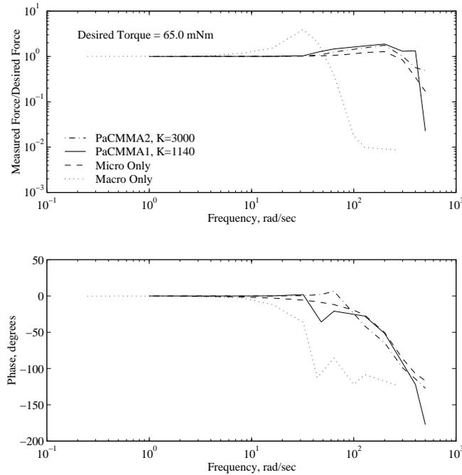
Figure 7-2: **Small Signal Force Control Bandwidth.**  $F_{des} = 0.08$ ,  $F_{2sat} = 0.57F_{1sat}$ . Performance was measured using explicit force control
