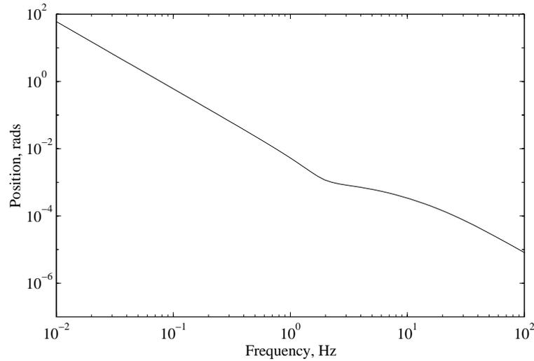
Figure 4-5: **Maximum Position Response.** This figure shows the position response if both actuators are saturated and their forces are summing constructively. It provides an upper bound on the achievable position bandwidth.
