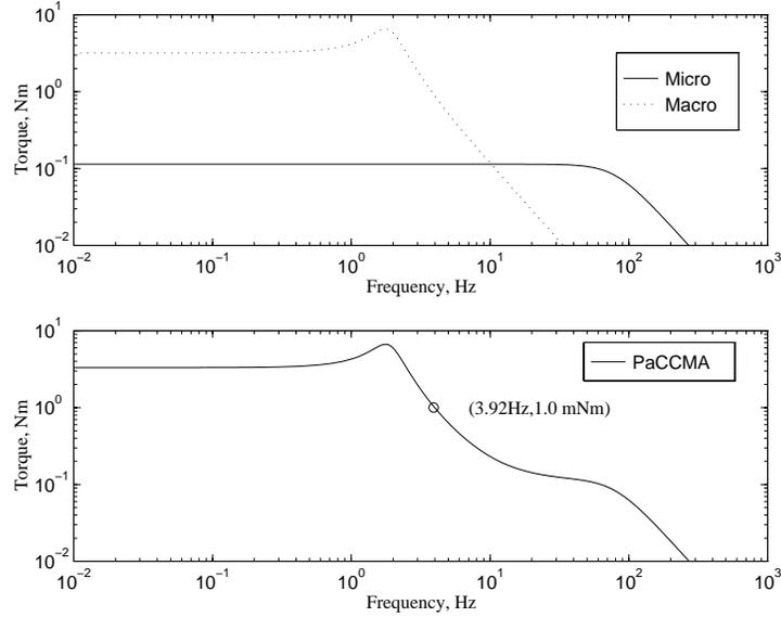
Figure 4-6: **Maximum Force vs. Frequency.** The top graph shows the micro and macro-actuator responses independently while the bottom graph shows the PaCCMA response. The PaCCMA response is the sum of the two responses due to the parallel arrangement.
