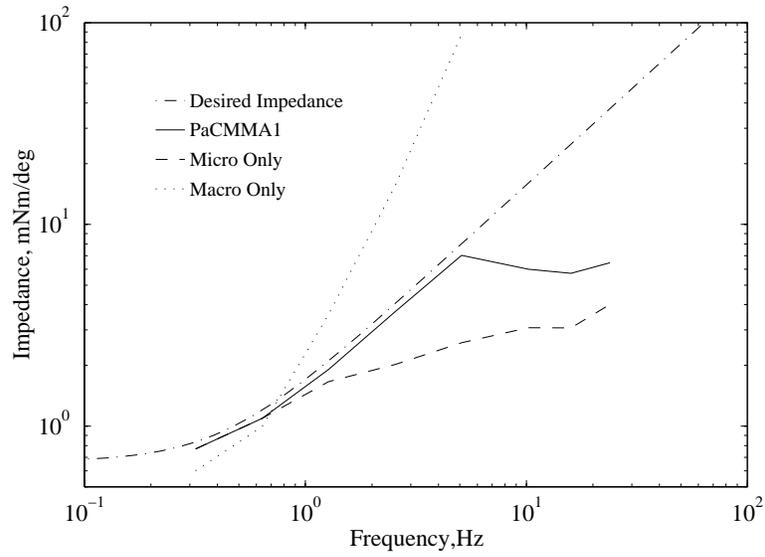
Figure 7-22: **Programmed Impedance.**  $Z(s) = 0.67 + 0.25s$  (Large Displacement)
