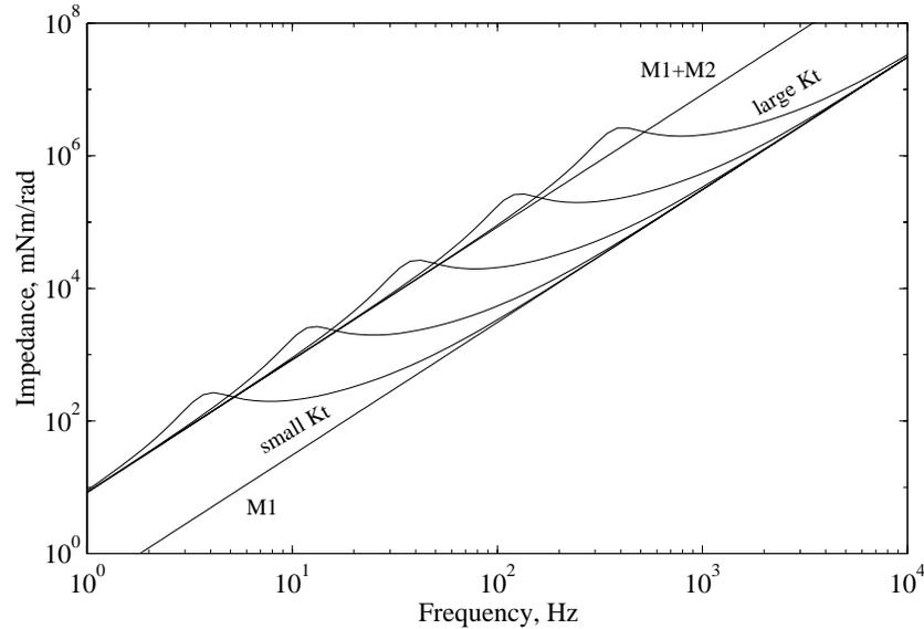
Figure 6-2: **Passive Impedance for Varied Transmission Stiffness.** The passive impedance of the system was calculated using equation 4.17 and the parameters in Appendix A. Inputs  $F_1$  and  $F_2$  were set to zero. Two asymptotes,  $M_1 s^2$  and  $(M_1 + M_2) s^2$  are also shown. The transmission stiffness,  $K_t$ , was given the following values: 114,  $1.14 \times 10^3$ ,  $1.14 \times 10^4$ ,  $1.14 \times 10^5$ ,  $1.14 \times 10^6$  mNm/rad.
