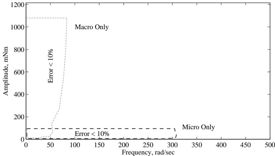
Figure 7-9: **Force Performance Space for Macro and Micro Actuators.** The force control response data of section 7.2.1 (explicit force control) was analyzed to determine the amplitudes and frequencies at which the RMS error was less than 10%.
