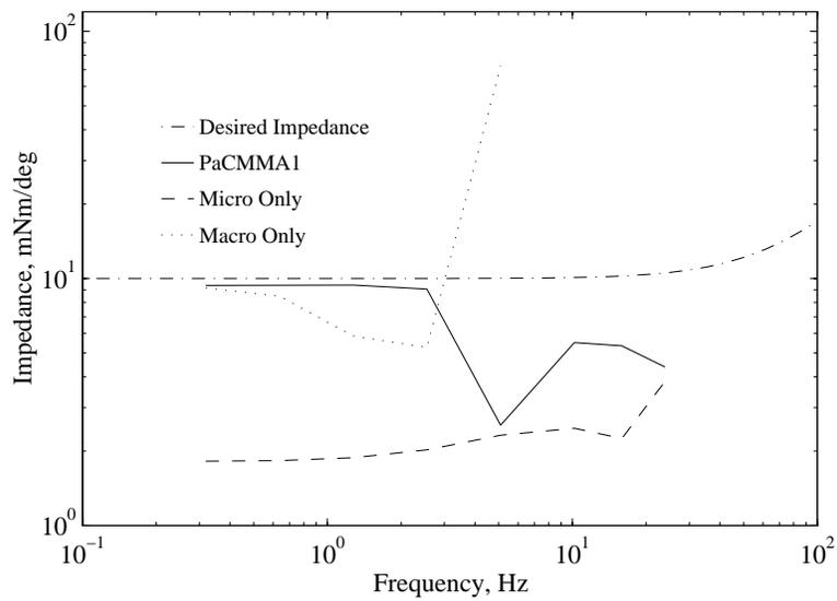
Figure 7-24: **Programmed Impedance.**  $Z(s) = 10 + 0.02s$  (Large Displacement)
