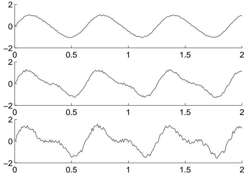
Figure 3-3: **Distortion Example.** These three graphs show examples of distorted signals. The values of Signal Fidelity for these graphs are 0.99, 0.86, and 0.74. Distortion is 1%, 14%, and 26% respectively.
