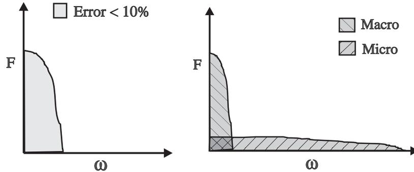
Figure 3-4: **Force Control Performance Space.** The regions are bounded by curves of constant error.
