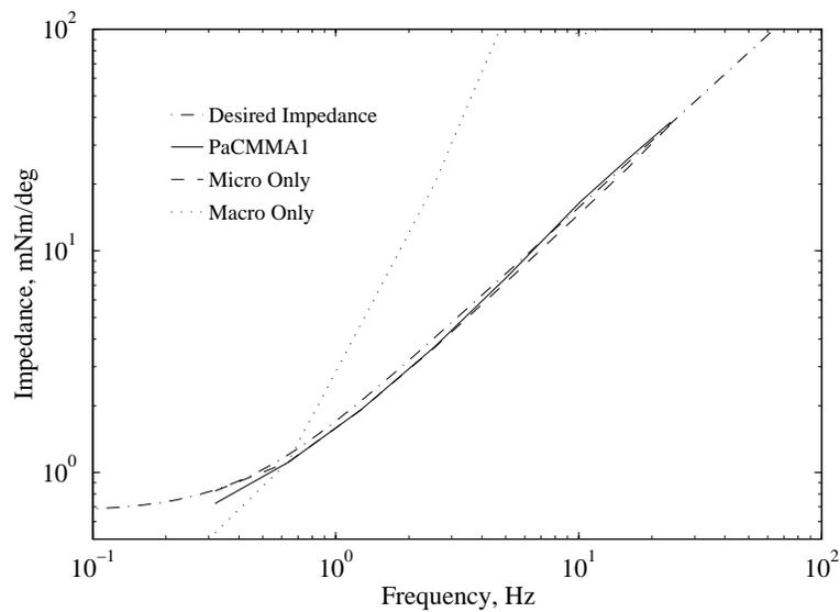
Figure 7-21: **Programmed Impedance.**  $Z(s) = 0.67 + 0.25s$  (Small Displacement)
