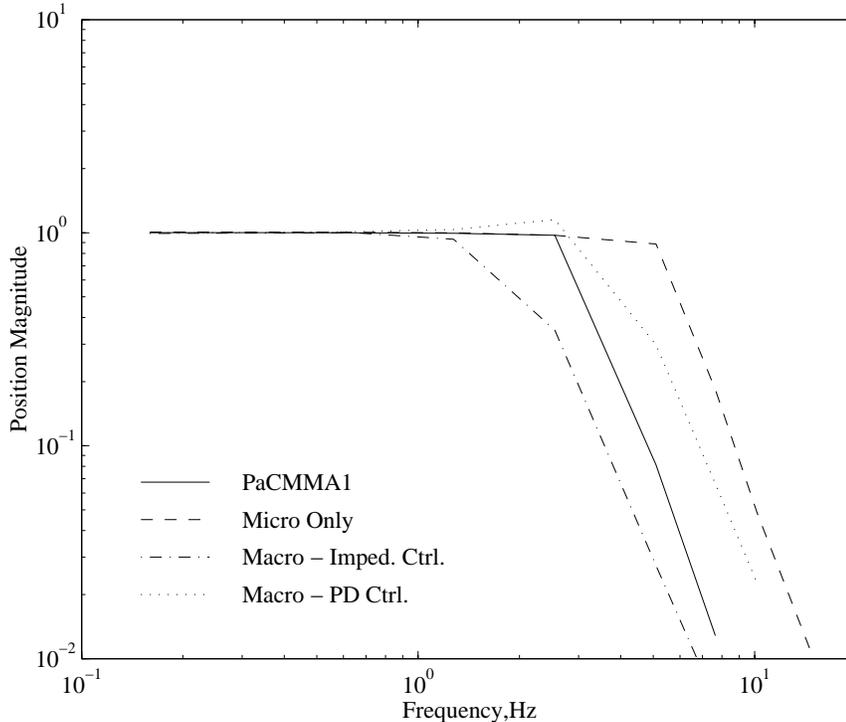
Figure 7-13: **Large Signal Position Bandwidth.**  $X_{des} = 62.0$  degrees
