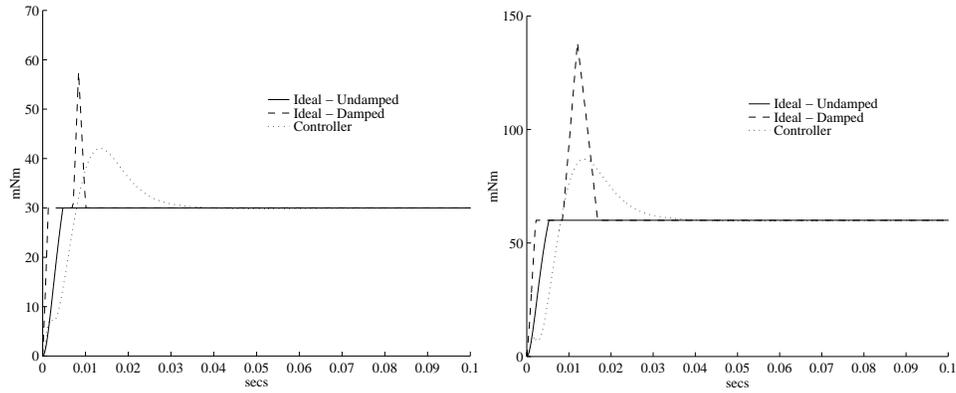
Figure 5-7: **Simulated Force Step Response.**  $F_{des} = 30$  mNm and  $F_{des} = 60$  mNm. This figure shows a comparison of three systems: Bang-bang control on an undamped transmission, bang-bang control on a damped system and the PaCMMA force controller. For the damped case,  $\zeta = 0.25$ .
