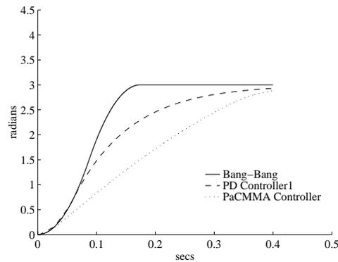
Figure 5-11: **Simulated Position Step Response.**  $x_{des} = 3.0\text{rad}$
