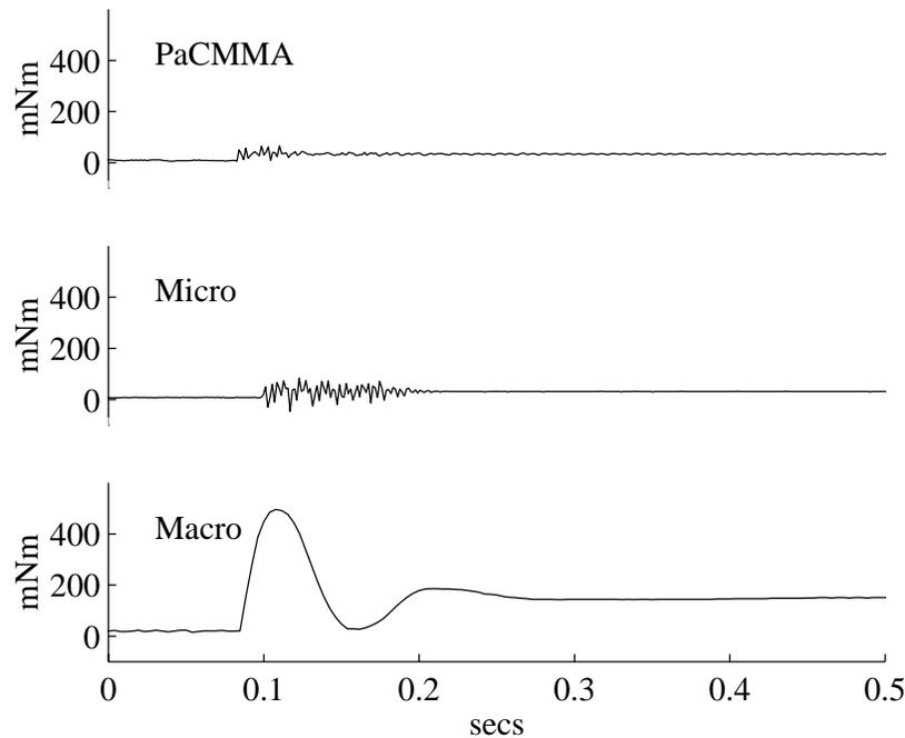
Figure 7-17: **Impact Response.**  $V_o = 1.9$  rad/sec. This graph shows the drastic reduction in impact force when a compliant transmission is attached to the macro-actuator in the PaCMMMA system. Notice that the PaCMMMA transients settle more quickly than even the micro-actuator by itself.
