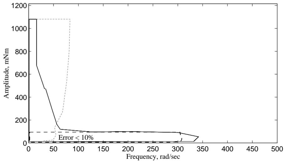
Figure 7-10: **Force Performance Space for PaCMMA1.** The performance space of the micro and macro-actuators is included. This shows how the PaCMMA's parallel coupling of the micro and macro-actuators can be used to get better performance than either actuator operating alone.
