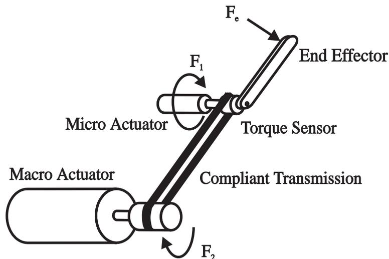
Figure 2-1: The Parallel Micro-Macro Actuator Concept
