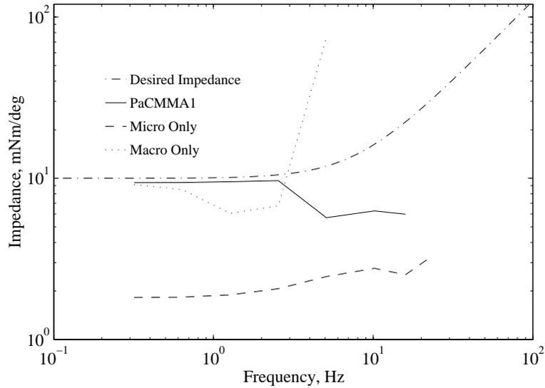
Figure 7-20: **Programmed Impedance.**  $Z(s) = 10 + 0.66s$  (Large Displacement). For large disturbances, the PaCMMA outperforms both the micro and macro-actuators. The micro-actuator saturates and can not produce enough force. An additional benefit of the PaCMMA is that its high frequency impedance is much lower than the macro-actuator.
