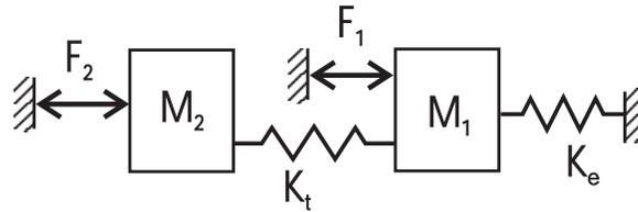
Figure 5-5: Lumped Element Model of PaCMMA
