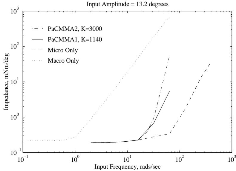
Figure 7-11: **Small Amplitude Impedance Response.** Impedance response data is shown for  $F_{des}=0$ . All systems used explicit force control algorithms.
