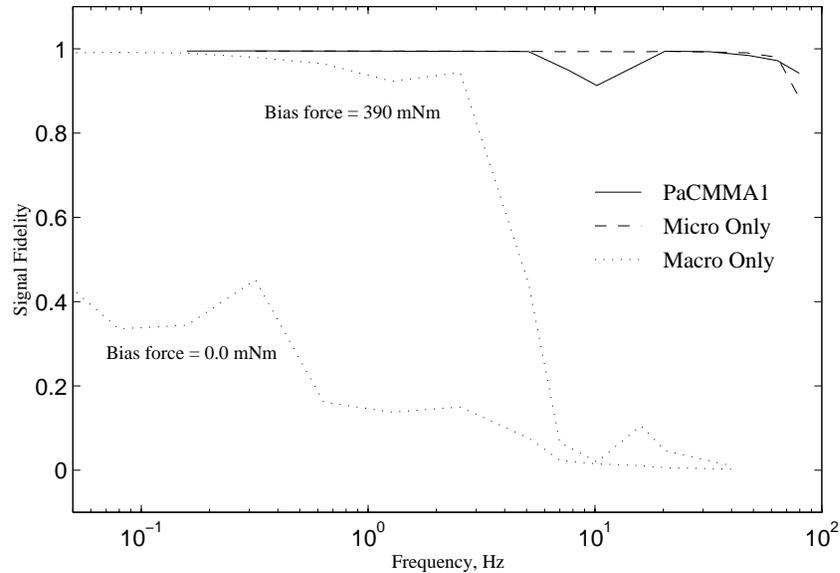
Figure 7-7: **Small Signal Distortion.**  $F_{des} = 13$  mNm. The figure shows that the PaCMMA and the micro-actuator perform much better than the macro-actuator for small amplitude force commands. While a force bias improves the performance of the macro-actuator somewhat, it is still not as accurate as the PaCMMA or the micro-actuator.
