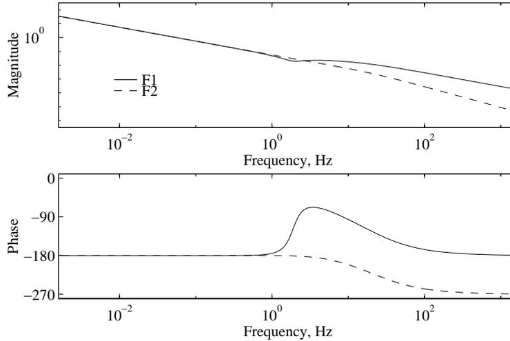
Figure 4-2: **Frequency Response in free space.**  $\frac{X_1(s)}{F_1(s)}, \frac{X_1(s)}{F_2(s)}$  where  $X_1$  is the displacement of the endpoint,  $F_1$  is the force command to the micro-actuator and  $F_2$  is the force command to the macro-actuator.
