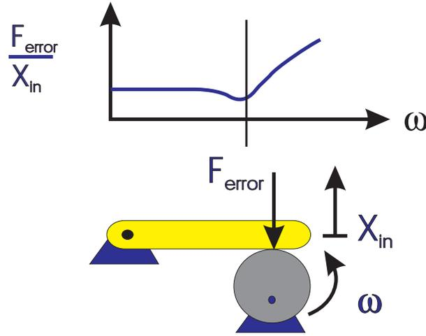
Figure 3-2: **Impedance Response.** Impedance response is a frequency response measurement which is obtained by commanding constant force and measuring the force error which results as the endpoint is moved. Impedance bandwidth may be defined as the frequency where the force error begins to increase with frequency.
