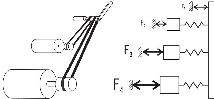
Figure 6-5: N-Actuator Concept
