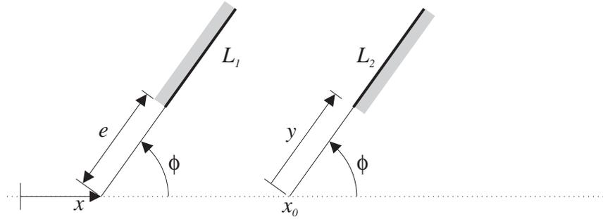
Figure A-20: Geometry used to implement a translating slider-stop. The position of one slider is measured positive to the left with  $x$ . The position of the other slider (the one that acts as a stop) is measured by displacement  $y$  along a fixed guide inclined an angle  $\phi$  from horizontal. This guide intersects the path of the other slider at  $x_0$ .
