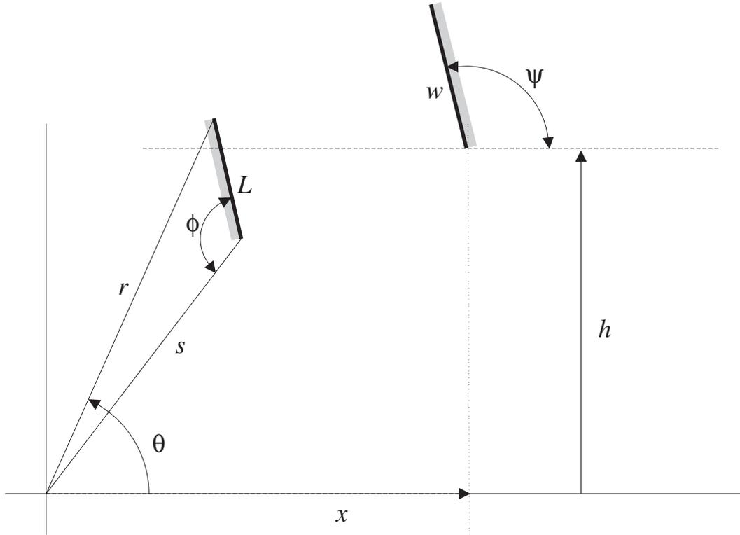
Figure 7-2: The parameterization of a pair of faces used to implement qcs-curve H. The rotating face rotates about the origin, its position measured positive counterclockwise with angle  $\theta$ . The translating face translates horizontally, its position measured positive to the right with  $x$ . Shading indicates the back sides of the faces, i.e., the sides that are inside the solids containing the faces.
