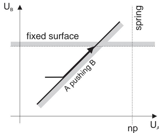
Figure 2-15: The qc-space of the two blocks modified to produce the desired behavior.
