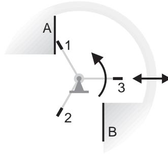
Figure 1-12: The stylized sketch of the yoke and rotor as actually input to SKETCHIT. The faces on the yoke are labeled A and B; those on the rotor are labeled 1–3. Each of the rotor faces is intended to engage each of the yoke faces.
