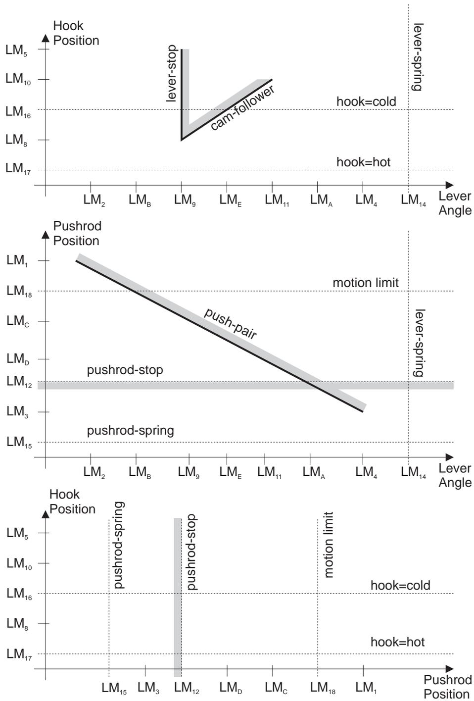
Figure 3-1: A candidate qc-space for the circuit breaker.
