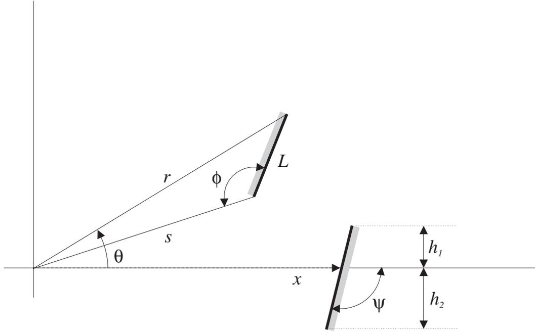
Figure 7-7: The parameterization of a pair of faces used to implement qcs-curve H. The rotating face rotates about the origin, its position measured positive counterclockwise with angle  $\theta$ . The translating face translates horizontally, its position measured positive to the right with  $x$ . Shading indicates the back sides of the faces, i.e., the sides that are inside the solids containing the faces.
