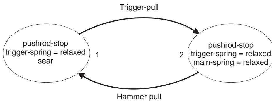
Figure 1-10: The desired behavior of the firing mechanism.
