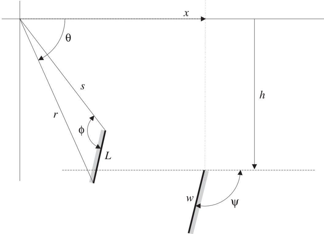
Figure 7-6: The parameterization of a pair of faces used to implement qcs-curve B. The rotating face rotates about the origin, its position measured positive *counterclockwise* with angle  $\theta$ . The translating face translates horizontally, its position measured positive to the right with  $x$ . Shading indicates the back sides of the faces, i.e., the sides that are inside the solids containing the faces.
