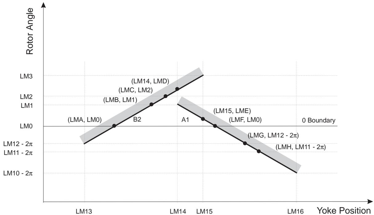
Figure 7-26: A reconstruction of the boundary-crossing qcs-curves from the yoke and rotor qc-space. The pieces of the boundary-crossing curves near the  $2\pi$  boundary in Figure 7-25 have been moved below the 0 boundary by subtracting  $2\pi$  from the ordinates of their end points and i-points. The small black circles with accompanying coordinate tuples are i-points. Although the qcs-curves are drawn as straight lines, they can have any shape as long as they are monotonic.
