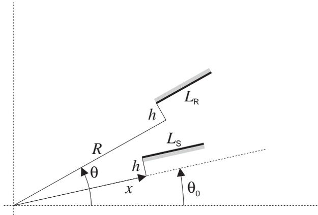
Figure A-14: Geometry used to implement a translating rotor-stop. The position of the rotor is measured positive counterclockwise with angle  $\theta$ . The translating face slides along a guide located at angle  $\theta_0$ .
