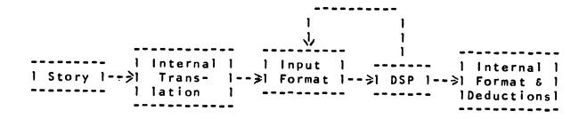
The arrow from DSP back to input format is to indicate that the input will be steadily modified in the process of applying DSP.
