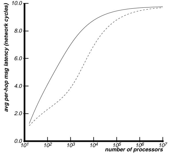
Figure 6: Average per-hop message latency  $T_h$  vs. number of processors  $N$ . The solid line represents the application of Section 3 running with two hardware contexts, assuming random communication patterns. The dashed line shows the impact of increasing the computation grain of that application by a factor of ten.
