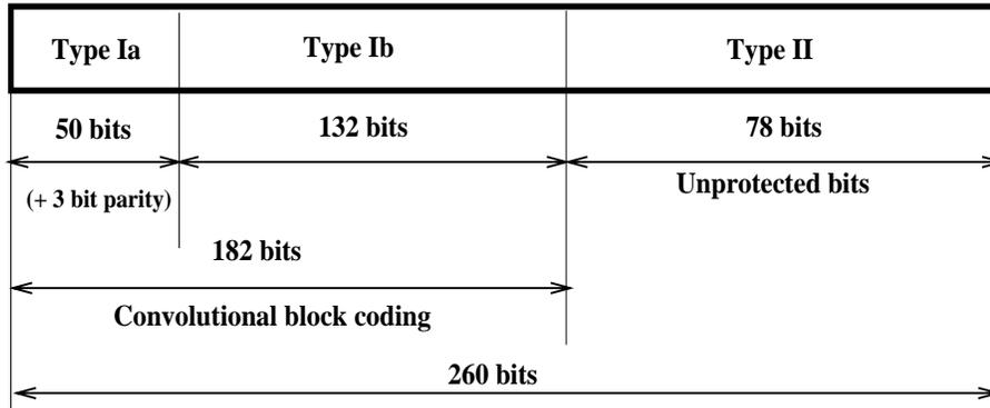
Figure 5: Audio sample: 1 block = 260 bits (20 ms)
