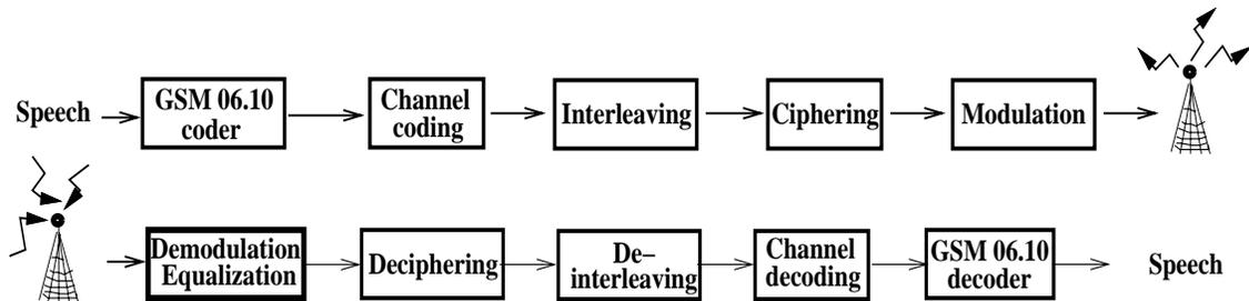
Figure 3: The sequence of operations
