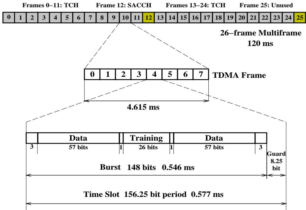
Figure 2: The TDMA frame structure
