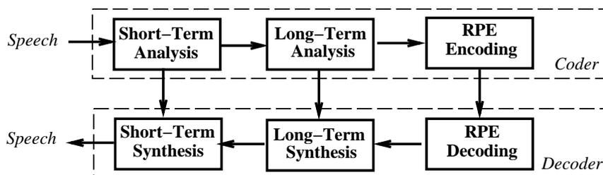
Figure 4: A block diagram of the GSM 06.10 codec
