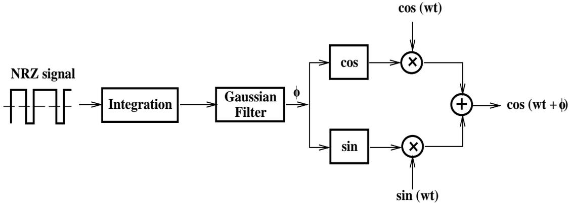
Figure 8: GMSK modulation block diagram
