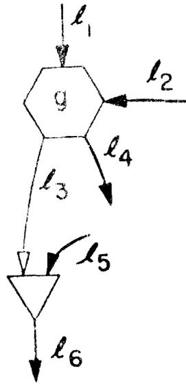
Fig. 3.9 The Link Names of Loop Junction-Loop Output Pairs
