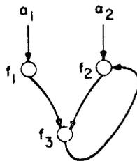
Fig. 3.7 A Cycle that does not Pass Through a Loop Junction
