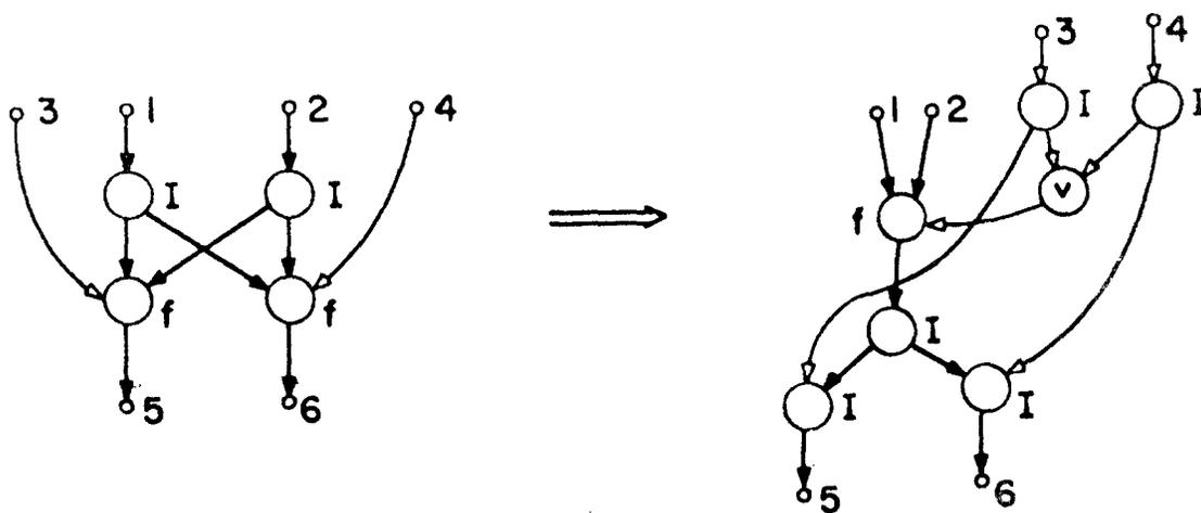
Fig. 4.6 Alternative Form of a Transformation Scheme Which Does Not Preserve Equivalence
