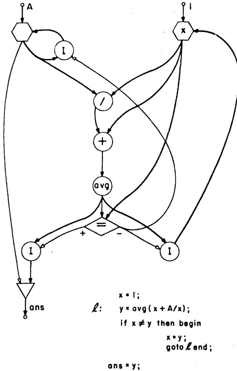
Fig. 2. 6 A Single Loop with Multiple Loop Junctions
