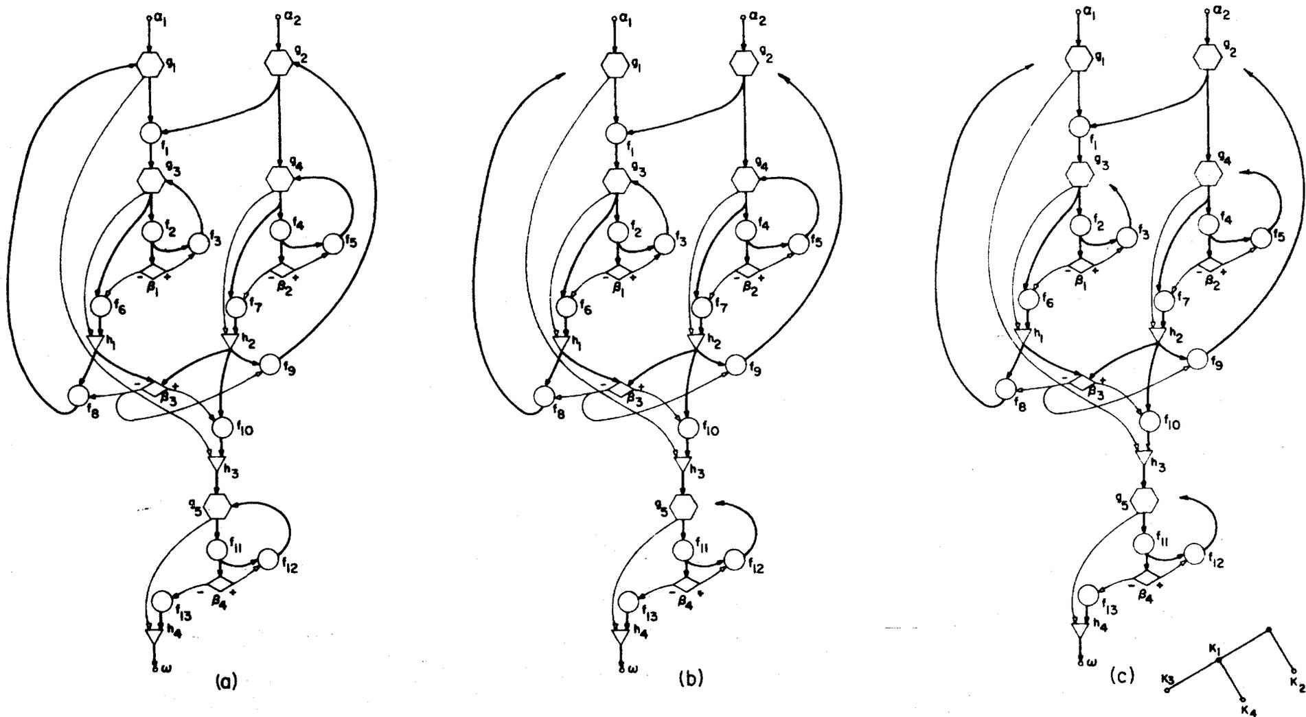
Fig. 3.8 Example of the Cycle Decomposition Procedure
