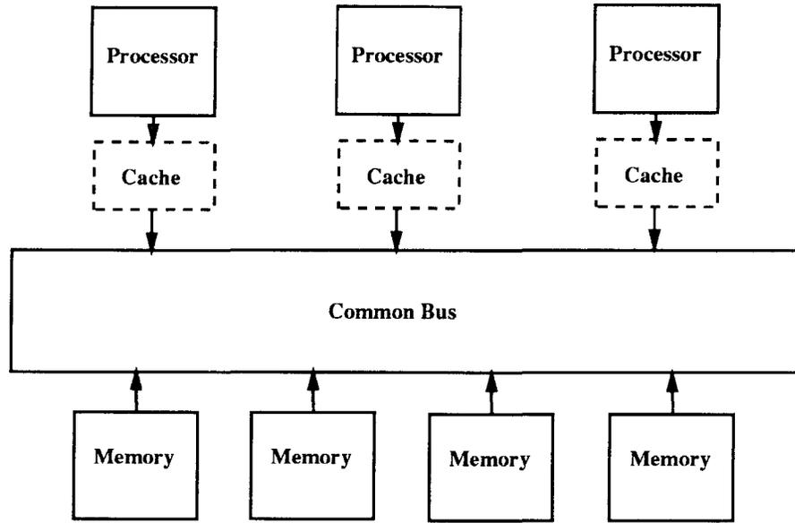
Figure 4-2: Typical bus-based architecture supported by the simulator.
