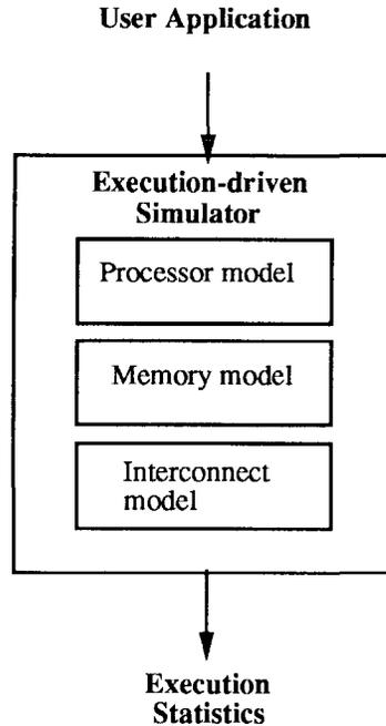
Figure 2-3: Typical structure of an execution-driven simulation system.
