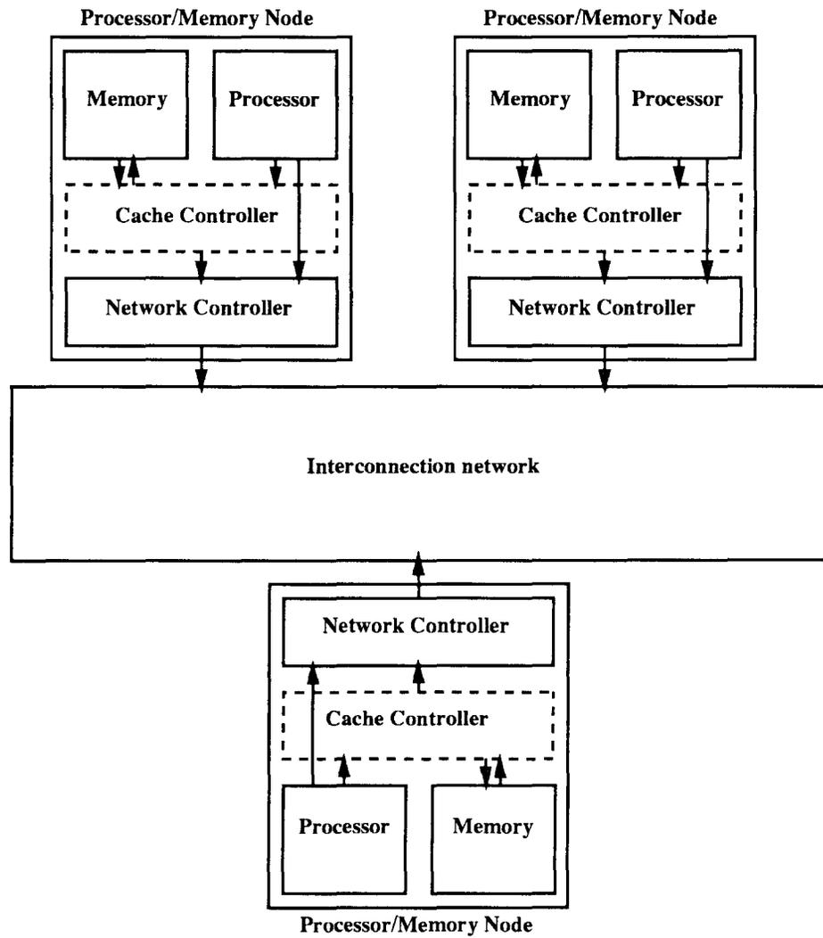
Figure 4-3: Typical network-based architecture supported by the simulator.
