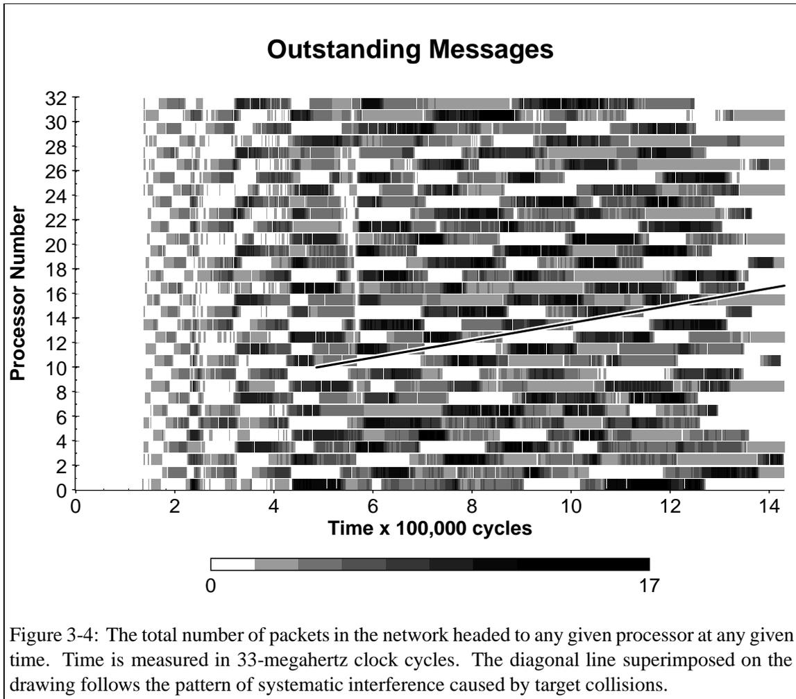
Figure 3-4: The total number of packets in the network headed to any given processor at any given time. Time is measured in 33-megahertz clock cycles. The diagonal line superimposed on the drawing follows the pattern of systematic interference caused by target collisions.
