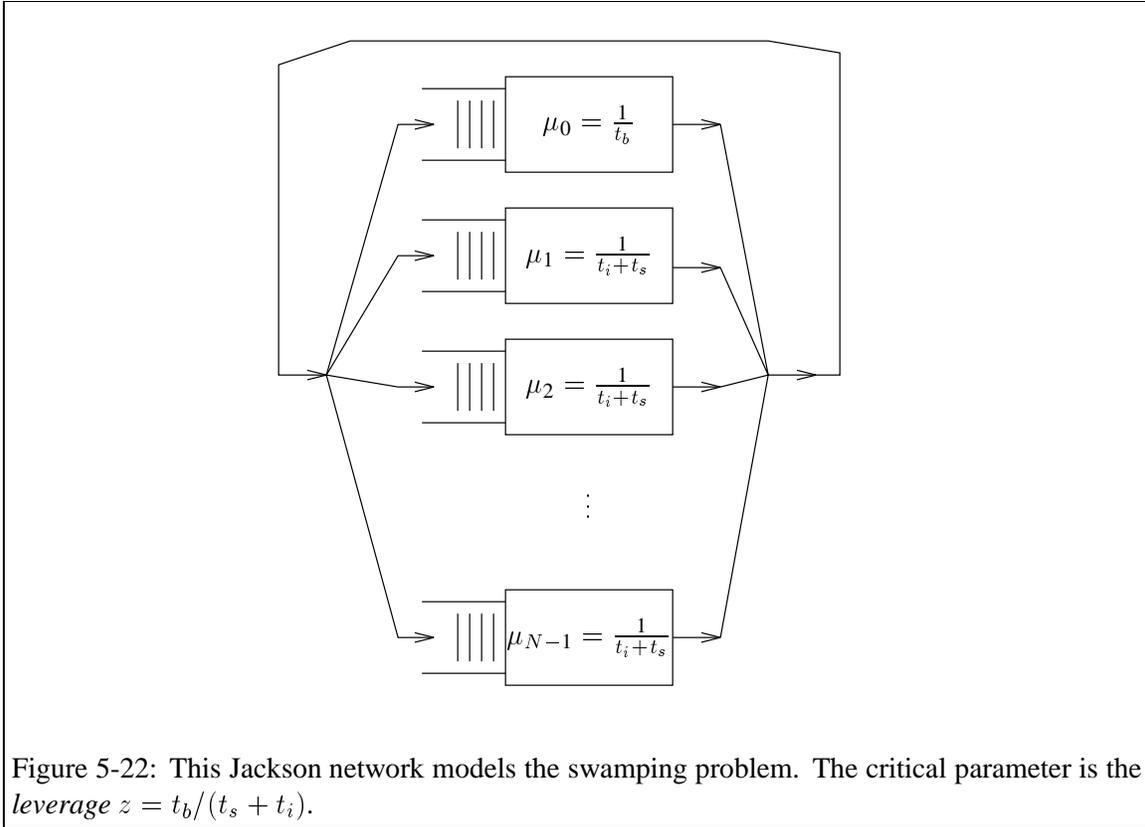
Figure 5-22: This Jackson network models the swamping problem. The critical parameter is the leverage  $z = t_b/(t_s + t_i)$ .
