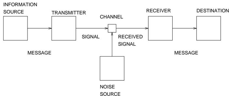
**Figure 1-1:** Shannon’s schematic of a communication system.
