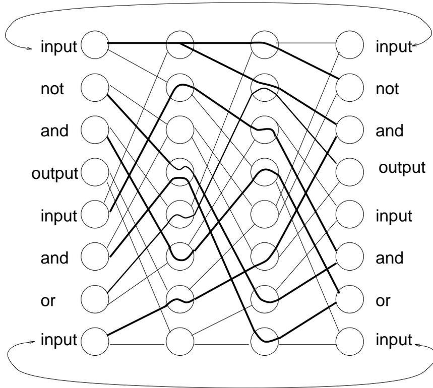
**Figure 4-7:** A drawing of the circuit on a wrapped de Bruijn graph. The left and right columns of the graph should be identified with one another, but are drawn twice for the convenience of the artist. Dark lines correspond to wires in the circuit.
