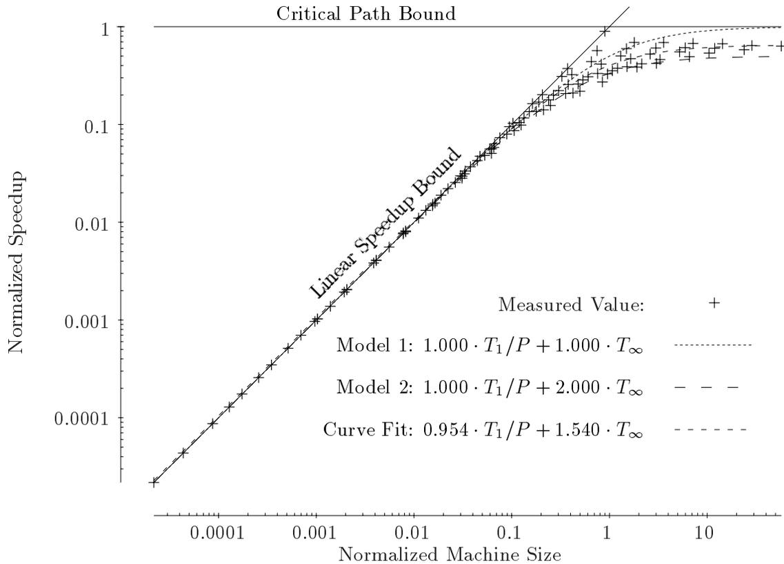
**Figure 5.14:** Normalized speedups for the knary synthetic benchmark using from 1 to 256 processors. The horizontal axis is the number  $P$  of processors and the vertical axis is the speedup  $T_1/T_P$ , but each data point has been normalized by dividing by  $T_1/T_\infty$ .
