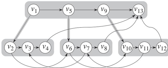
**Figure 2.9:** The dependency edges in this computation form cycles through all of the child threads, though they do not create any cycle of instructions. Any execution schedule must have all 4 of this computation's threads simultaneously living at some step. This computation is not depth-first, since the dependency edges,  $(v_7, v_3)$  and  $(v_{11}, v_7)$ , violate the left-to-right depth-first order,  $v_1, v_2, \dots, v_{13}$ .
