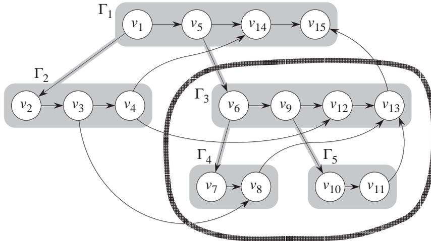
**Figure 3.2:** The spawn edge  $(v_5, v_6)$  and the dependency edges,  $(v_4, v_{12})$  and  $(v_3, v_8)$ , pass arguments into the subcomputation rooted at thread  $\Gamma_3$ . This computation is not strict.
