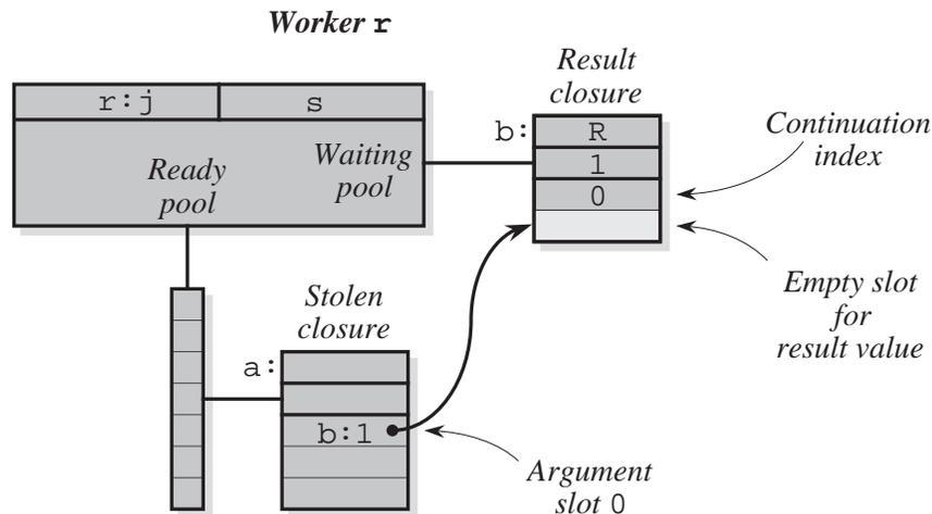
**Figure 6.5:** When the thief worker  $r$  steals a closure  $a$  which contains a continuation in its argument slot 0, the thief replaces this continuation with a new continuation referring to an empty slot in a newly allocated result closure  $b$ . Additionally, the thief stores the continuation's slot number 0 in an argument slot of the result closure.
