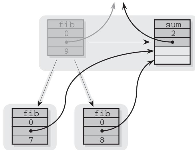
**Figure 5.9:** When the `fib` thread spawns children, it creates for each child a new closure with `fib` as the thread and no empty argument slots. Each child closure has a continuation referring to an empty slot in the parent's successor closure. Each child thread is the initial thread of a new child procedure.
