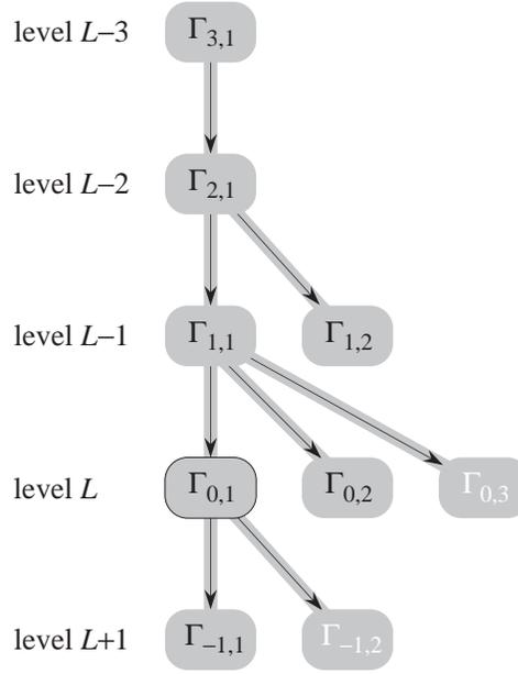
**Figure 5.19:** The structure of procedures in a processor's ready pool. The processor  $p$  is executing a thread of procedure  $\Gamma_{0,1}$  at level  $L$ . In this example, we have  $l = 3$ , so for each  $i = 0, 1, 2, 3$ , the procedures  $\langle \Gamma_{i-1,j} \rangle$  are tuple children of  $\Gamma_{i,1}$ . The procedures  $\Gamma_{0,3}$  and  $\Gamma_{-1,2}$  must be ghost procedures.
