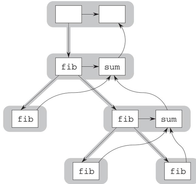
**Figure 5.10:** The dag grown by an execution of the Fibonacci program. Dag edges created by `spawn_next` are horizontal; dag edges created by `spawn` are straight, shaded, and point downward; and dag edges created by `send_argument` are curved and point upwards. The background shading groups the threads into procedures.
