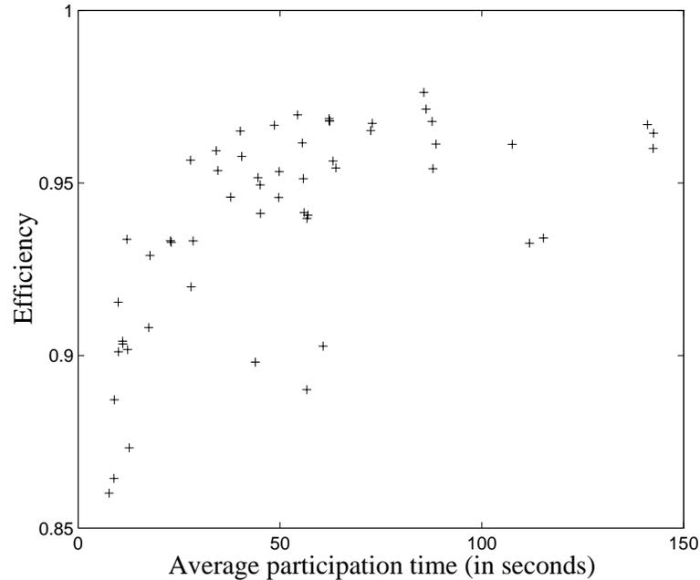
**Figure 6.7:** This plot shows the efficiency of 8-processor executions of the `knary(11, 6, 2)` program as a function of the amount of adaptiveness. The adaptiveness is measured as the average amount of time each worker participated in the job. The efficiency is measured as the ratio of the work in the computation to the total worker execution time.
