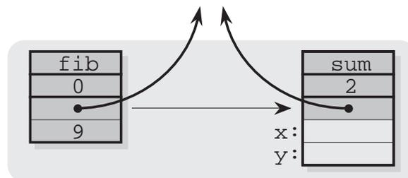
**Figure 5.8:** When the `fib` thread spawns its successor `sum`, it creates a new closure with `sum` as the thread and two empty argument slots referred to by the continuations `x` and `y`. The background shading denotes that both threads are part of the same procedure.
