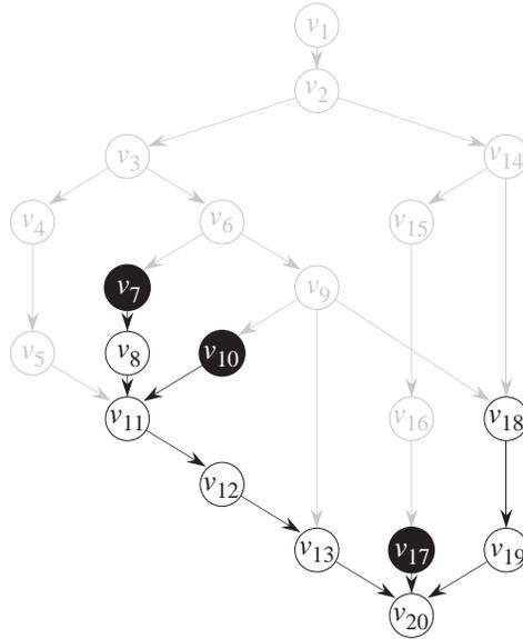
**Figure 2.5:** Step 6 in the 3-processor execution of our example computation. The faint instructions have already been executed. The white-on-black instructions are the ones actually executed at this step. All 3 processors do work at this step.
