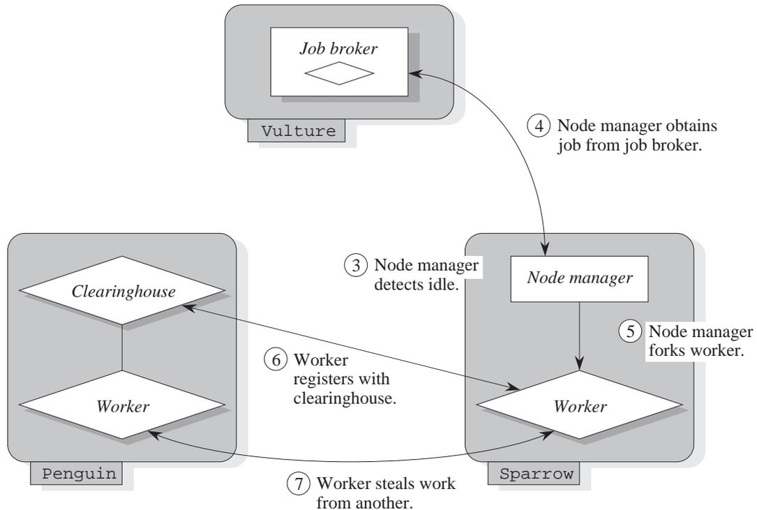
**Figure 6.2:** An idle machine joins a Cilk job. When the node manager detects that its machine is idle, it obtains a job from the job broker and then forks a worker. The worker registers with the clearinghouse and then begins work stealing.
