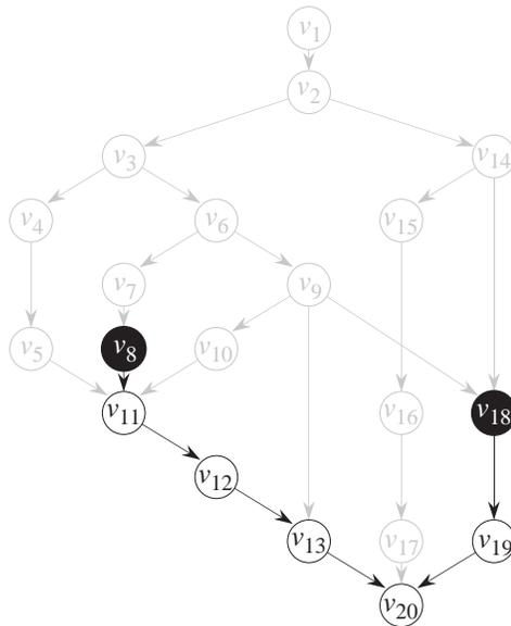
**Figure 2.6:** Step 7 in the 3-processor execution of our example computation. At this step a processor sits idle. Nevertheless, every instruction with in-degree 0 get executed, and consequently, the length of the critical path is reduced by 1.
