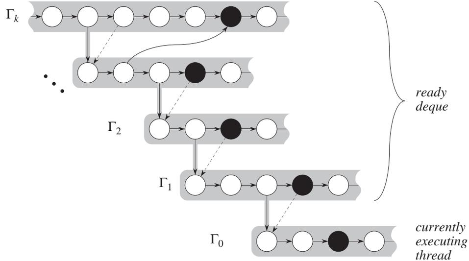
**Figure 4.1:** The structure of a processor’s ready deque. The black instruction in each thread indicates the thread’s currently ready instruction. Only thread  $\Gamma_k$  may have been worked on since it last spawned a child. The dashed edges are the “deque edges” introduced in Section 4.3.
