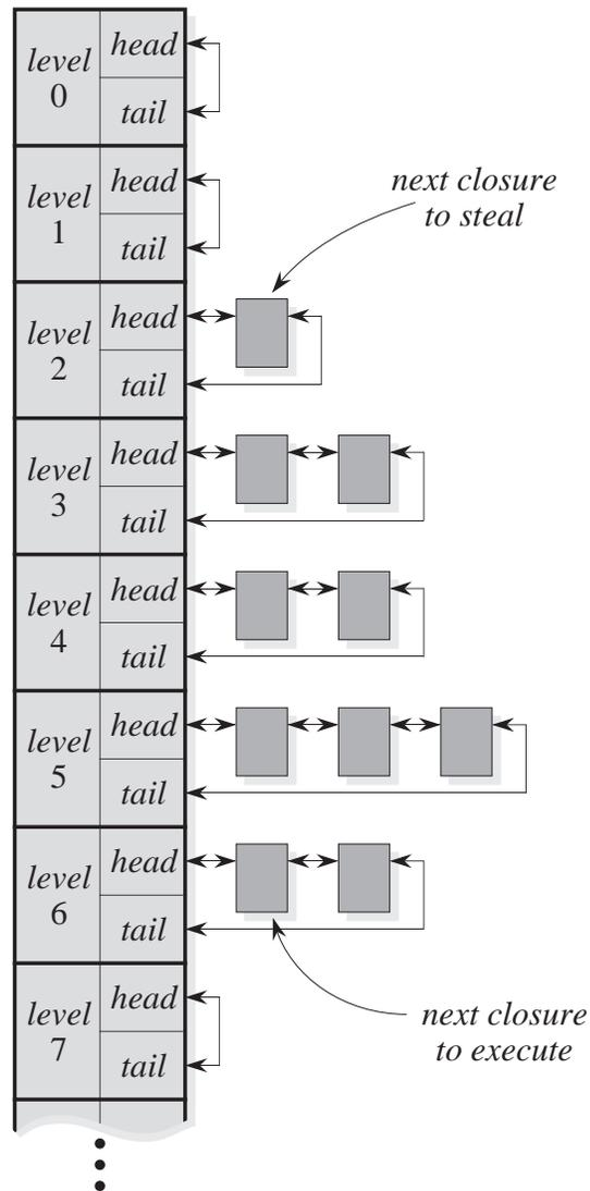
**Figure 5.11:** A processor's ready pool. At each iteration through the scheduling loop, the processor executes the closure at the head of the deepest nonempty level in the ready pool. If the ready pool is empty, the processor becomes a thief and steals the closure at the tail of the shallowest nonempty level in the ready pool of a victim processor chosen uniformly at random.
