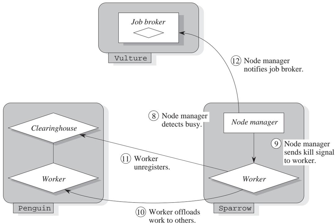
**Figure 6.3:** A no-longer-idle machine leaves a Cilk job. When the node manager detects that its machine is no-longer idle, it sends a kill signal to the worker. The worker catches this signal, offloads its work to other workers, unregisters with the clearinghouse, and then terminates.
