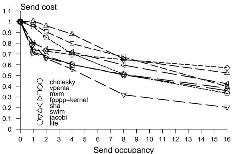
the registers for later use, Raw incurs a receive occupancy of one. Thus Raw is plotted showing a receive occupancy of one). The results indicate that occupancy impacts performance significantly -- performance drops by 10 to 30 percent even when the occupancy is increased by 1 cycle. It is clear from these results that scalar operand networks must implement zero cycle send and receive occupancy. Because it has the least parallelism, notice also that Sha is most affected by higher occupancies.
