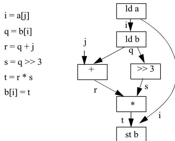
Figure 6: A code fragment and its dataflow graph
