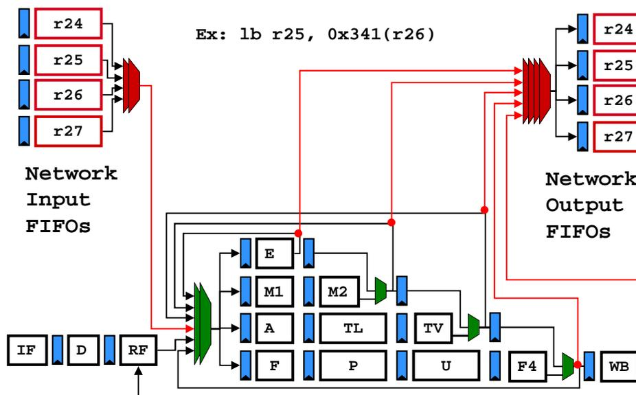
Figure 9: Directly integrating the network interfaces into the bypass paths
