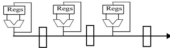
Figure 4: The operand network in the Multiscalar
