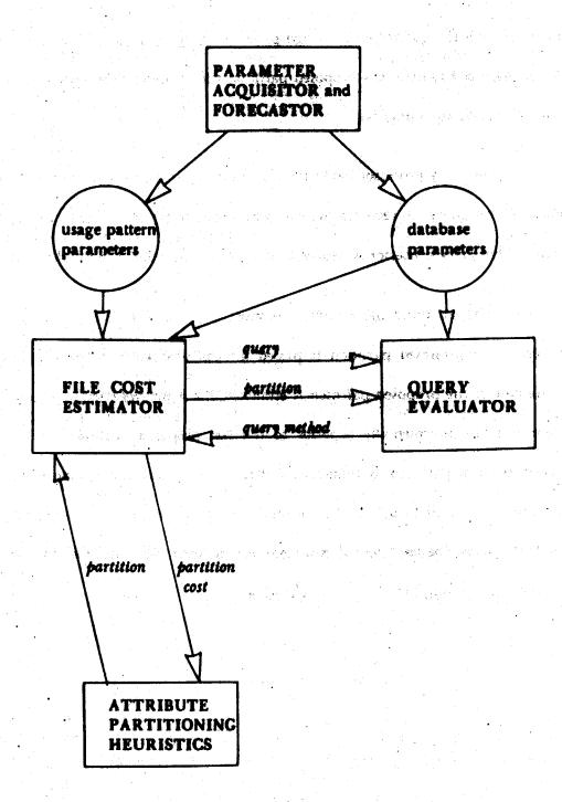
Figure 1 Block diagram of the attribute partitioning system.
