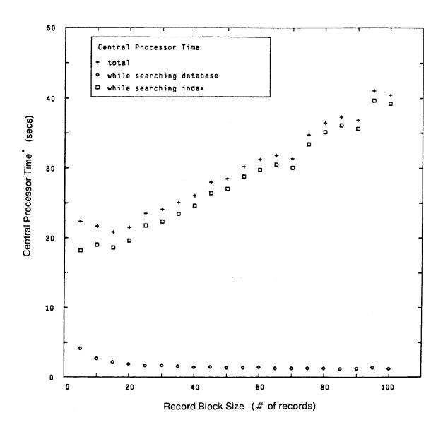
Figure B-10: Central Processor Time vs. Record Block Size, Buffer Size 2048
