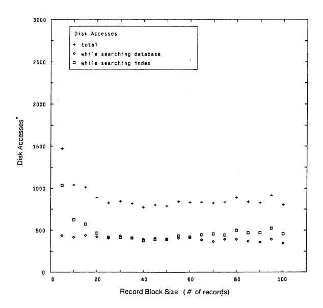
Figure B-4: Disk Accesses vs. Record Block Size, Buffer Size 1024
