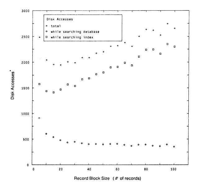
Figure B-1: Disk Accesses vs. Record Block Size, Buffer Size 128
