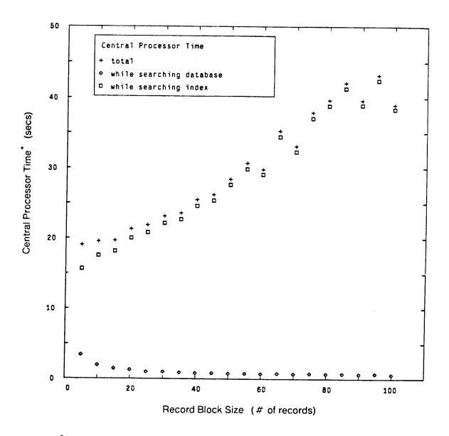
Figure 4-2: Central Processor Time vs. Record Block Size, Buffer Size 128
