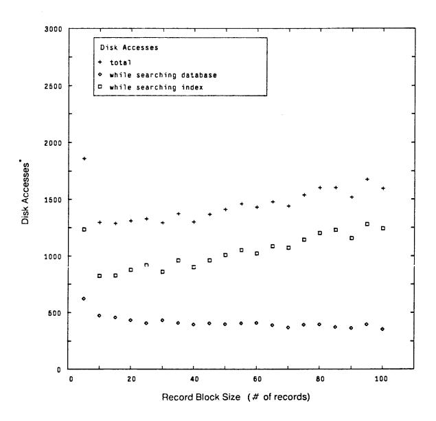
Figure B-2: Disk Accesses vs. Record Block Size, Buffer Size 256
