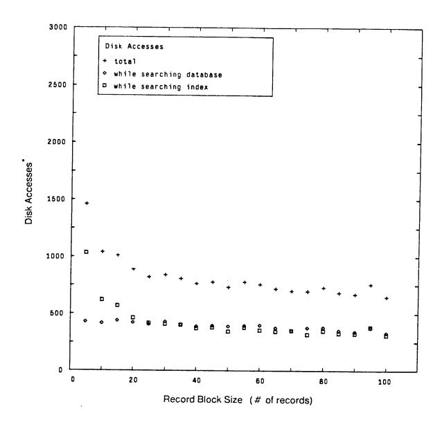
Figure B-5: Disk Accesses vs. Record Block Size, Buffer Size 2048
