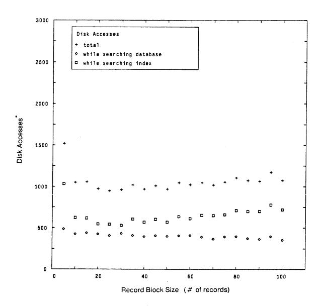
Figure B-3: Disk Accesses vs. Record Block Size, Buffer Size 512
