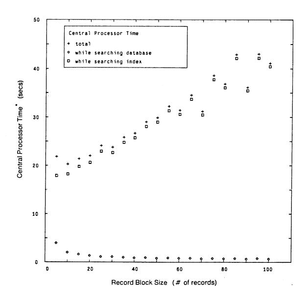
Figure B-7: Central Processor Time vs. Record Block Size, Buffer Size 256
