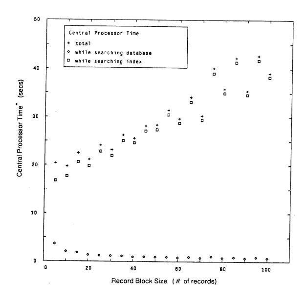
Figure B-8: Central Processor Time vs. Record Block Size, Buffer Size 512
