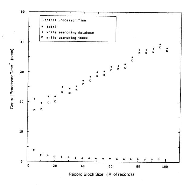
Figure B-9: Central Processor Time vs. Record Block Size, Buffer Size 1024
