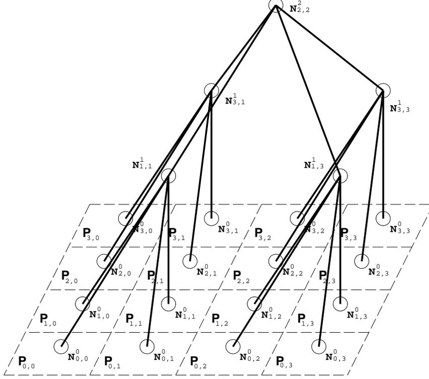
Figure 4-5: Embedding a Quad-Tree in a Two-Dimensional Mesh.
