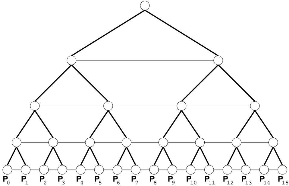
Figure 4-1: Binary X-Tree on a One-Dimensional Mesh Network: Labels of the form  $\mathbf{P}_i$  indicate physical processors. Circles indicate nodes in the X-Tree. Thick lines indicate parent-child links. Thin lines indicate near-neighbor links.
