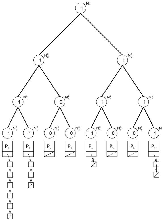
Figure 3-2: Combining Tree with Presence Bits: *The tree is distributed among the processors as described in Figure 3-1. Each node in the tree maintains a “presence bit,” which is turned on whenever any queue on any processor at any leaf on the subtree headed by that node contains at least one runnable thread.*
