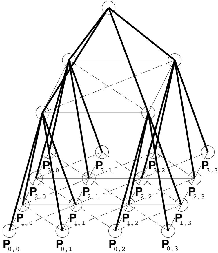
Figure 4-2: Quad-X-Tree on a Two-Dimensional Mesh Network: Labels of the form  $\mathbf{P}_{i_0, i_1}$  indicate physical processors. Circles indicate nodes in the X-Tree. Thick lines indicate parent-child links. Thin solid lines indicate near-neighbor links to edge-adjacent neighbors. Thin dashed lines indicate near-neighbor links to corner-adjacent neighbors.
