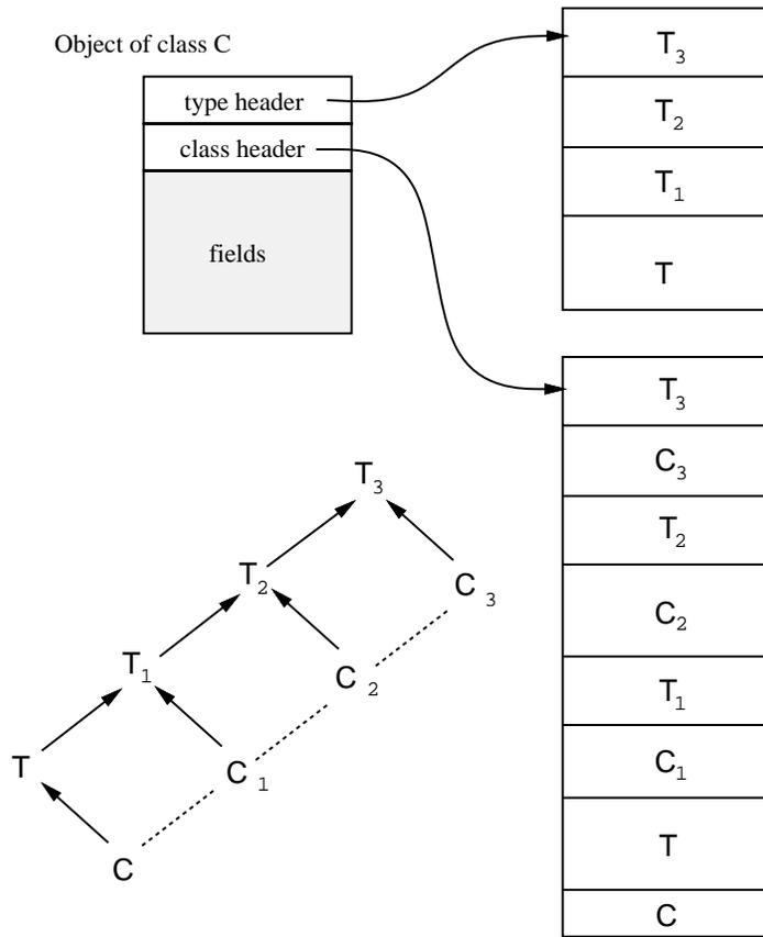
Figure 2-16: A class ladder and corresponding object layout
