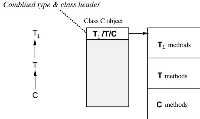
Figure 2-15: Result of merging type and class headers
