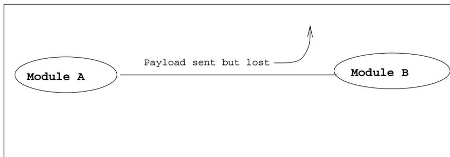
Figure 3.7: A Sends a Payload which is Lost
