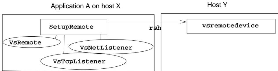
Figure 4.9: Setup Remote Called, Remote Device Script Started
