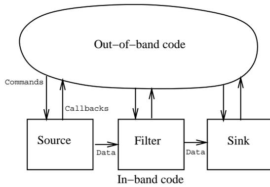
Figure 1.2: The structure of a simple VuSystem application
