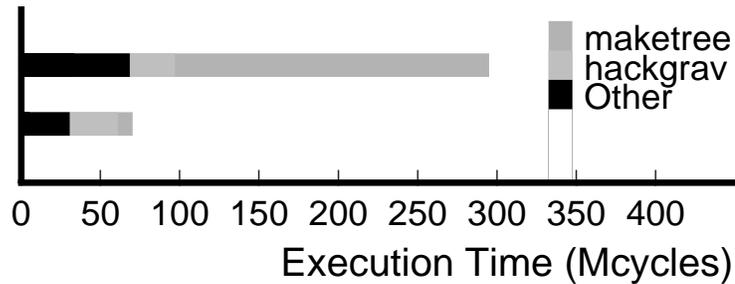
Figure 6.10: Breakdown of runtime in Barnes-Hut into major phases of computation. “maketree” is the parallel tree build phase, “hackgrav” is the force computation phase, and “Other” is all other computation. The top bar represents a 32-node DSSMP with an SSMP node size of 4, the bottom bar represents a 32-node Alewife machine.
