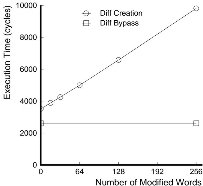
Figure 4.3: Overhead of Diff Creation and Diff Bypass as a function of the number of modified words in the page. Page size is 1K-bytes.
