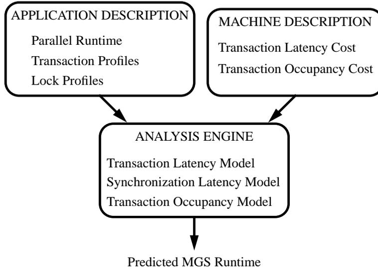
Figure 7.4: The performance analysis framework for multigrain systems.
