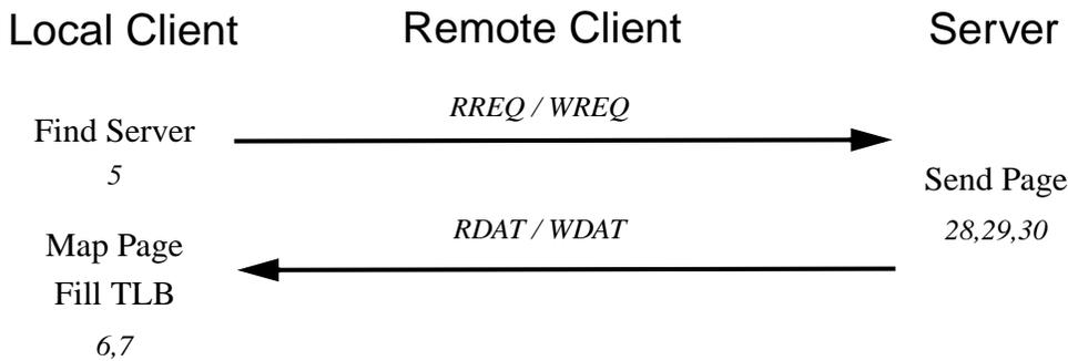
Figure 4.7: Page fault transactions in MGS. Each column represents a state machine. All italicized text, *e.g.* the message names and state transition numbers, refer to the state diagrams and state transition tables in Appendix A.
