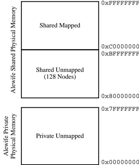
Figure 5.2: Memory map for the MGS system.
