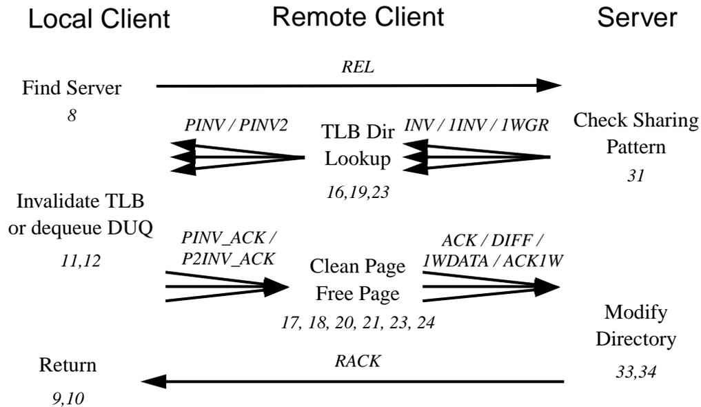
Figure 4.9: Release transactions in MGS. Each column represents a state machine. All italicized text, *e.g.* the message names and state transition numbers, refer to the state diagrams and state transition tables in Appendix A.
