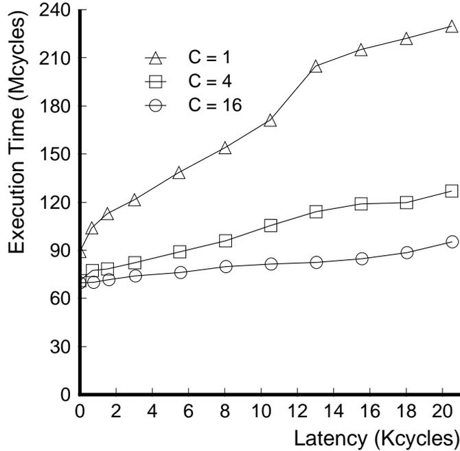
Figure 6.19: Latency sensitivity results for Water-Kernel with tiling.
