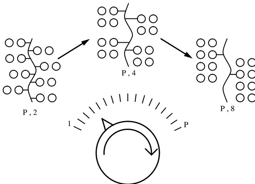
Figure 3.5: A family of DSSMPs is defined by fixing the total processing and memory resources, and varying the SSMP node size. The notation  $P, C$  denotes a DSSMP with  $P$  total processors, and  $C$  processors per SSMP node.
