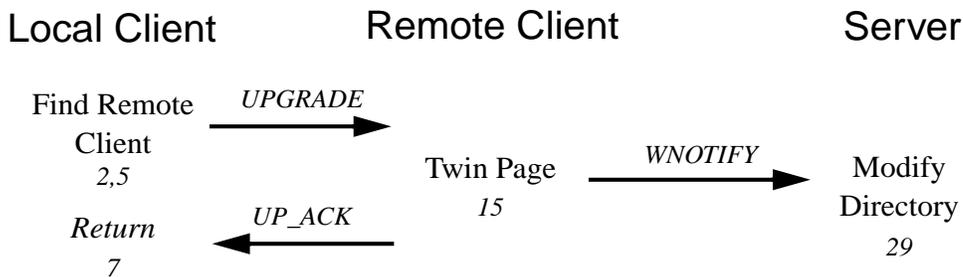
Figure 4.8: Page upgrade transactions in MGS. Each column represents a state machine. All italicized text, *e.g.* the message names and state transition numbers, refer to the state diagrams and state transition tables in Appendix A.
