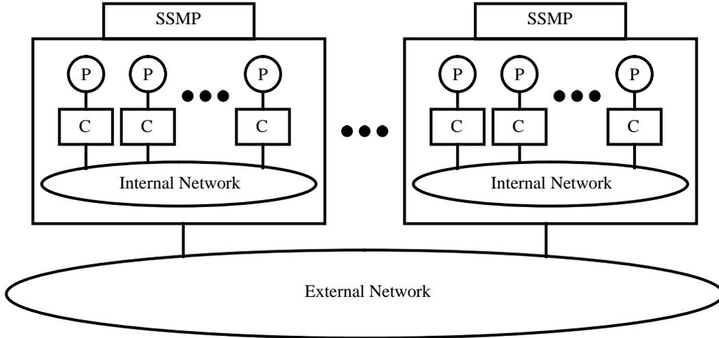
Figure 3.3: A Distributed Scalable Shared Memory Multiprocessor (DSSMP).
