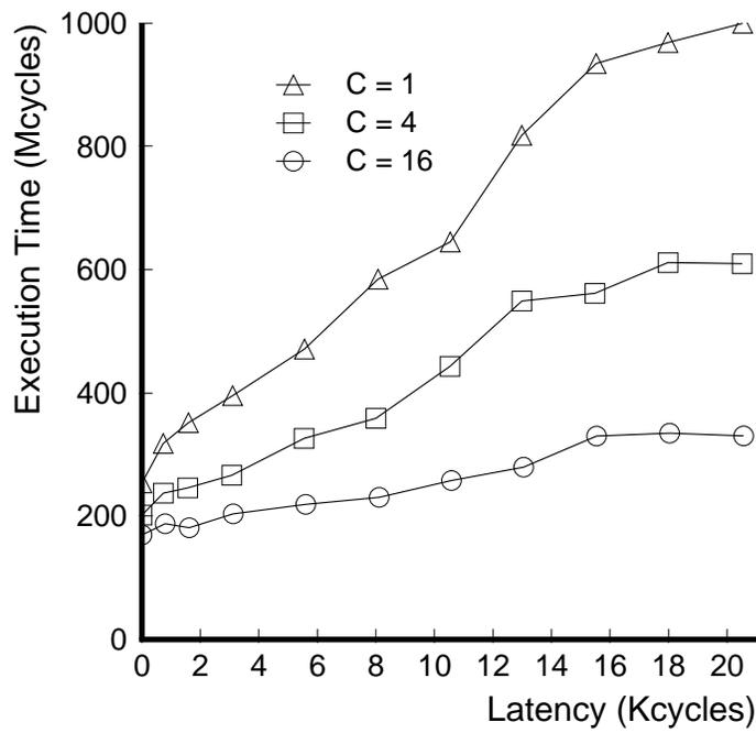
Figure 6.18: Latency sensitivity results for Water.
