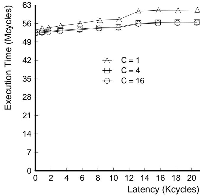
Figure 6.17: Latency sensitivity results for Jacobi.
