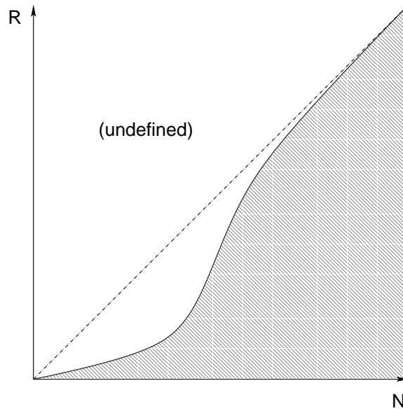
Figure 14: Phase plot showing regions of the  $N$ - $R$  phase space (shaded) where Sift performs well in comparison to 802.11. Both protocols degrade when  $N$  increases to infinity.  $N$  represents the number of sensors that respond to each event and  $R$  is the number of event reports required for each event.
