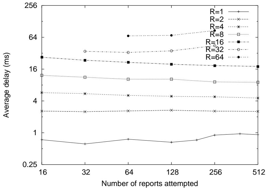
Figure 11: Average delay of Sift event reports as a function of  $N$ . We show curves for  $R$  (number of reports required) equal to powers of two between zero and 64. This experiment uses a constant-event-rate workload.
