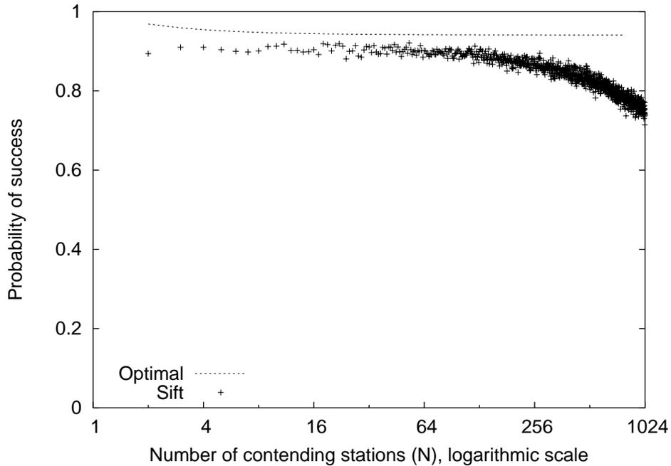
Figure 3: A comparison between Sift with  $\alpha = 0.82$  and  $CW = 32$ , and an optimal protocol, with  $CW = 32$ . The optimal protocol has full knowledge of  $N$ ; Sift has no knowledge of  $N$ . The Sift distribution shown above was engineered for a maximum value of  $N = 512$  nodes, but degrades gracefully when  $N$  exceeds that figure.
