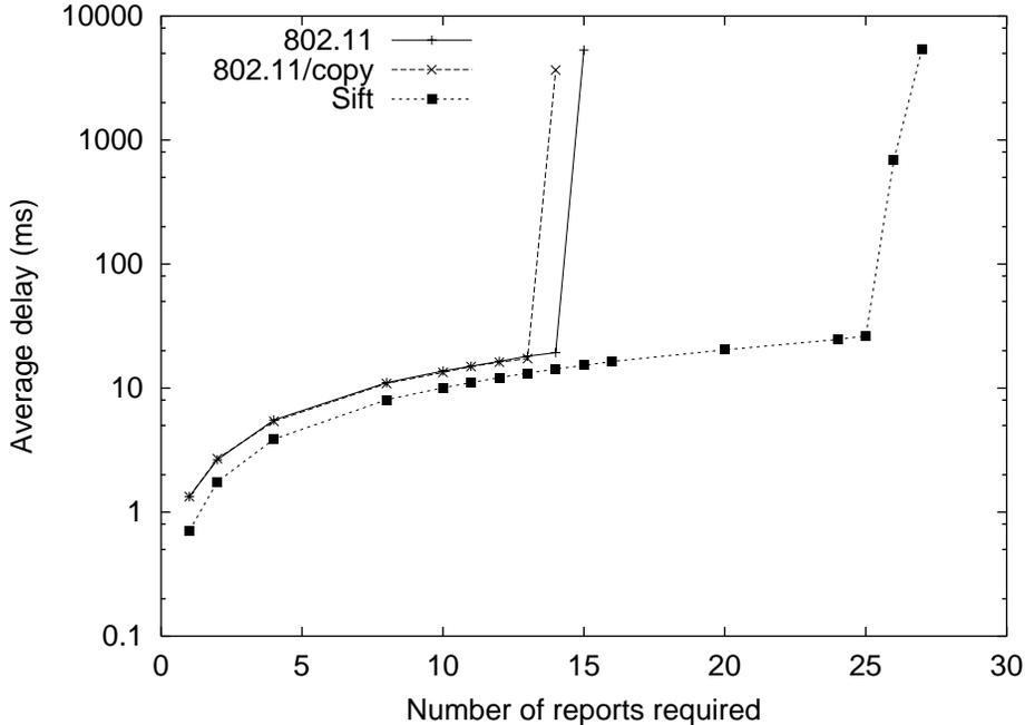
Figure 12: Average delay as a function of the number of reports  $R$  needed for each camera motion event. The sensor range in this experiment,  $d_{\text{report}}$  is fixed at 20. This experiment uses our trace-driven workload.
