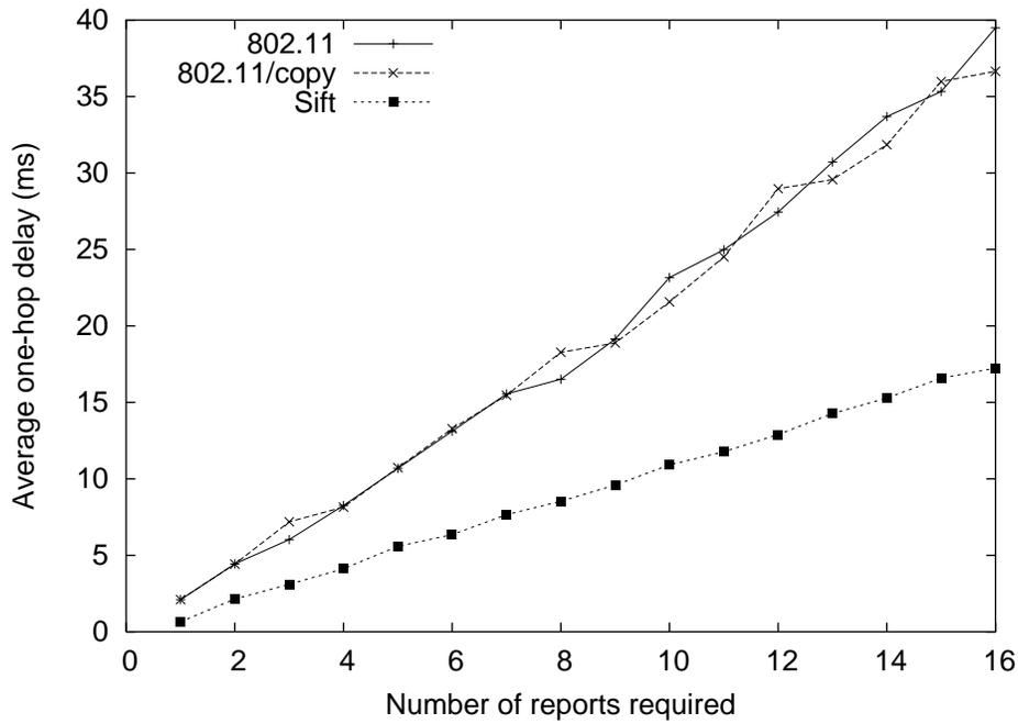
Figure 10: Average delay as a function of the number of event reports required when 128 sensors report an event ( $N = 128$ ). All sensors detect the event at the same time. This experiment uses a constant-event-rate workload.
