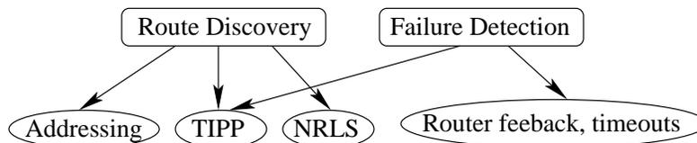
Figure 4-1: Dependency between the function modules (route discovery and failure detection) and the mechanisms.
