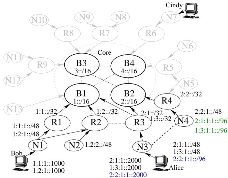
Figure 5-26: In this example, the two domains  $N_3$  and  $N_4$  have a sibling relationship. So  $N_3$  will allow  $N_4$  to use its provider  $R_3$ , and  $N_4$  will allow  $N_3$  to use its provider  $R_4$ .  $N_4$  allocates a subdivision ( $2:2:1:1::/96$ ) of an address prefix ( $2:2:1::/48$ ) obtained from  $R_4$  to its sibling domain  $N_3$ . So does  $N_3$ .
