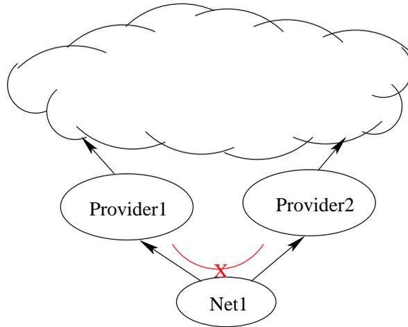
Figure 2-7: Packets are generally forbidden to traverse the path  $\text{Provider1} \rightarrow \text{Net1} \rightarrow \text{Provider2}$ . An arrowed line in the figure represents a customer-provider connection, with the arrow ending at the provider.
