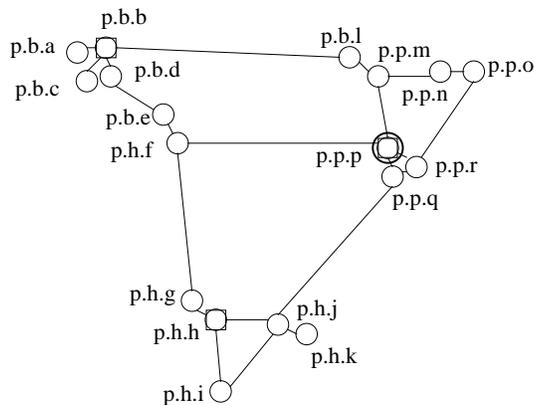
Figure 2-4: An example of a landmark-hierarchy network. A node marked by a square is a level 1 landmark. A node marked by a bigger circle is a level 2 landmark.  $r_0 = 0$ ,  $r_1 = 2$ ,  $r_2 = 4$ .
