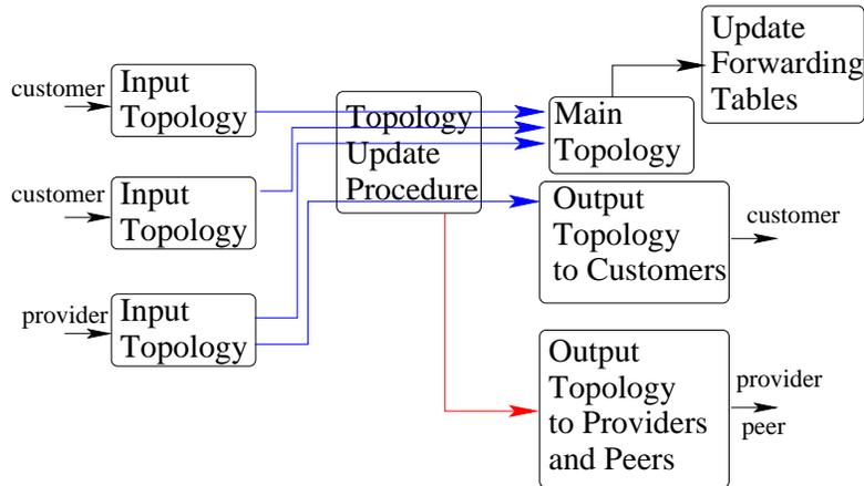
Figure 4-15: When a router receives a **topology** message from a neighbor, it first updates the input topology database for the neighbor. If the input topology database is connected to the output topology database of a neighbor class, the router will invoke the topology update procedure and send changes to the corresponding neighbors. The router may also update its forwarding tables.
