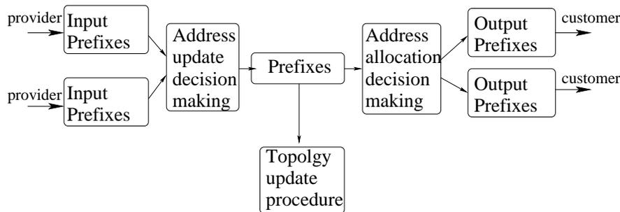
Figure 4-12: When a router receives a non-empty **address** message from a neighbor, it first updates its input prefix database. If its policy allows, it will update its main prefix database, allocate, withdraw, or renew subdivisions of its prefixes, update its output prefix databases to its customers, and send out messages to notify the customers of the update. The router will also invoke the topology update procedure to update its topology databases and its forwarding tables.
