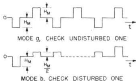
Fig. 4—Core-testing pulse patterns of H.
