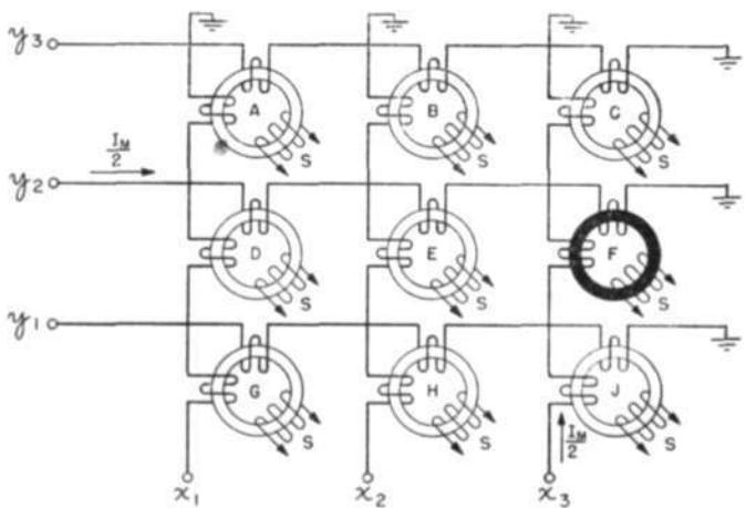
Fig. 2—A two-dimensional array of cores.
