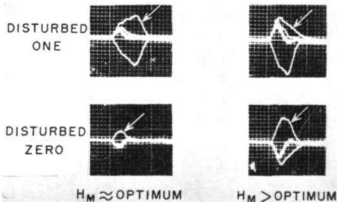
Fig. 6—Coincident-current test results, best ferritic core.
