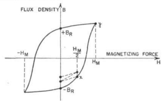
Fig. 1—Paths of operation of a magnetic memory unit.
