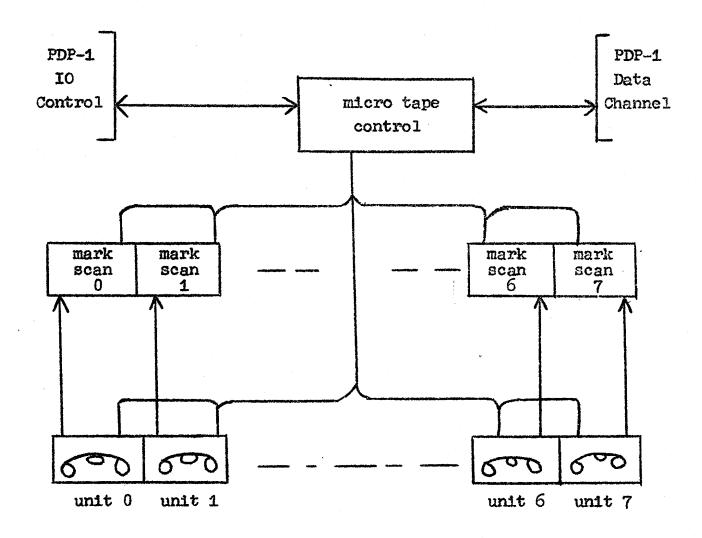
Figure 1. Microtape system configuration.
