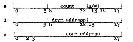
Mta 104 and mta 105 are used to read any absolute drum address. The format is the same as for a drum 1vk, except that the drum field comes from I(0-5). Mta 104 reads fields 0-77, mta 105 reads fields 100-177. Mta 104 and mta 105 skip if no drum error occurs.
