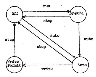
When a drive is off, the motors are not operating, and a tape may be mounted or removed. When in manual mode, the motors are under control of the "fwd" and "rev" buttons. When in automatic or write permit modes, the motors are under control of the computer and the tape may be read or written under program control.
