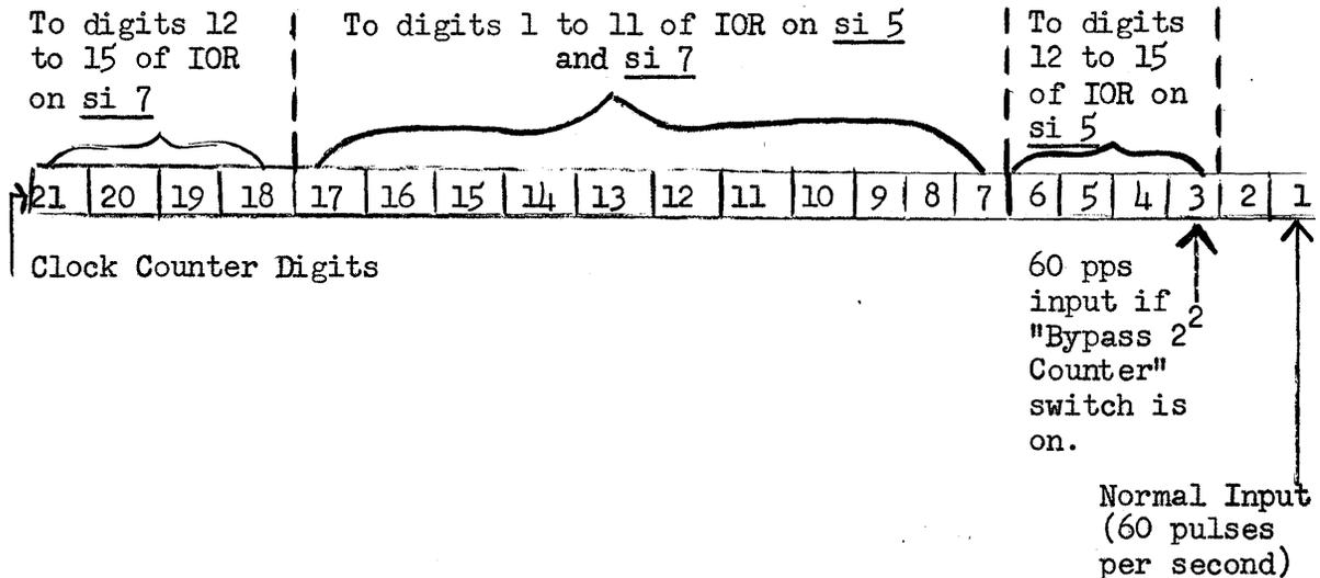
Figure 4: Clock (Timing Register)
