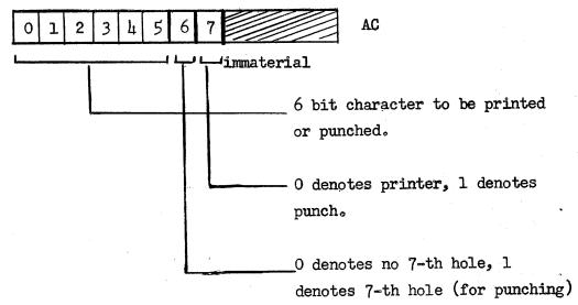
An rc instruction must be given for each character to be printed or punched. Any number of rc instructions may follow the si. Each rc instruction requires 7.6 ms during which time no in-out instruction can be performed.
