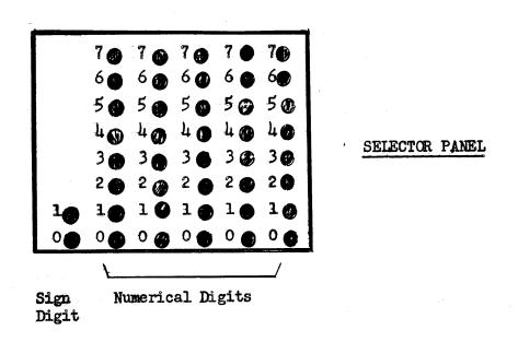
For example, if the number 0.00001 is placed in the selector panel, then selection of the manual mode by the operator will cause the CS translation program to produce binary (fb) tapes whenever CS flexo (fc) tapes are translated.
