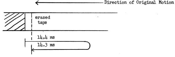
Use of this si instruction guarantees that a tape unit will stop in erased area. If a tape unit is stopped by selecting another piece of equipment it is switched immediately to the read mode and in coasting to a stop may pass over previously recorded information. This technique for stopping a unit may be used, however, if it is known in advance that the tape has been erased.
