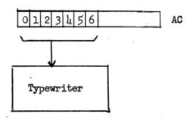
It takes 125 ms to print each character (not a tab or carriage return). It takes up to 900 ms to print a tab or carriage return. A table of the Flexowriter characters printed by the typewriter is given in Chapter V.
