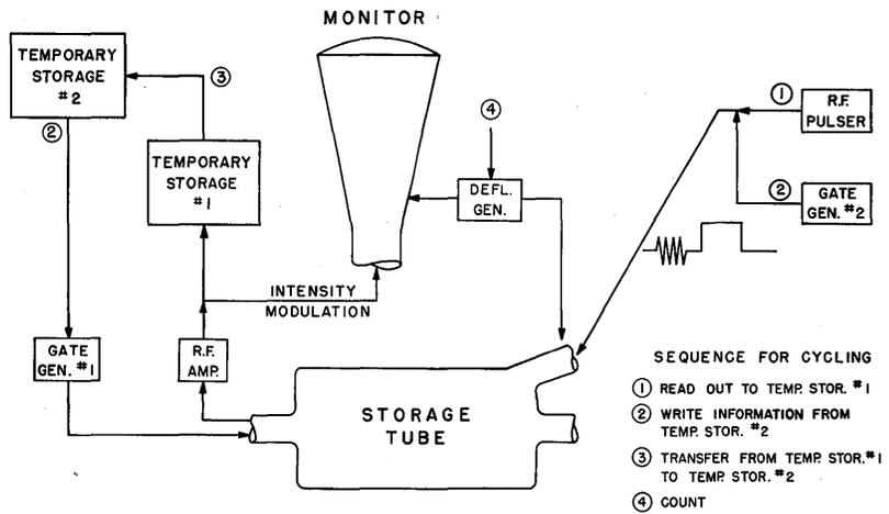
Fig. 13. Block diagram of dynamic tester
