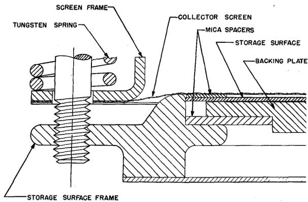
Fig. 5. Storage assembly section
