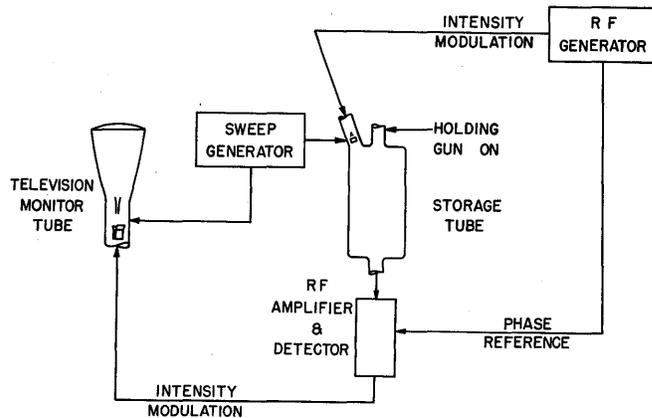
Fig. 10. Television test method
