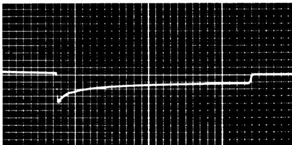
Fig. 3. Plate current waveform deteriorated tube
