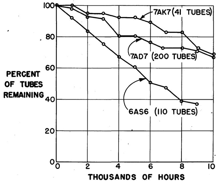
Fig. 6. Tube life experience in computer circuits
