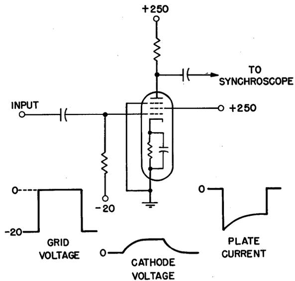
Fig. 4. Effective equivalent of deteriorated tube
