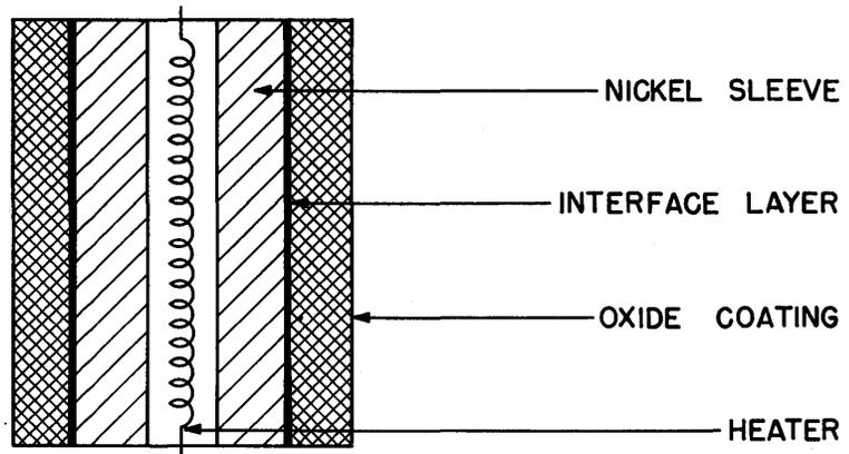
Fig. 5. Section through cathode with interface
