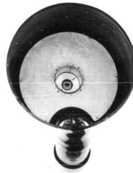
Fig. 2-1. Storage tube ion collector plate.
