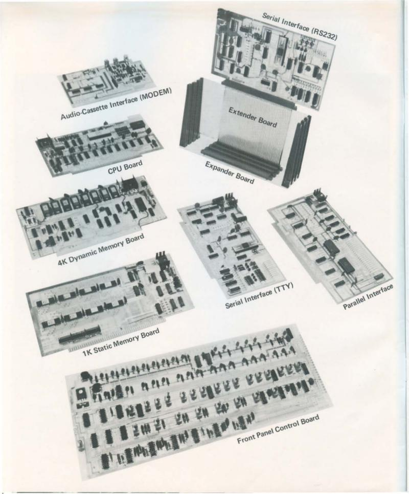
Memory board options include 1024 byte static cards, 4096 byte dynamic cards and an Audio-Cassette Record Interface that allows you to connect your Altair to any tape recorder for inexpensive, unlimited storage. EACH MEMORY CARD HAS MEMORY PROTECT FEATURES.
