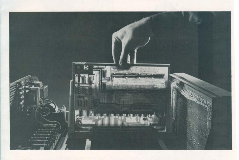
The Altair 8800 has been designed with buss orientation to be easily expanded and easily adapted to thousands of applications. Any card can be plugged into any slot and the correct address, etc., for that card will be picked up off the buss system.
