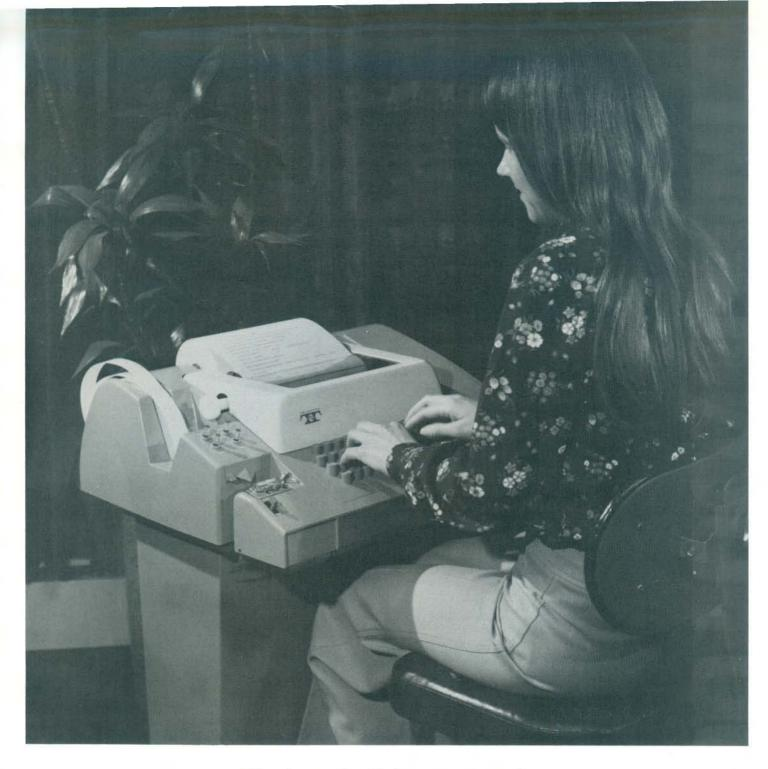
This teletype prints 10 characters per second. It has a built-in paper tape reader and punch. It is a completely checked-out machine with a standard 120 day teletype warranty. Includes teletype interface card.
