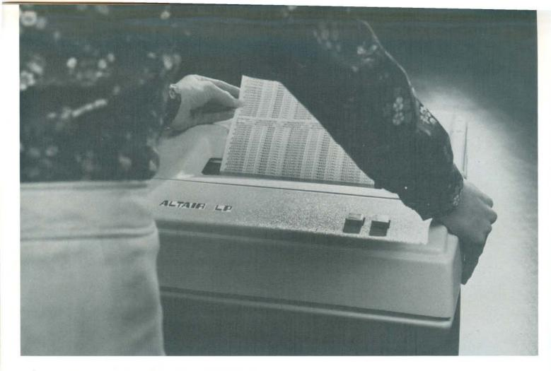
The Altair 110 Line Printer is a desktop line printer that produces 80 columns of 5 x 7 dot matrix characters at 100 characters per second x 70 lines per minute. The impact head prints bidirectionally on a 8½" roll paper\* using a conventional teletype ribbon. The Altair Line Printer will print up to four copies of any item.
