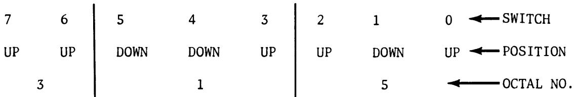
Note that switches 8 through 15 were not used. Switches 0 through 7 correspond to the switches labeled DATA on the front panel. A memory address would use all 16 switches.
