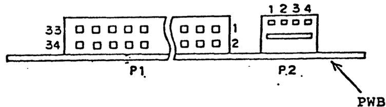
Figure 3-1 Connector P1 and P2 Pin Numbers
