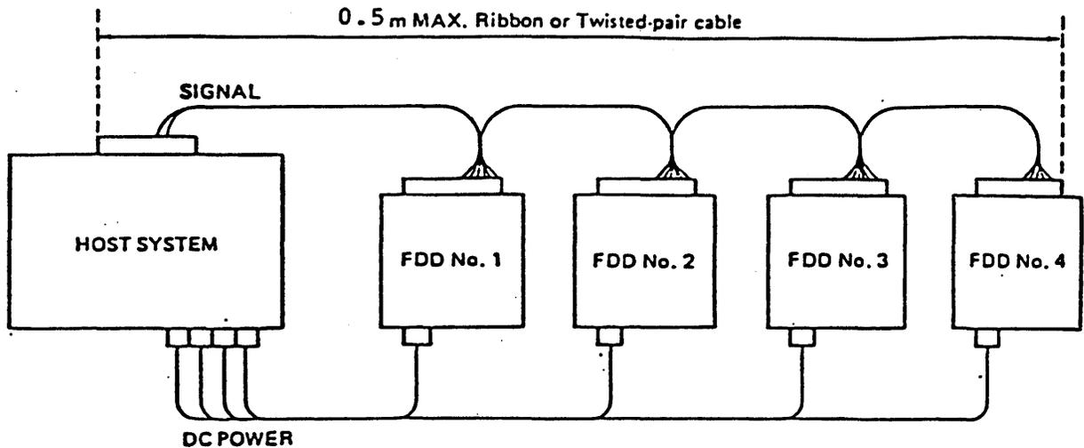
Figure 3-2 Cable connection (Schematic diagram)
