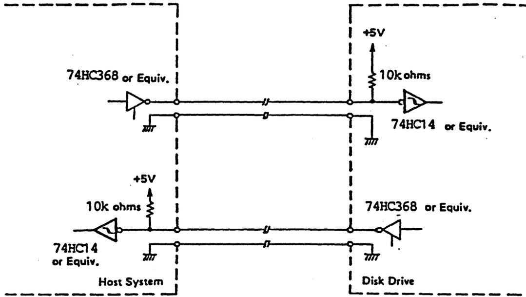
Figure 3-3 Recommended Line Drive and Receiver Circuit
