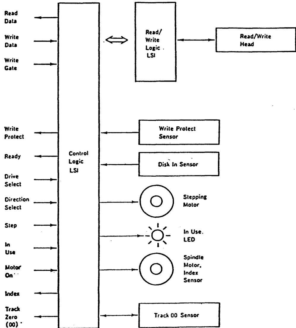
Figure 2-1 MF355B Functional Diagram
