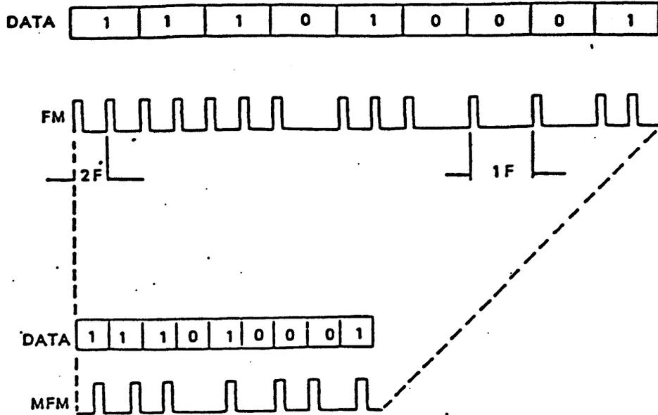
Figure 4-1 Comparison of FM and MFM encoding
