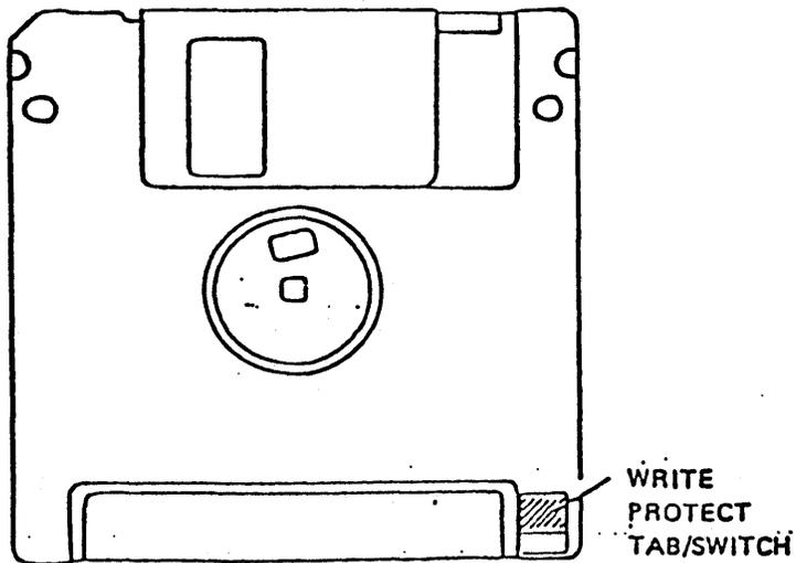
Figure 3-12 Write Protect on Disk
