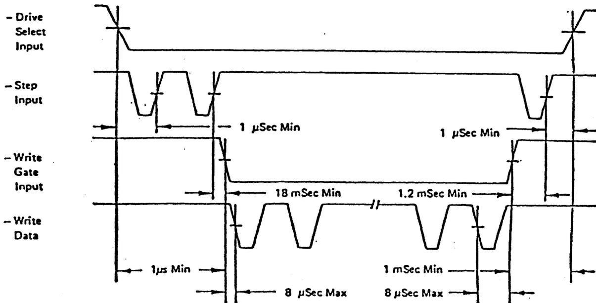
Figure 3-6 Write Gate Timing
