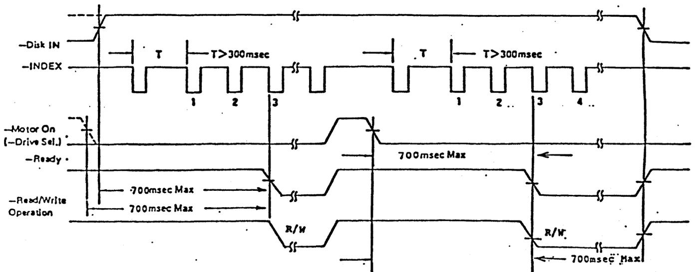
Figure 4-2 The Timing of STANDARD READY signal
