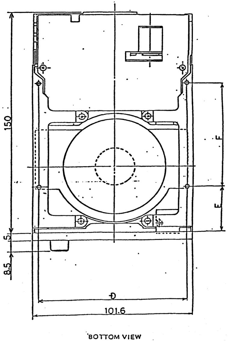
Figure 6-2 Dimensions of MF355B ( mm )
