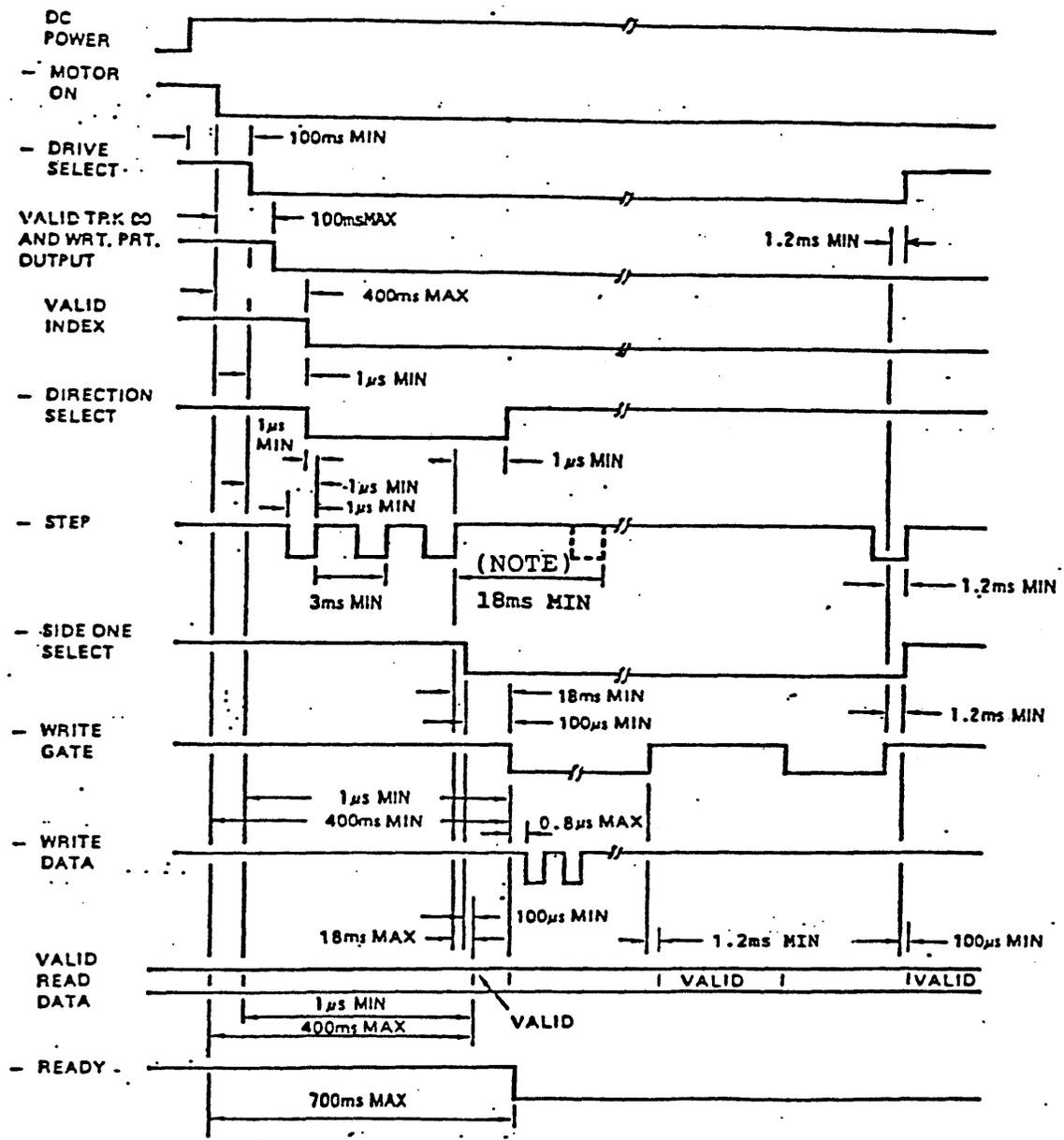
NOTE:When reversing direction, issue a next step pulse after more than 18 ms from the step pulse before inversion.
