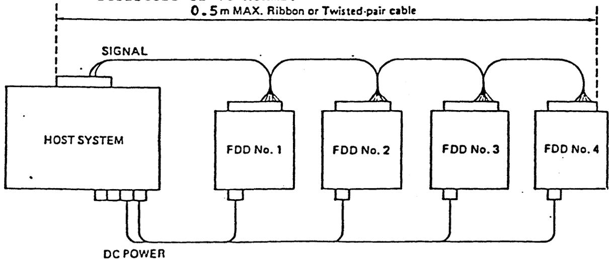
Figure 3-2 Cable connection (Schematic diagram)
