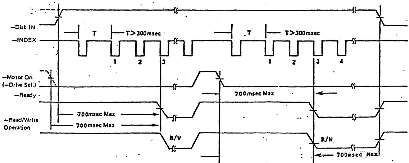
Figure 4-2 The Timing of STANDARD READY signal
