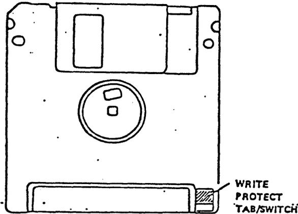
Figure 3-12 Write Protect on Disk
