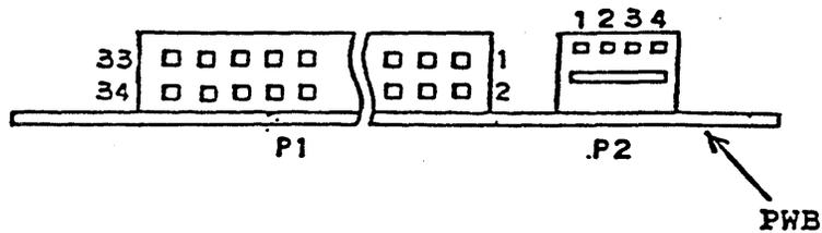
Figure 3-1 Connector P1 and P2 Pin Numbers
