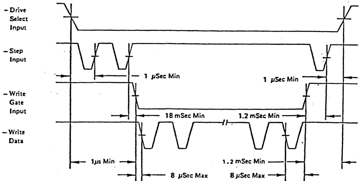
Figure 3-6 Write Gate Timing
