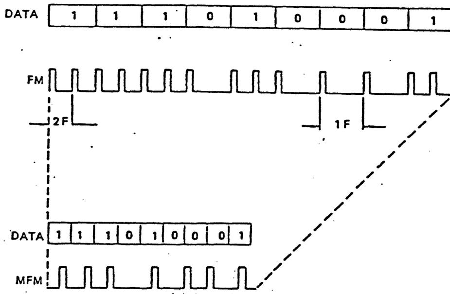
Figure 4-1 Comparison of FM and MFM encoding
