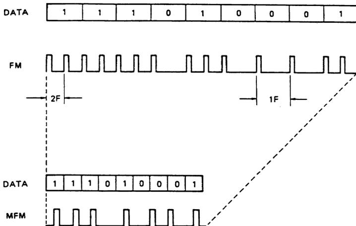
Fig. 4-3 Comparison of FM and MFM Encoding Systems
