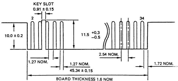
Fig. 5-1 Connector J1 Dimensions (mm) and Pin Numbers
