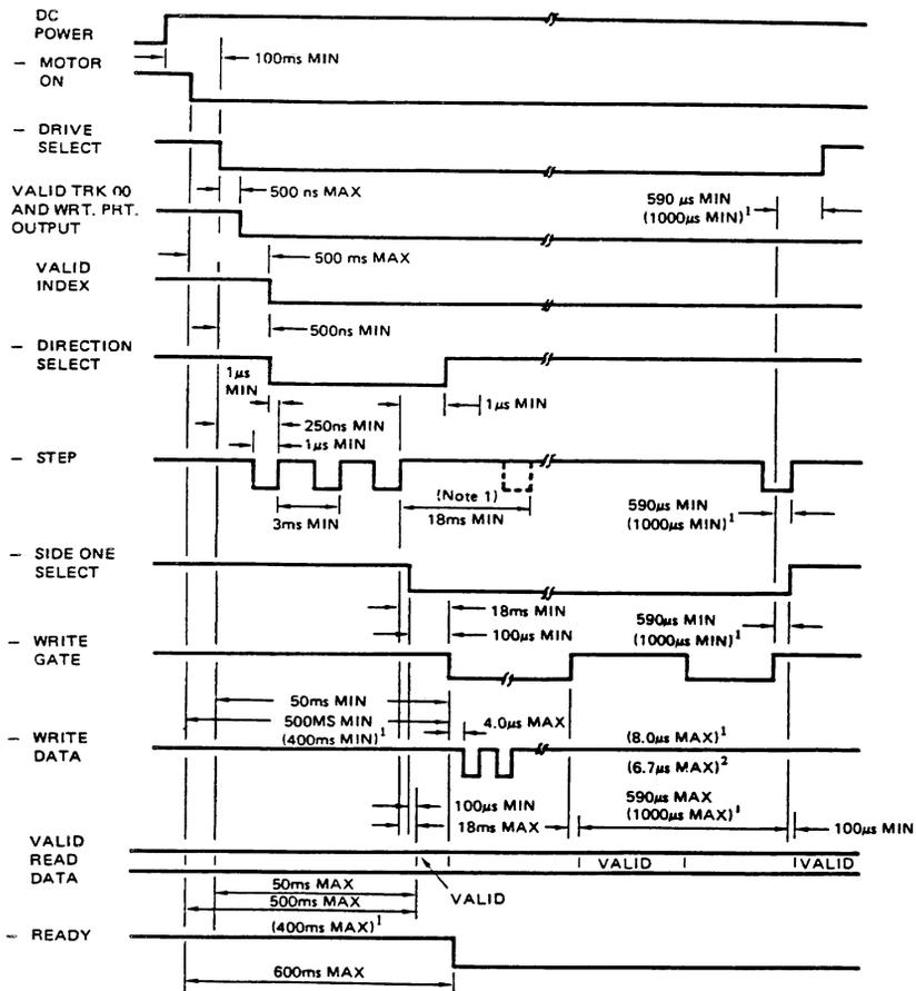
Note 1: When reversing direction, issue a next step pulse after more than 18 ms from the step pulse before inversion.
