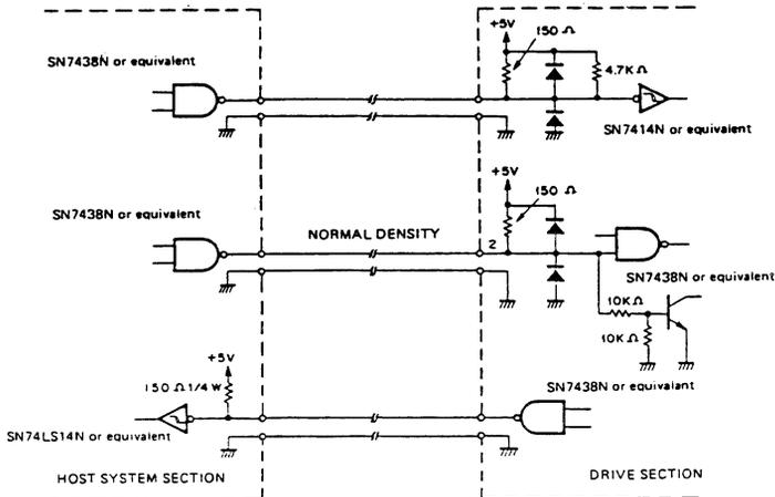
Fig. 3-2 Recommended Line Driver and Line Receiver Circuits
