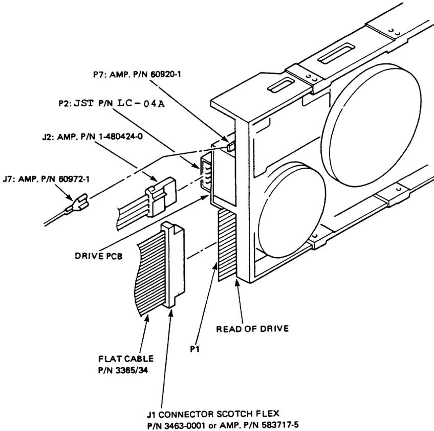
Fig. 5-3 Location of Interface Connectors
