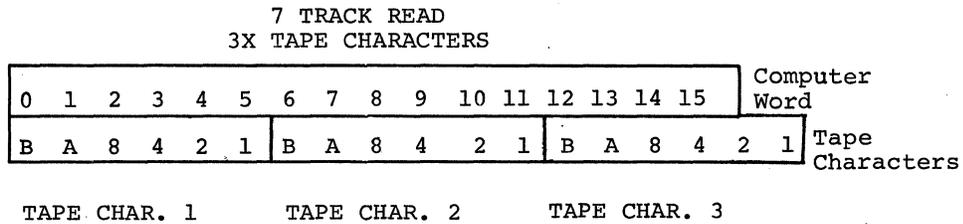
When reading from 7 track drives, transfer is implemented by positioning the first tape character encountered as the 6 upper order bits, the second tape character as the next 6 bits, and the third tape character as the 4 low order bits of the computer word. Tracks 1 and 2 of every third tape character are ignored and thereby lost.
