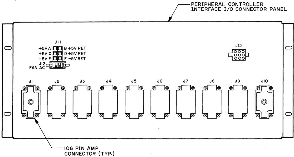
FIGURE 2-6 PCI I/O CONNECTOR PANEL
