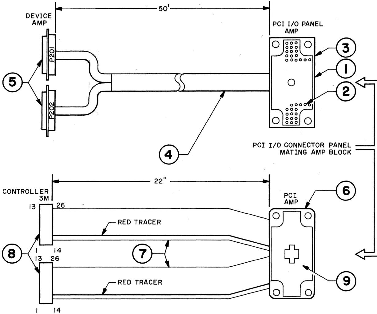
FIGURE 7-2 Line Printer Device Cabling to PCI
