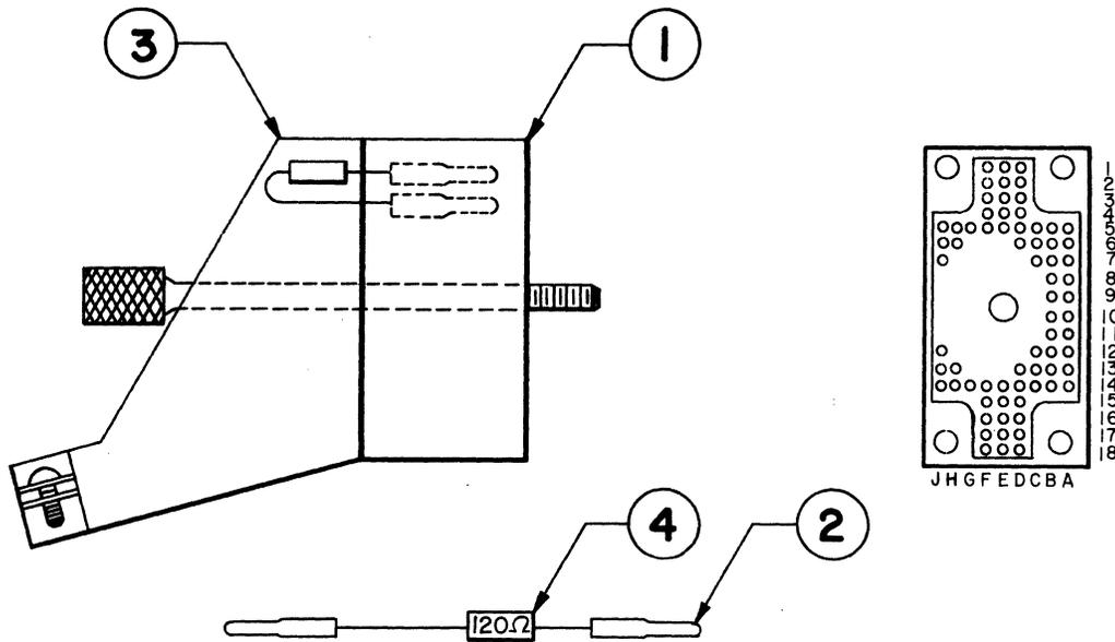
FIGURE 2-13 I/O TERMINATOR
