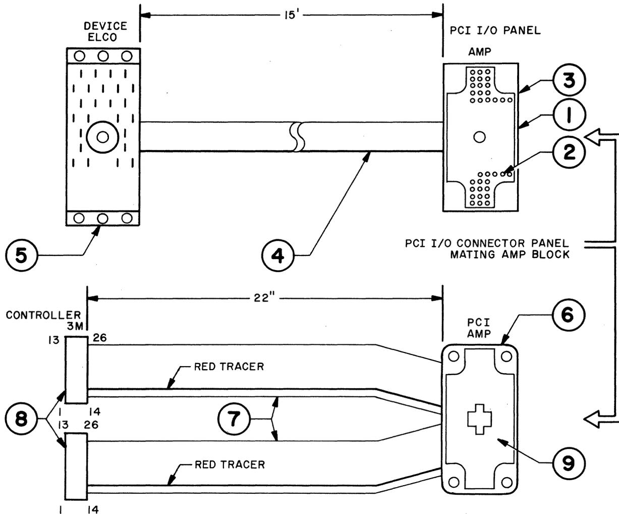
FIGURE 6-2 CARD READER I/O CABLING
