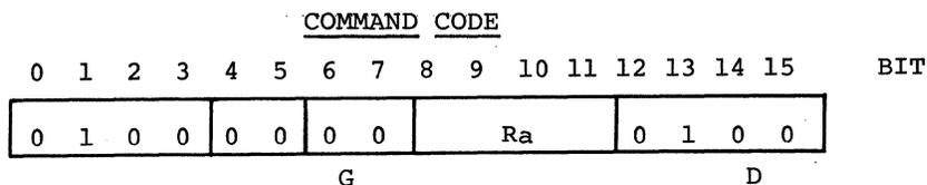
Bit one of the transfer initiate write and read commands defines the I/O transfer mode. See figure 1. Bit one = 0 specifies programmed I/O mode. Bit one = 1 specifies memory file DMP transfer mode.
