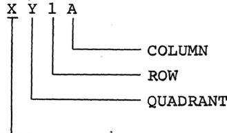
Normally, the plane number (1-4) would be here, but since the controller may be located in any plane (1-4) the 'X' represents the plane number. Refer to Figure 2-3 for an example.
