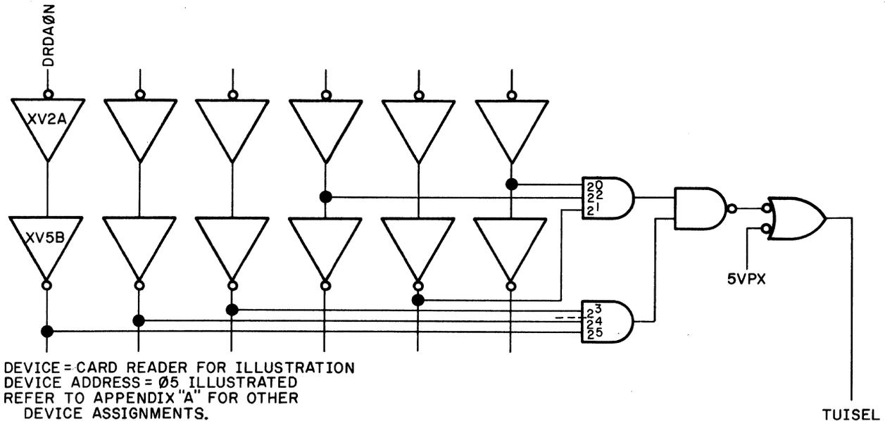
FIGURE 5-2 DEVICE ADDRESS
