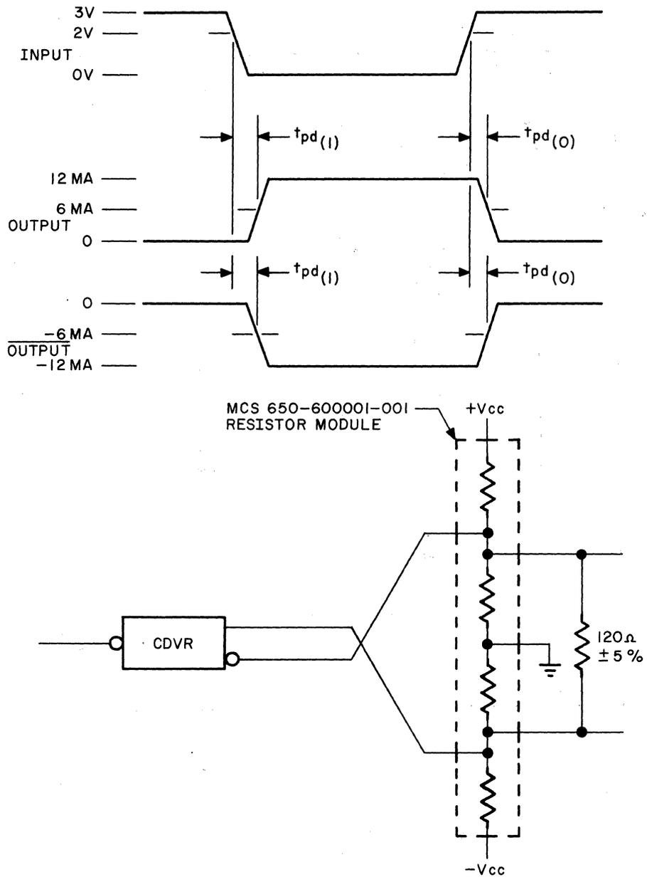
FIGURE 2-11 WAVE FORMS AND TERMINATION NETWORK
