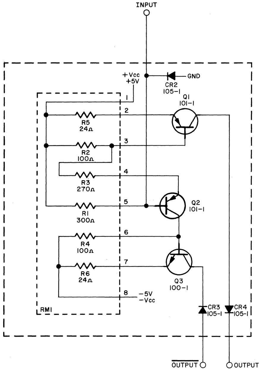
FIGURE 2-10 CABLE DRIVER SCHEMATIC
