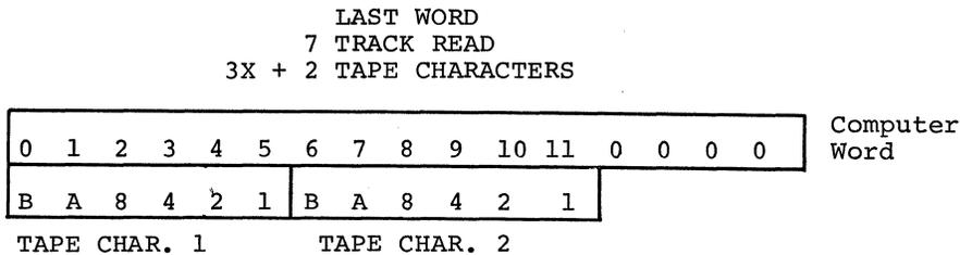
If a multiple of three plus 1 tape characters are read, the last tape character is positioned as the upper order 6 bits and bits 6 thru 15 of the last word are set to zero as shown below.
