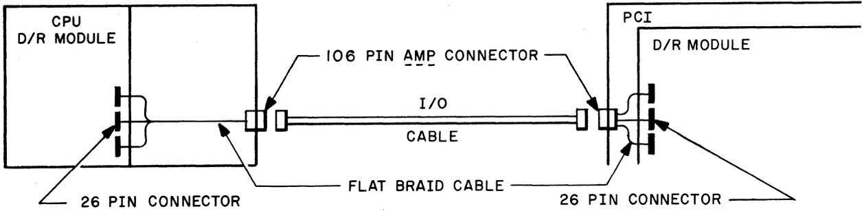
FIGURE 2-5 I/O BUS INTERCONNECTION DIAGRAM
