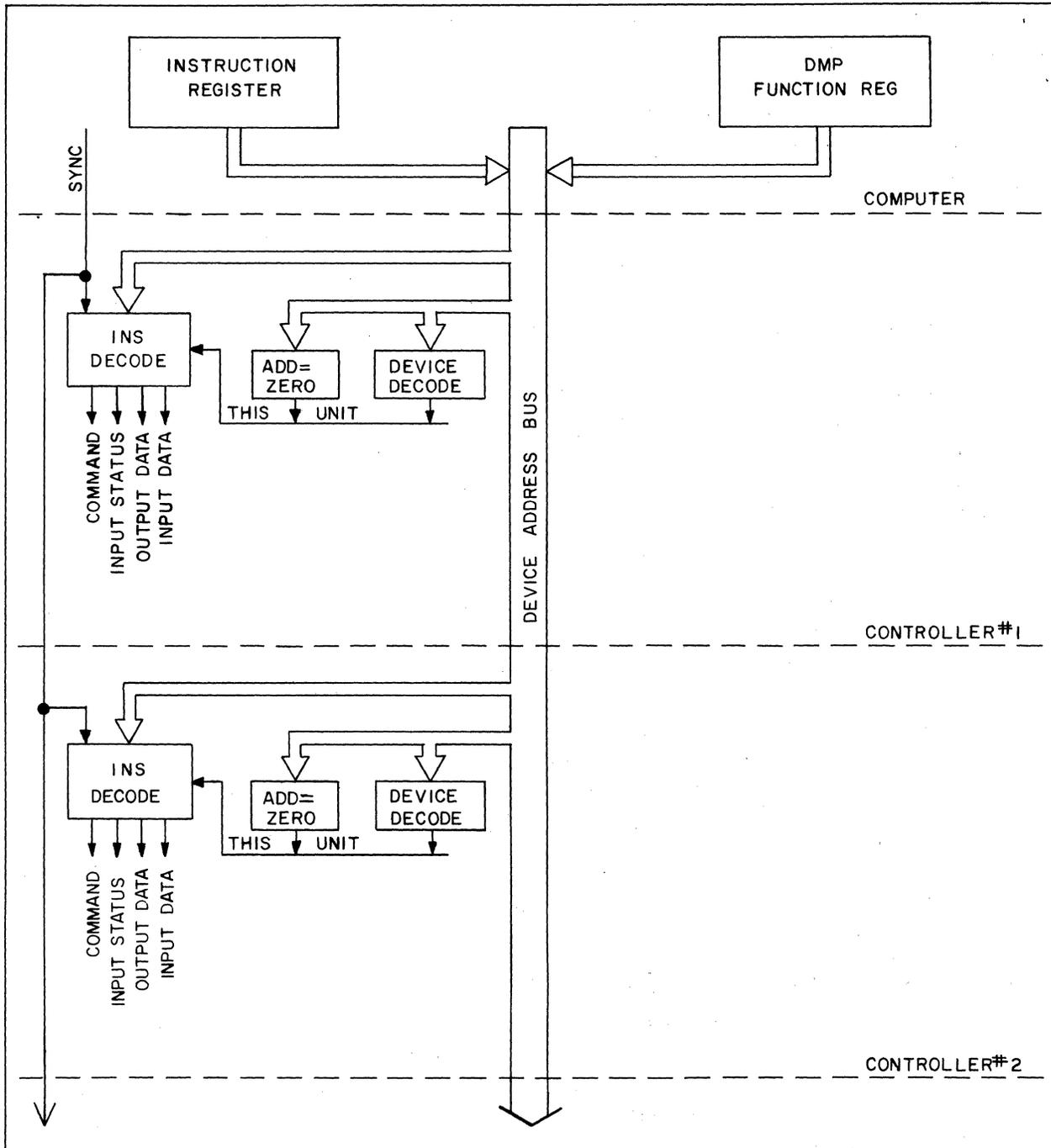
FIGURE 3-2 DEVICE ADDRESS AND INSTRUCTION DECODE
