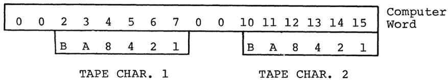
When reading from 7 track drives, transfer is implemented by positioning the first tape character encountered as bits 2-7 and the second tape character as bits 10-15 of the computer word. Bits 0,1,8 and 9 are set to zero in each word.
