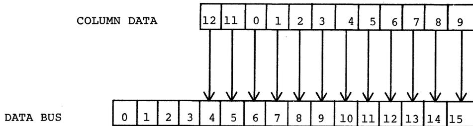
In the translate mode, the correct gates are selected by signal TRANS. In this mode of operation, data is changed from a 12 bit code to a modified 8 bit code.
