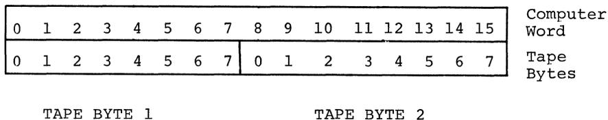
When reading from 9 track drives, transfer is implemented by storing the first tape byte encountered as the most significant byte in a memory word and the second as the least significant byte.
