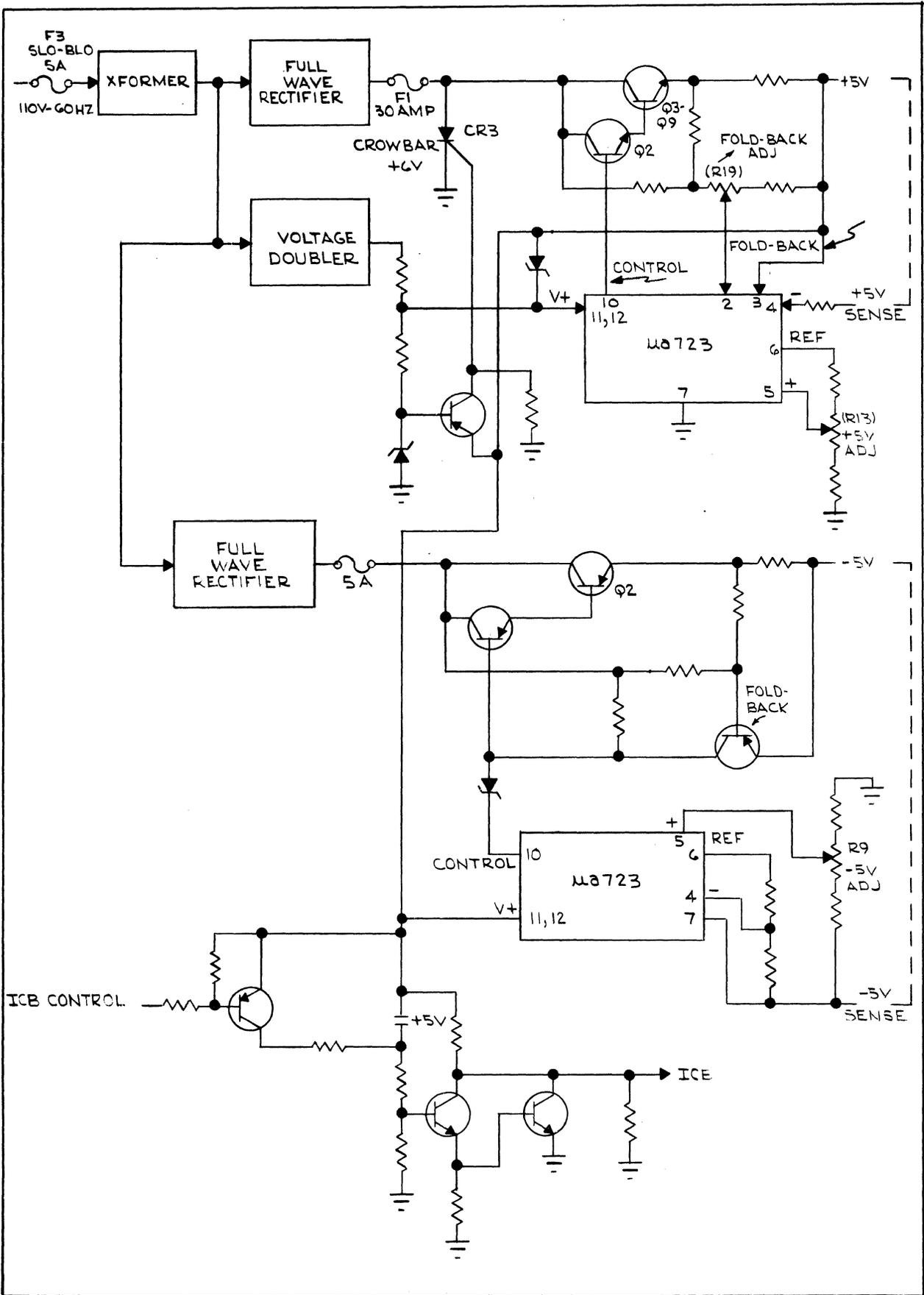
FIGURE 2-7 +5V POWER SUPPLY FUNCTIONAL DIAGRAM
