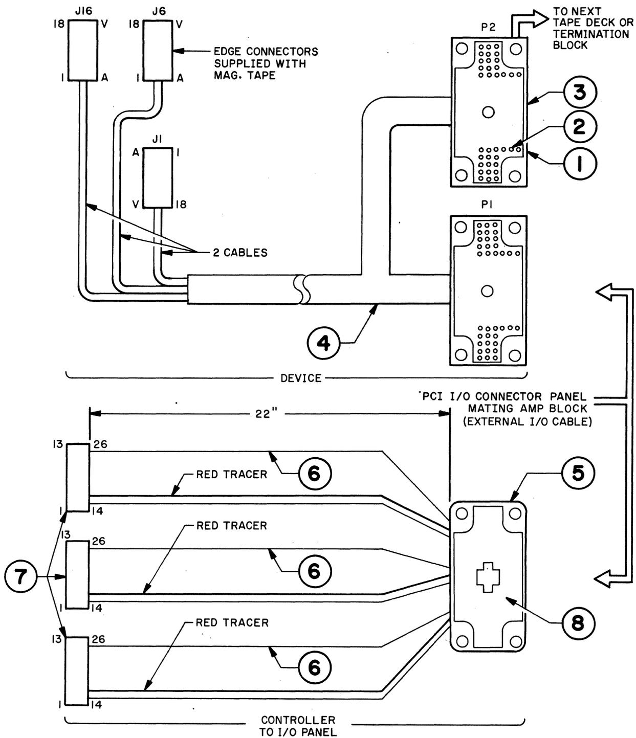
FIGURE 8-1 DEVICE CABLING
