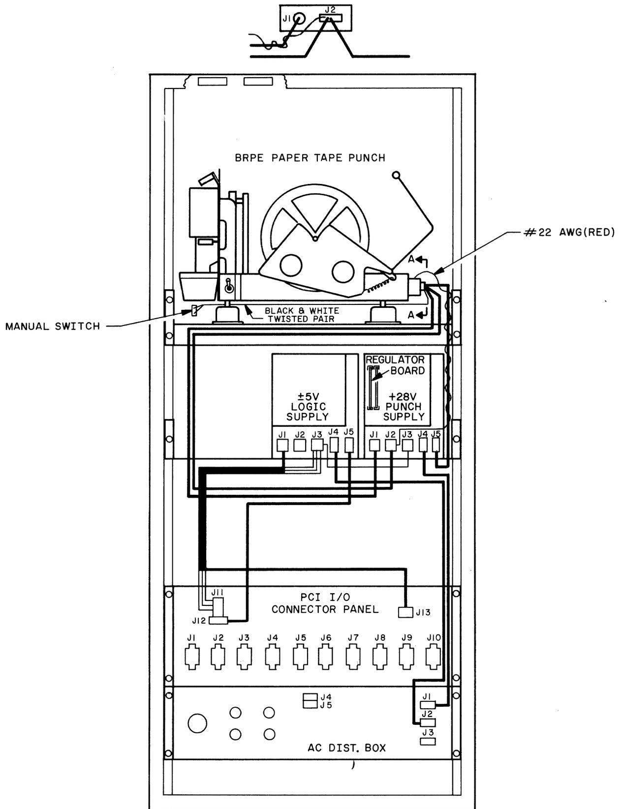
FIGURE 10-1 BRPE RACK CABLING
