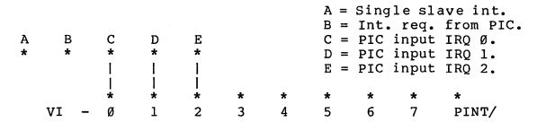
When the cascade cable is installed, [A] may be used to route a single slave's interrupt request [B] to one of the master PIC inputs. In this way, none of the S-100 vectored interrupt lines need be used. This only applies to a master and one slave, additional Mult I/O slaves must send their interrupt requests down any of the vectored interrupt lines of the buss.
